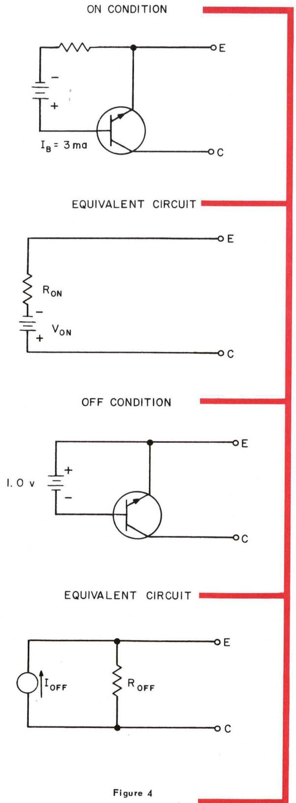
Note that the germanium transistors were operated in the inverted position.
