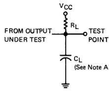
**LOAD CIRCUIT FOR OPEN-COLLECTOR OUTPUTS**
