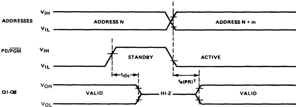
$t_{a(PR)}^\dagger$  referenced to PD/PGM or the address, whichever occurs last.
