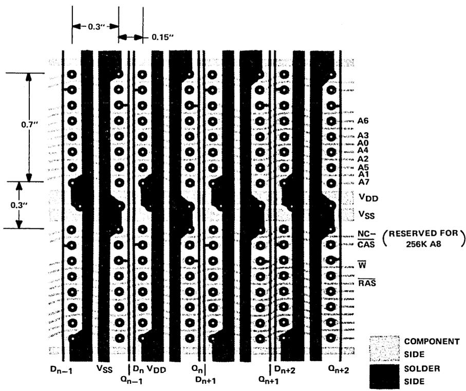
FIGURE 2 – PC BOARD LAYOUT FOR TMS 4164 (SHOWN 2X)
