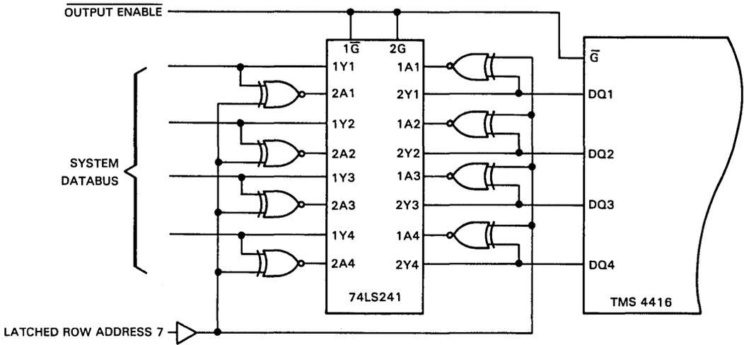
FIGURE 2 - CIRCUIT FOR COMPENSATION OF INTERNAL DATA INVERSION
