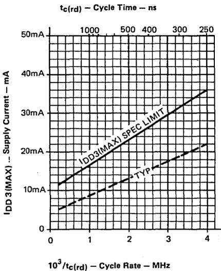
PAGE-MODE CYCLE RATE (& TIME) vs MAX SUPPLY CURRENT, I<sub>DD4</sub>
