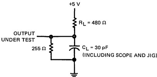
FIGURE 1 – LOAD CIRCUIT
