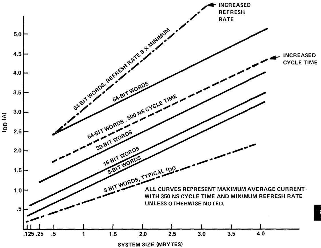
FIGURE 2 – 100%-ACTIVE  $I_{DD}$  vs SYSTEM SIZE
