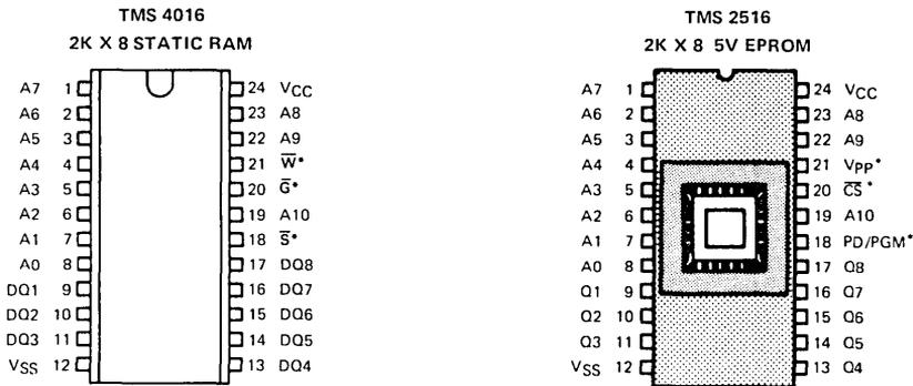
\*These pins though apparently different are compatible when switching to the TMS 2516.
