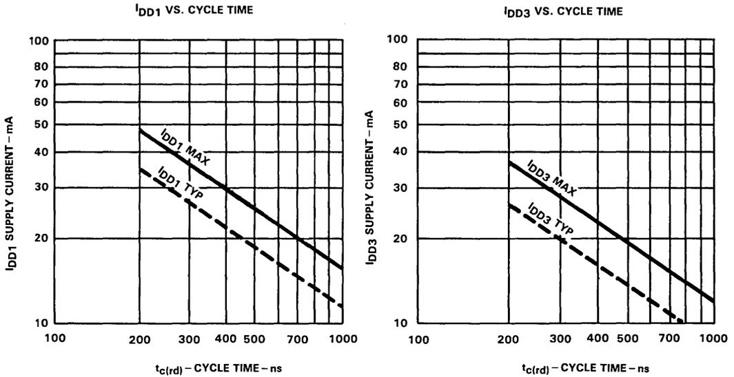
FIGURE 1 – I<sub>DD</sub> vs CYCLE TIME
