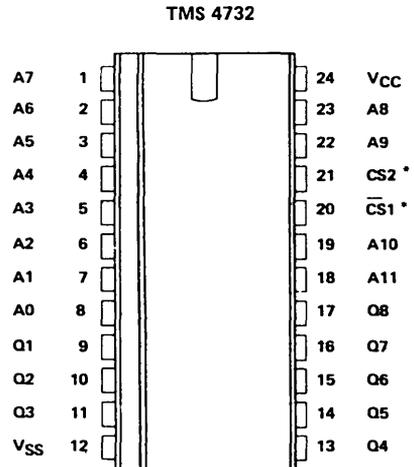
\*These pins though functionally different are compatible when upgrading to the TMS 4732. ( $\overline{CS1}$  must be active low and CS2 active high).
