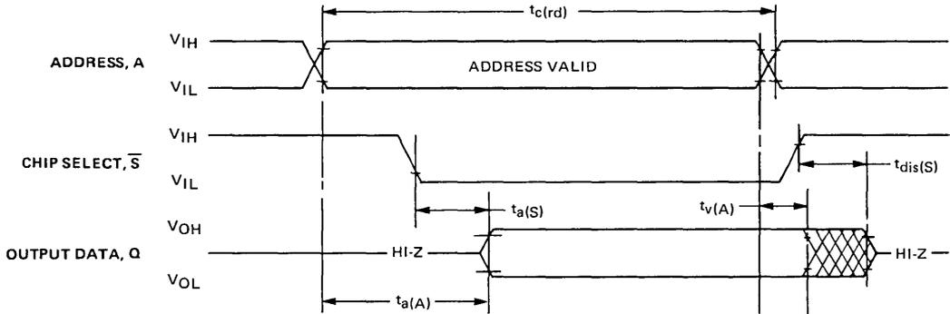
All timing reference points are 0.8 V and 2.0 V on inputs and 0.6 V and 2.2 V on outputs (90% points). Input rise and fall times = 10 ns.
