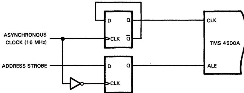
FIGURE 2b – TMS 4500A FAST CLOCK FAST SYNCHRONIZATION INTERFACE
