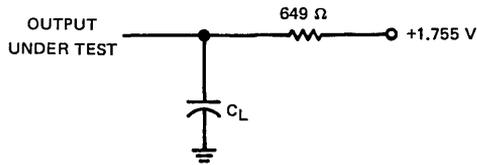
FIGURE 1 – OUTPUT LOAD
