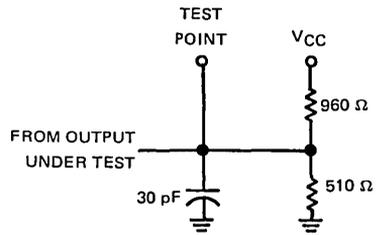
FIGURE 1B – MATCH OUTPUT LOAD CIRCUIT
