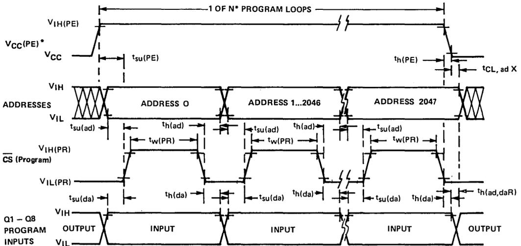
\* $V_{CC(PE)}$  is at 0 V or +12 V through N program loops where  $N \geq 100 \text{ ms}/t_w(PR)$ .
