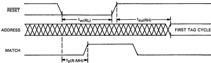
NOTE: Input pulse levels are 0 V and 3 V, with rise and fall times of 5 ns. The timing reference levels on the input pulses are 0.8 V and 2.0 V. The timing reference level for output pulses is 1.5 V. See Figures 1A and 1B for output loading.
