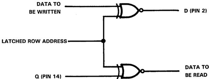
FIGURE 2 - CIRCUIT FOR COMPENSATION OF INTERNAL DATA INVERSION
