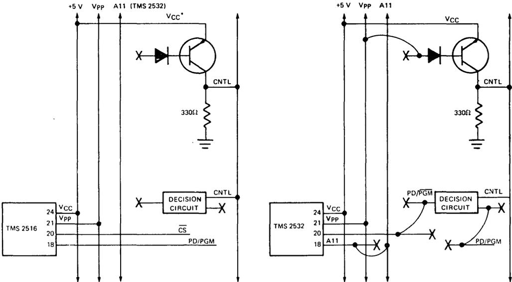
\*In the original circuitry before upgrade one of the power supplies, either  $V_{CC}$  or  $V_{PP}$ , should not be connected to the transistor. (In above example we show  $V_{CC}$  connected.) In the upgraded TMS 2532 circuit, both supplies are connected to the transistor.
