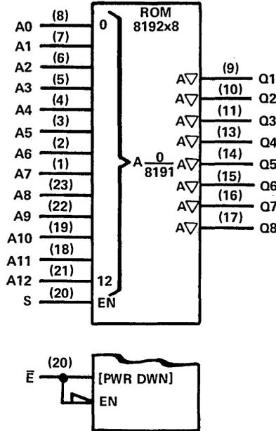
Pin 20 can be active-high as shown in the upper symbol or active-low as shown in the lower (partial) symbol. It can be either a chip select (S or  $\bar{S}$ ) or a chip enable/power down ( $\bar{E}$ ).
