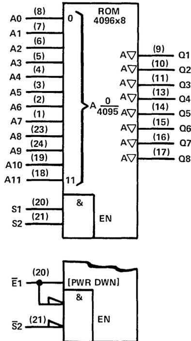
Pins 20 and 21 can be active-high as shown in the upper symbol or active-low as shown in the lower (partial) symbol. Pin 20 can be either a chip select (S or  $\bar{S}$ ) or a chip enable/power down ( $\bar{E}$ ).
