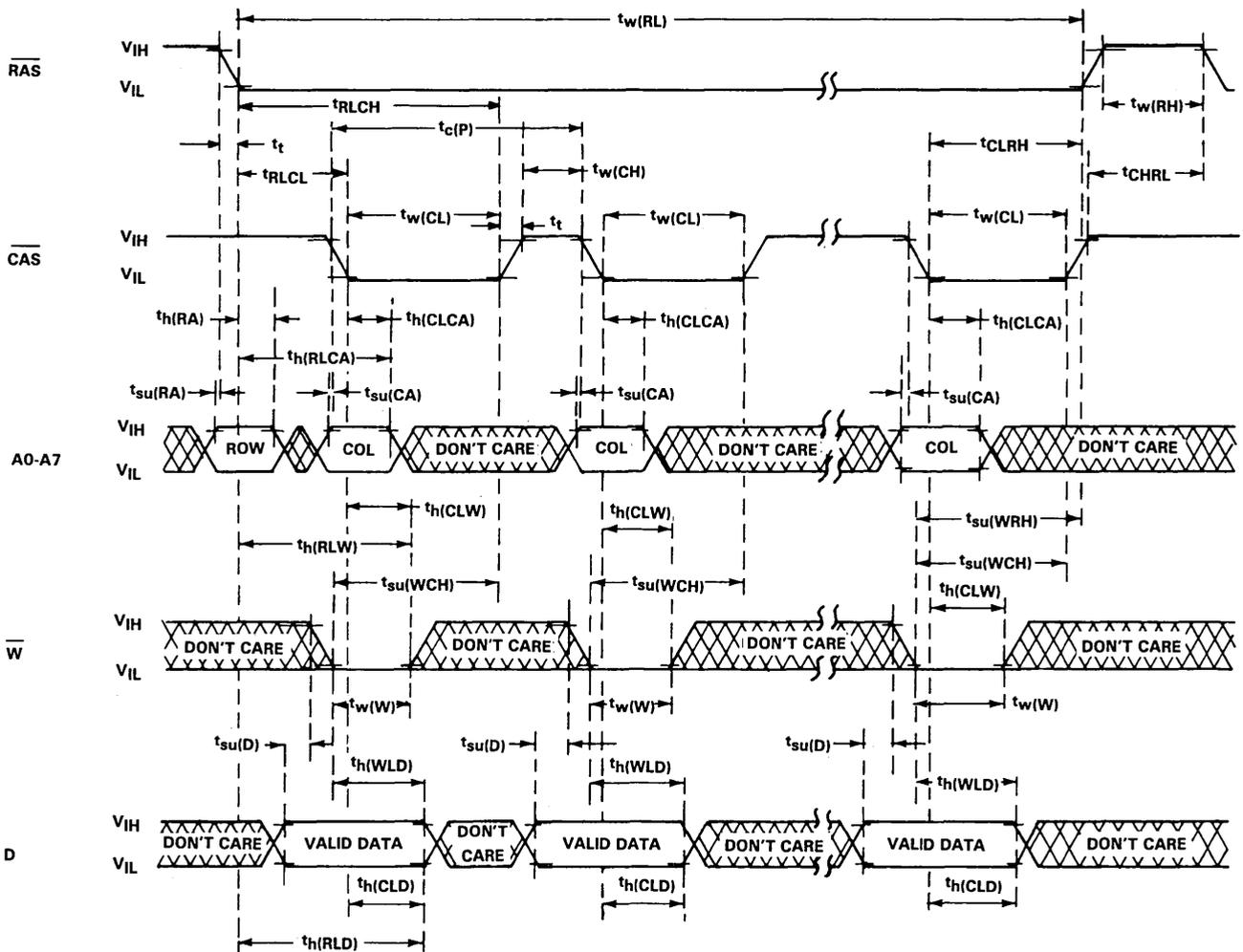
NOTE: A read cycle or a read-modify-write cycle can be intermixed with write cycles as long as read and read-modify-write timing specifications are not violated.
