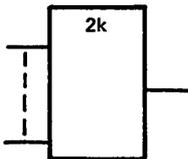
Even-parity element. The output stands at its 1-state if an even number of inputs stand at their 1-states.
