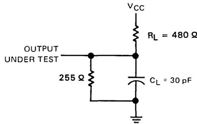
FIGURE 1 – LOAD CIRCUIT
