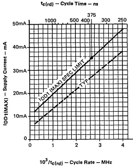
CYCLE RATE (& TIME) vs MAX SUPPLY CURRENT, I<sub>DD3</sub>
