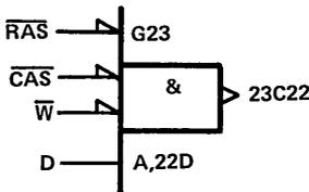
By virtue of the AND relationship between  $\overline{CAS}$  and  $\overline{W}$  (explicitly shown), when either one of these inputs goes low with the other one and  $\overline{RAS}$  already low ( $\overline{RAS}$  is AND'ed by G23), the D input is momentarily enabled (through C22). In an "early-write" cycle it is  $\overline{W}$  that goes low first; this causes the output to remain off as explained below.
