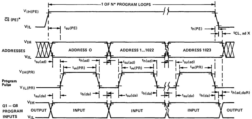
\*CS(PE) is at +12 V through N program loops where  $N \geq 100 \text{ ms}/t_w(PR)$ .
