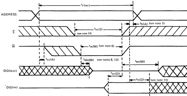
All timing reference points are 0.8 V and 2.0 V on inputs and 0.6 V and 2.2 V on outputs (90% points). Input rise and fall times equal 10 nanoseconds.
