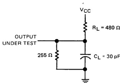
FIGURE 1 – LOAD CIRCUIT
