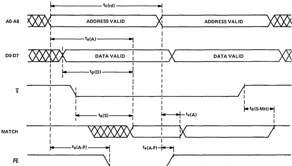
NOTE: Input pulse levels are 0 V and 3 V, with rise and fall times of 5 ns. The timing reference levels on the input pulses are 0.8 V and 2.0 V. The timing reference level for output pulses is 1.5 V. See Figures 1A and 1B for output loading.
