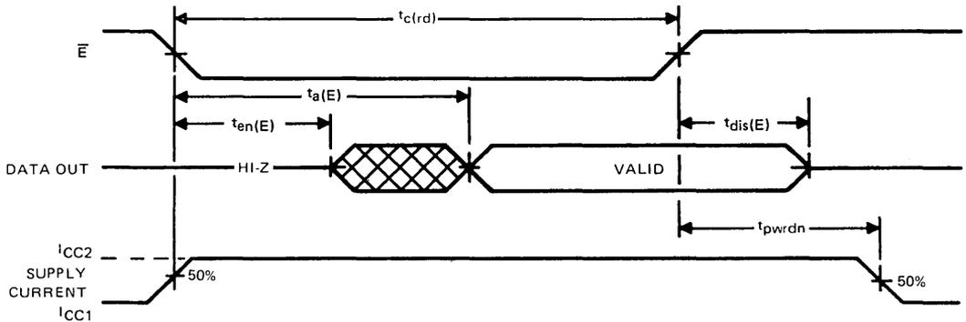
$\bar{W}$  is high, address is valid prior to or simultaneously with the high-to-low transition of  $\bar{E}$ .
