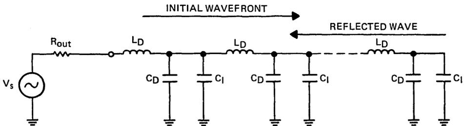
FIGURE 1 - EQUIVALENT CIRCUIT OF MEMORY ARRAY
