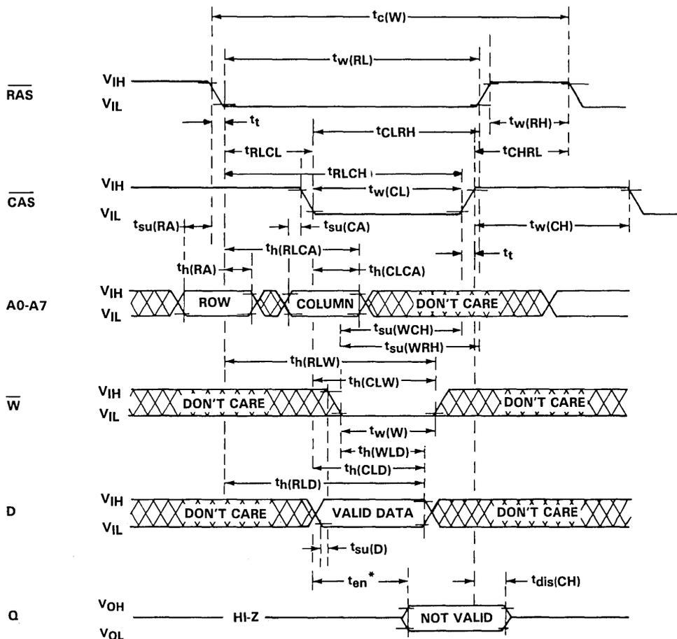
\* The enable time ( $t_{en}$ ) for a write cycle is equal in duration to the access time from  $\overline{CAS}$  ( $t_a(C)$ ) in a read cycle; but the active levels at the output are invalid.
