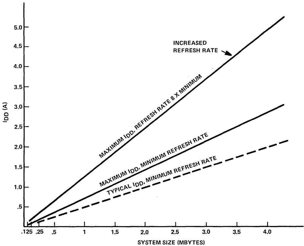
FIGURE 3 – STANDBY  $I_{DD}$  vs SYSTEM SIZE
