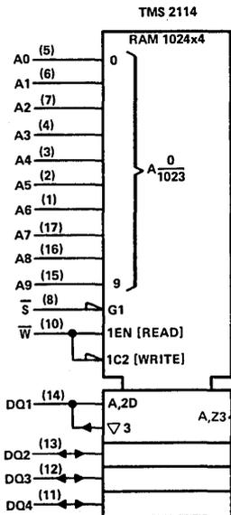
By convention all input lines are located on the left and output lines are located on the right. When an exception is made, an arrowhead shows reverse signal flow. The input/output lines (DQ1 through DQ4) illustrate this.
