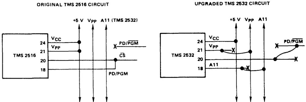
Three modifications need to be made here when upgrading to the TMS 2532: 1) disconnect pin 18 from the  $\overline{CS}$  PC run and jumper it to the A11 bus; 2) disconnect pin 20 from the  $\overline{CS}$  PC run and jumper it to a PD/ $\overline{PGM}$  PC run (or use the existing  $\overline{CS}$  run, and change the function to PD/ $\overline{PGM}$ ); and 3) disconnect  $V_{PP}$  from the  $V_{CC}$  +5 V supply and jumper to the  $V_{PP}$  signal. All other pins are identical.
