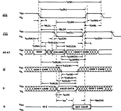
\* The enable time  $t_{en}$  for a write cycle is equal in duration to the access time from  $\overline{\text{CAS}}$  ( $t_{ACC}$ ) in a read cycle, but the active levels at the output are inverted.
