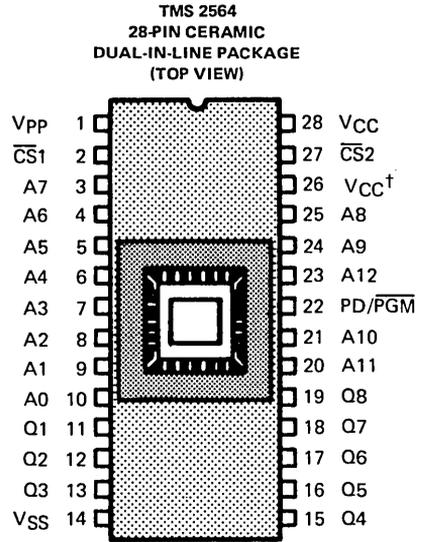
†V<sub>CC</sub> may be connected to pin 26 for 24-pin ROM compatibility.
