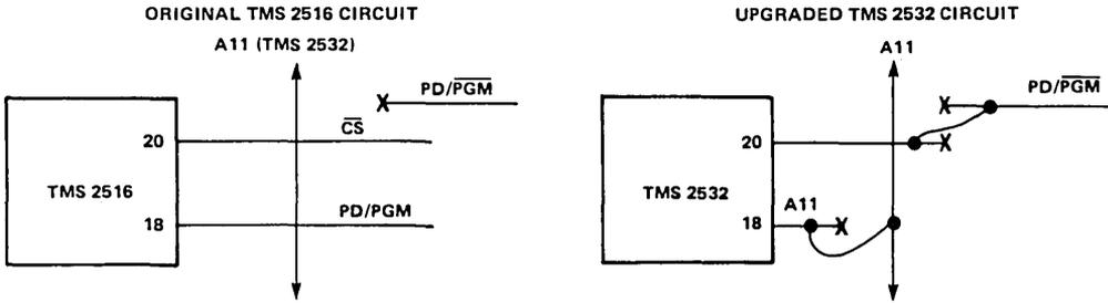
**NOTE:** For both the original and upgrade circuit  $V_{PP}$  (pin 20) and  $V_{CC}$  (pin 21) are not commoned.
