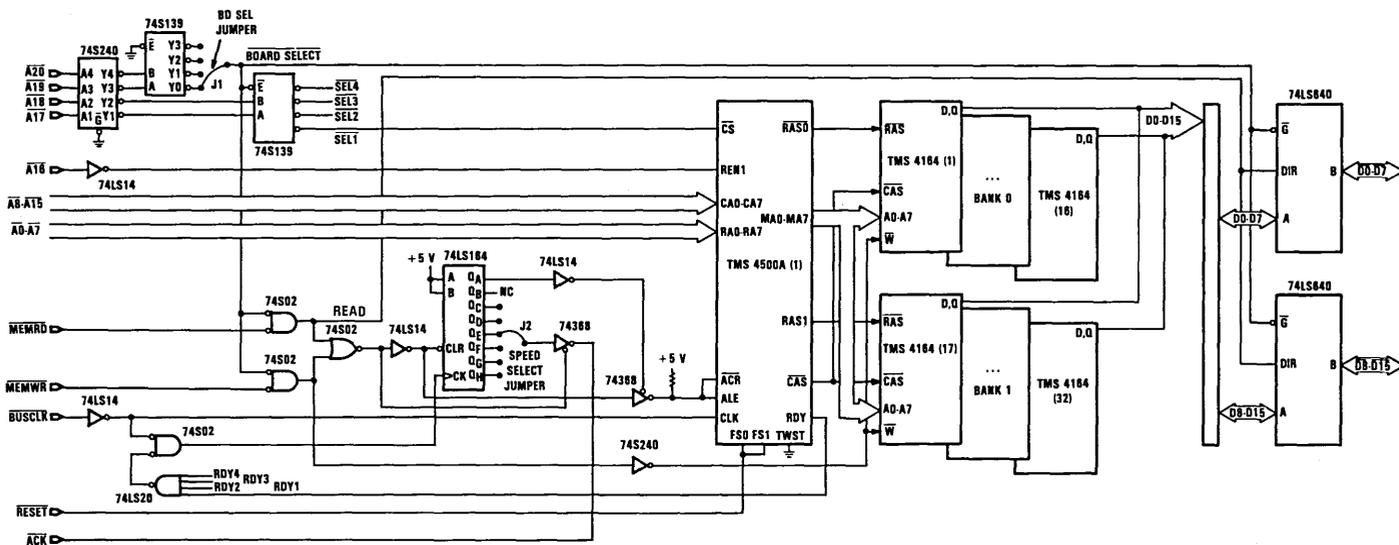
FIGURE 1 - TMS 4500A IN AN ASYNCHRONOUS BUS SYSTEM
