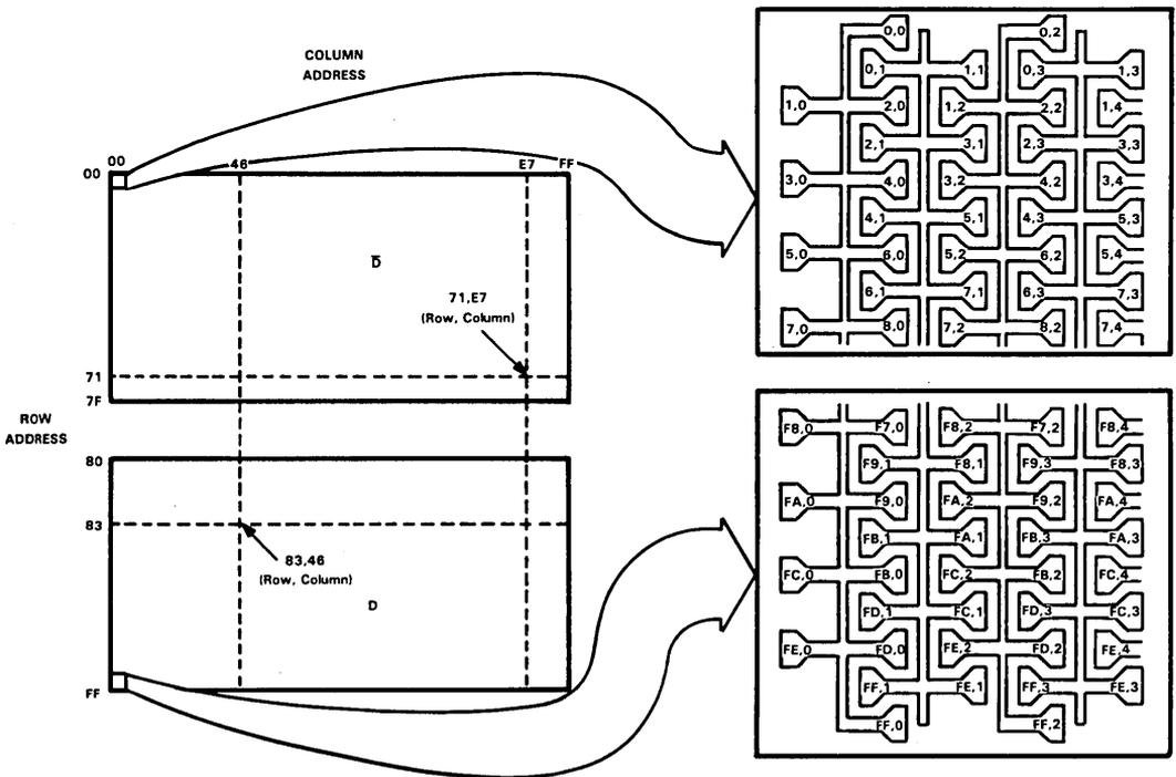
**FIGURE 1C – TMS 4164 ARRAY BIT MAP**
