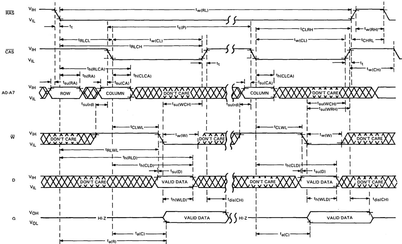
NOTE: A read or a write cycle can be intermixed with read-modify-write cycles as long as the read and write timing specifications are not violated.
