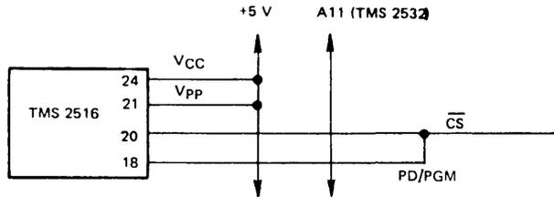
Note that Pin 21, V<sub>PP</sub> can be commoned to the V<sub>CC</sub> +5 V supply since no programming (which requires V<sub>PP</sub> to be +25 V) is planned. Also Pin 18, PD/PGM, can be commoned to the  $\overline{CS}$  PC run. This latter connection causes the device to be powered down whenever it is deselected. (More specifically, for any device not being read (i.e., CS high), PD/PGM will also be high.) The result is a significant savings in power.
