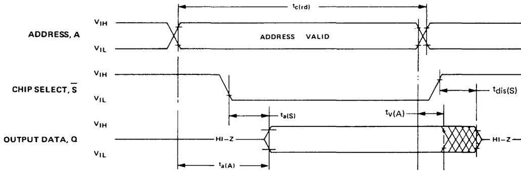
All timing reference points are 0.8 V and 2.0V on inputs and 0.6 V and 2.2 V on outputs (90% points). Input rise and fall times equal 10 nanoseconds.
