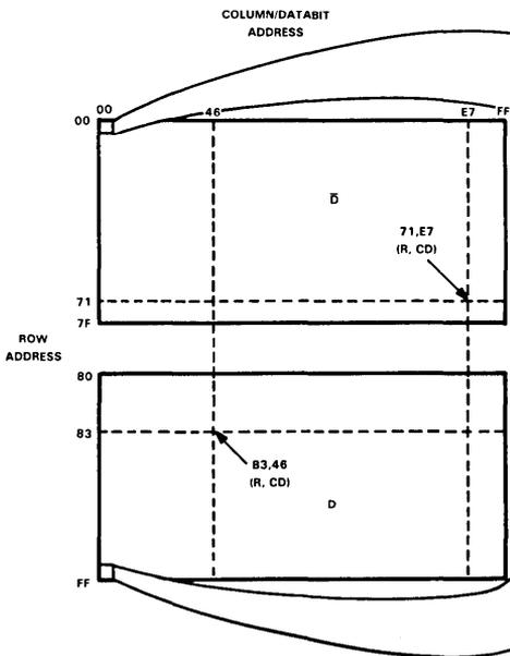
**FIGURE 1C – TMS 4416 ARRAY BIT MAP**
