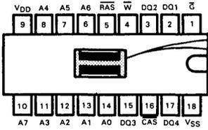
**FIGURE 1A – TMS 4416 PINOUT**
