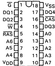
FIGURE 1 - TMS 4416 PIN CONFIGURATION
