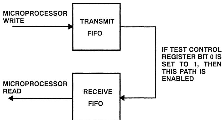
**Figure 3-1. Internal Loop-Back Path for FIFO Test**
