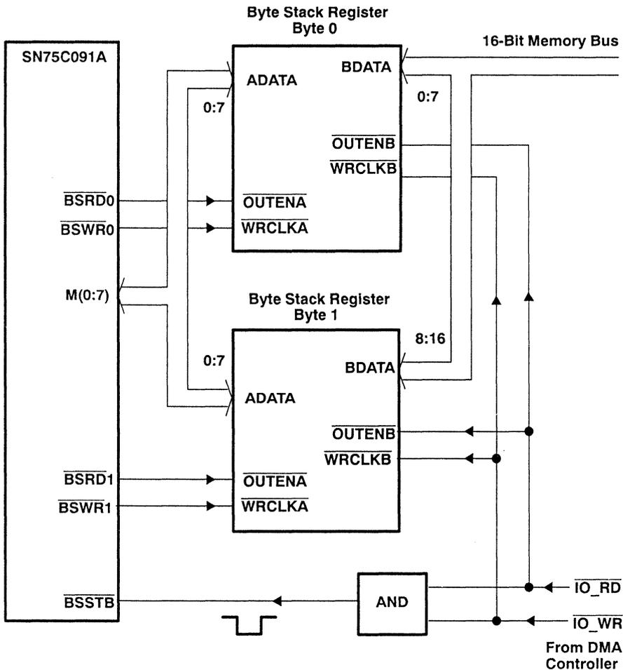
Note: The SBC  $\text{M}(0:7)$  bus provides an optional parity bit. Byte stack registers should be designed for nine-bit operation if this parity bit is used.
