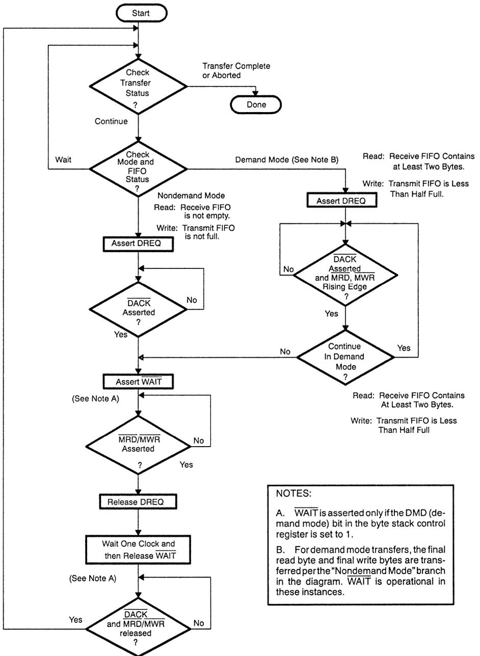
Figure 6-1. Flowchart for DMA Read/Write (Non-Byte-Stack Mode)
