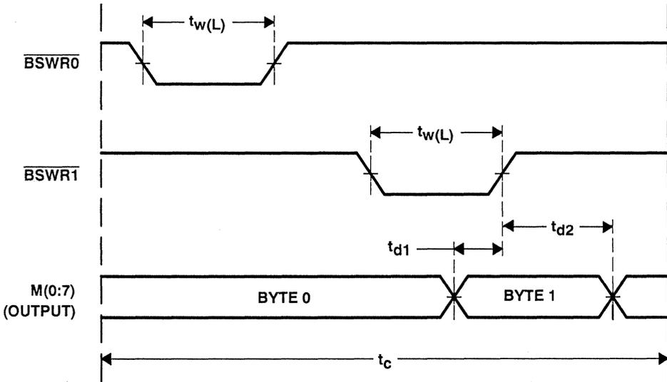
Figure 7-13. Byte Stack Load Cycle (16-bit)
