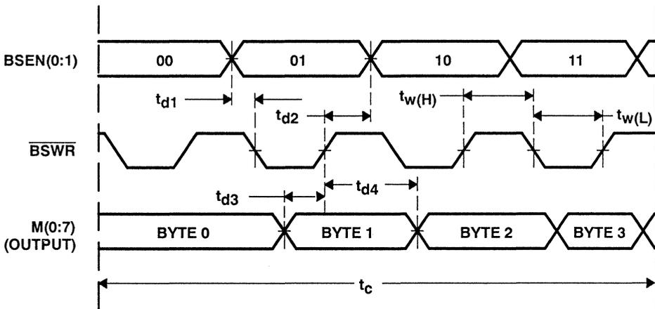
**Figure 7-15. Byte Stack Load Cycle (24- or 32-Bit)**
