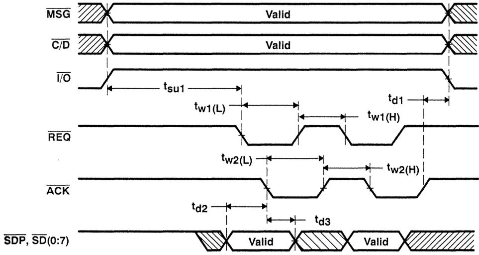
Figure 7-30. SCSI Bus Synchronous Data-Out Transfer (Initiator)
