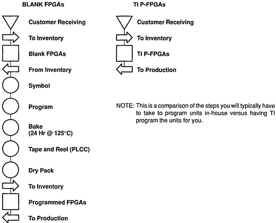
**Figure 6. Blank vs TI Programmed FPGA Process Steps**
