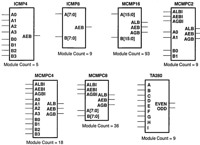
Figure 29. Comparators/Parity Checker
