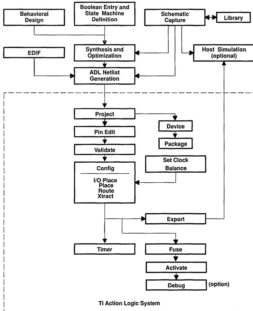
The TI FPGA design flow, as illustrated in Figure 3–2, simplifies and speeds design implementation at the user's desktop. The process is initiated within the host system environment in conjunction with the TPC Series macro libraries. Prelayout and postlayout simulations of the design can be performed within the host environment. When the host environment design processes are complete, the TI-ALS files are exported to the TI-ALS.
