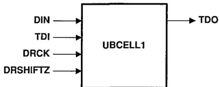
**Figure 6. Unidirectional Boundary Cell 1**
