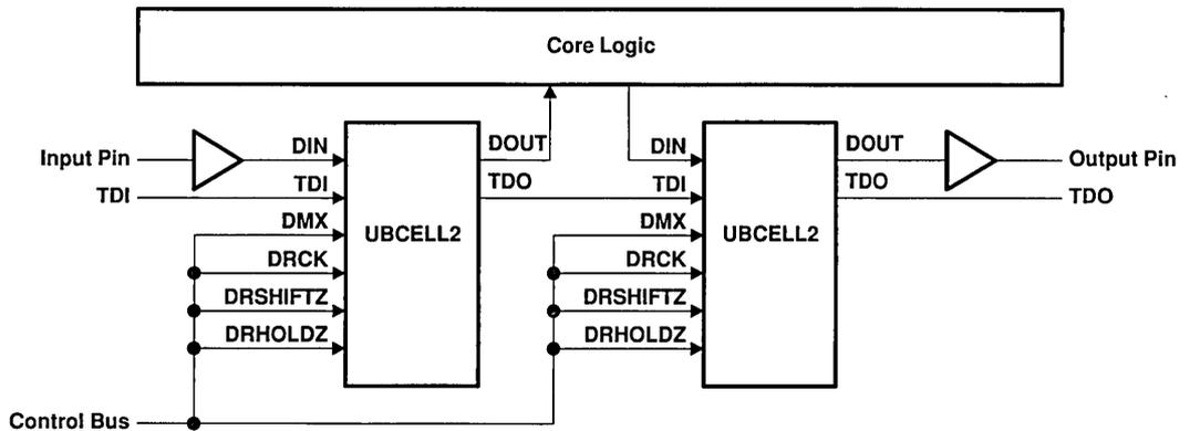
Figure 9. Boundary Register Using UBCELL2
