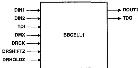
**Figure 10. Bidirectional Boundary Cell 1**
