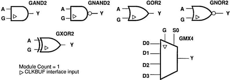
Figure 33. Clock Buffer (CLKBUF) Interface
