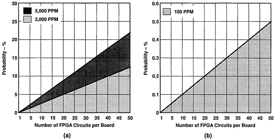
Figure 5. Defect Probability vs PPM Level
