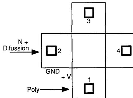
Test devices were stressed by forcing a constant 5 mA current from polysilicon to N+ through the antifuse at 250°C. Note that this stress is far greater than a programmed antifuse would see in a device under normal operating conditions. Because the antifuse is used to connect two networks together, there is usually no voltage across it and hence no current passes through. A voltage will appear across the antifuse only momentarily while a network switches from low-to-high or high-to-low.
