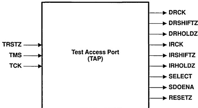
Figure 1. Test Access Port (TAP)
