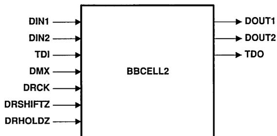
**Figure 12. Bidirectional Boundary Cell 2**
