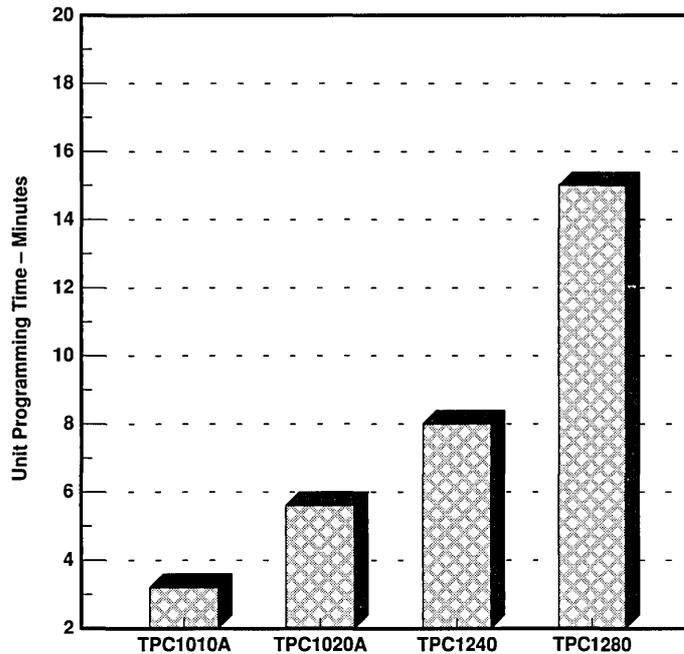
**Figure 1. FPGA Per Unit Programming Time**
