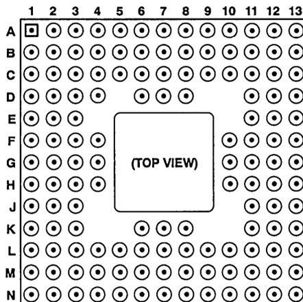
I/O Pin Assignments for the 133-Pin Ceramic Pin Grid Array Package
