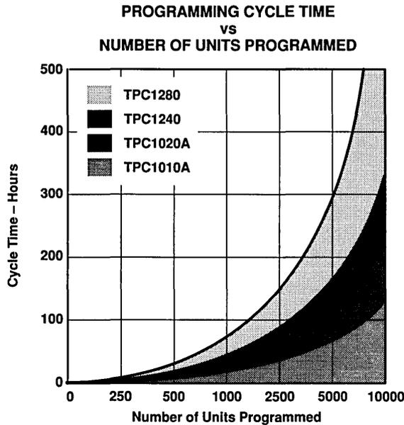
**Figure 2. FPGA Programming Cycle Time**
