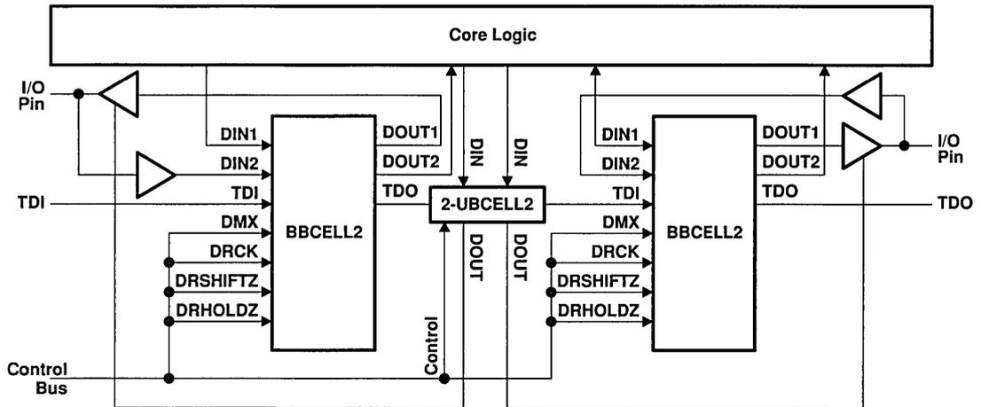
Figure 13. Boundary Register Using BBCELL2
