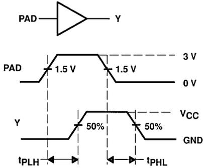
NOTE: Measurements made with  $t_r = t_f = 3$  ns to pads only.
