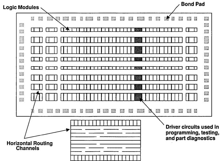
Figure 1-2. Architecture Detail
