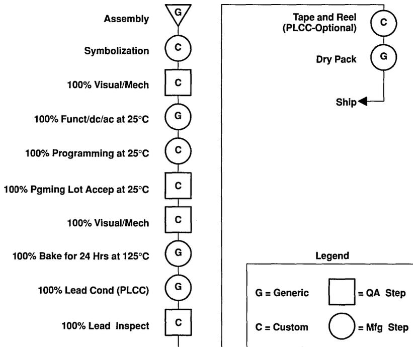
**Figure 7. TI P-FPGA Factory Process Flow**
