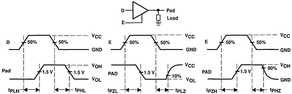
Figure 5. Symbols, Test Loads, and Waveforms
