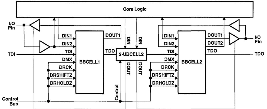
Figure 11. Boundary Register Using BBCELL1
