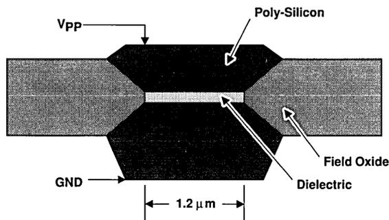
Metal routing tracks run horizontally and vertically over the die, with an antifuse at each intersection. The unprogrammed resistance of the antifuse is greater than 100 M $\Omega$  and the programmed resistance is approximately 500  $\Omega$ .
