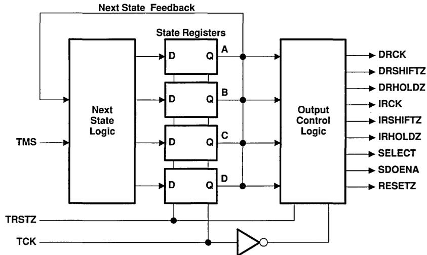
**Figure 2. TAP Block Diagram**
