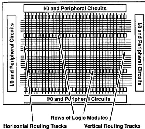
Figure 1. Diagram of TPC14 Series Architecture
