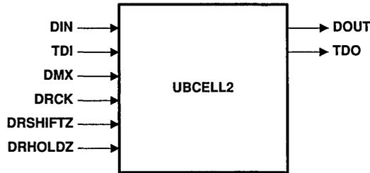
**Figure 8. Unidirectional Boundary Cell 2**
