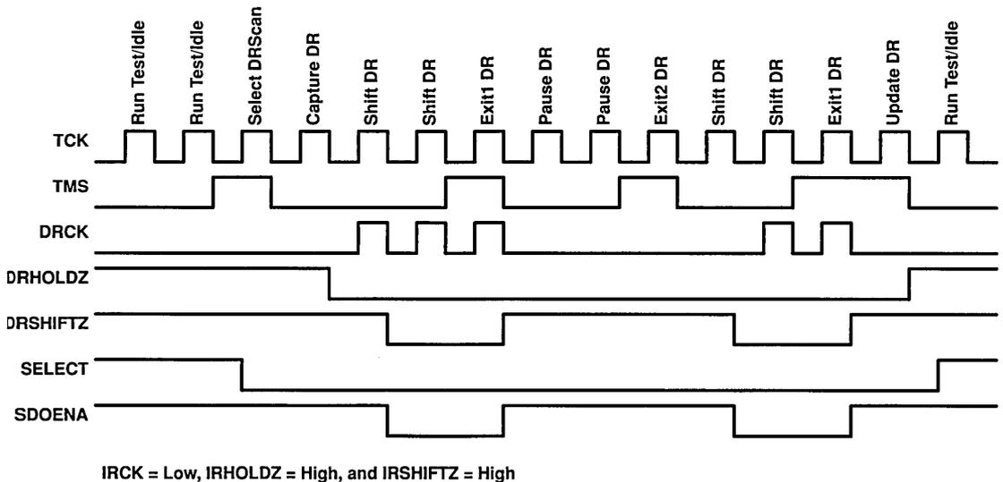
**Figure 4. TAP Data Register Scan Timing Diagram**
