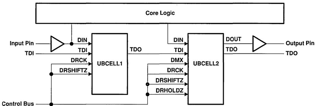
**Figure 7. Boundary Register Using UBCELL1**
