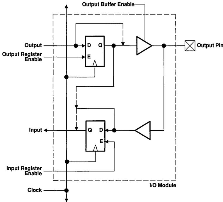
Figure 3. I/O Module With Registered Inputs and Outputs
