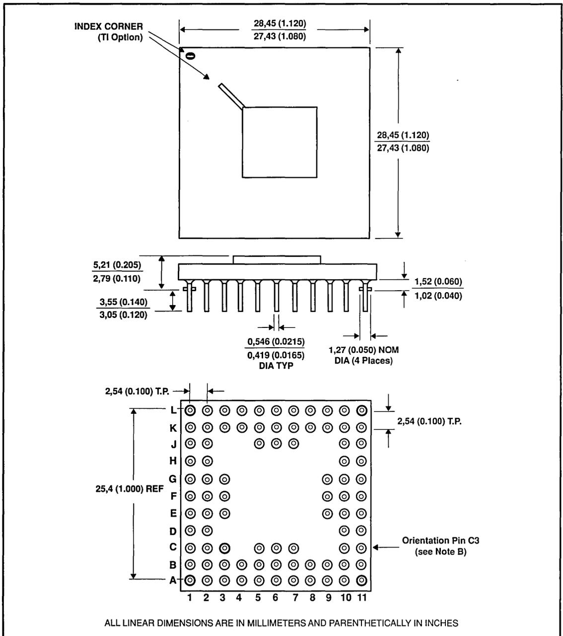
NOTES: A. Pins are located within 0,13 (0.005) radius of true position relative to each other at maximum material condition and within 0,381 (0.051) radius relative to the center of the ceramic.
