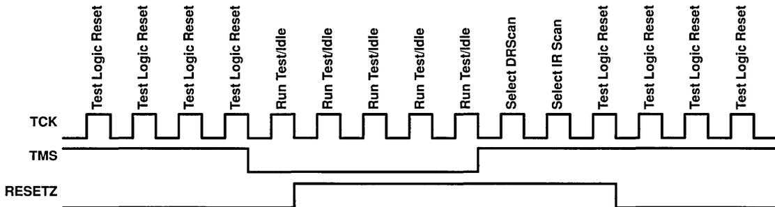
**Figure 5. TAP Test Logic Reset Timing Diagram**
