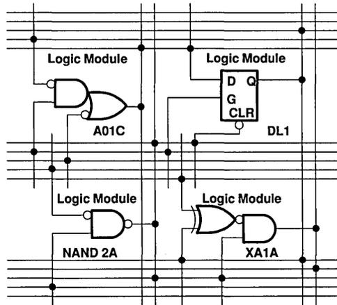
Figure 2. Partial View of TPC10 Series Interconnection Capability
