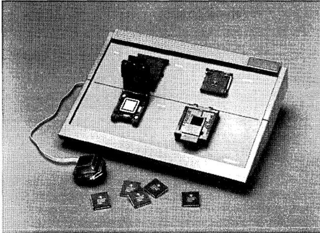
Figure 3-4. Activator 2 Programmer
