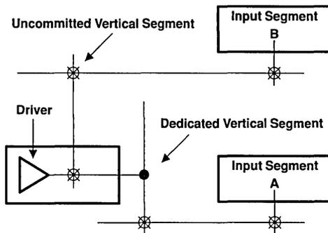
Figure 1. TPC12 Enhanced Routing Architecture
