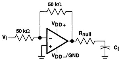
**Figure 55. Series-Resistance Circuit**
