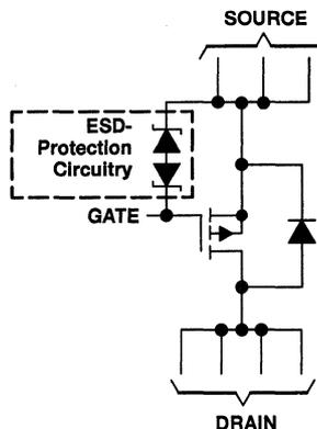
NOTE: For all applications, all source pins should be connected and all drain pins should be connected.
