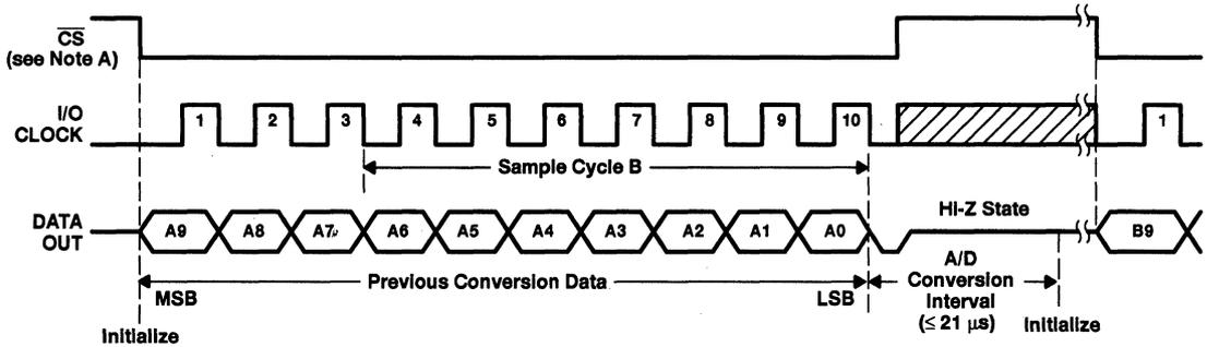
**Figure 6. Timing for 10-Clock Transfer Using  $\overline{CS}$**
