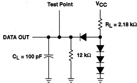
**Figure 2. Load Circuit**
