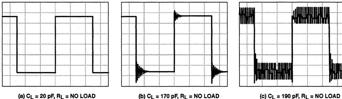
Figure 106. Effect of Capacitive Loads in Medium-Bias Mode
