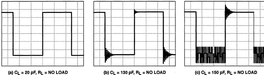
Figure 105. Effect of Capacitive Loads in High-Bias Mode
