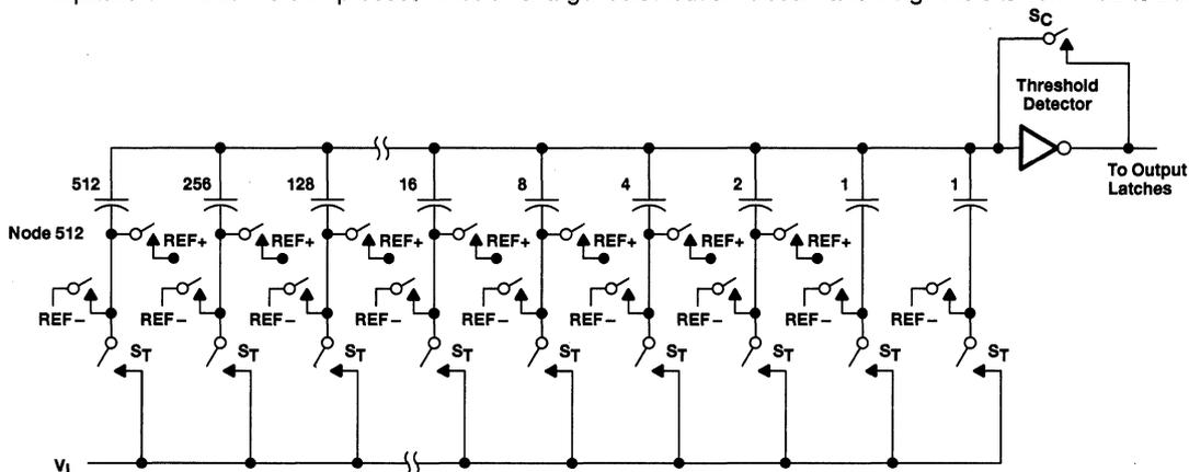
**Figure 1. Simplified Model of the Successive-Approximation System**
