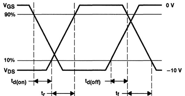
Figure 2. Switching-Time Waveforms
