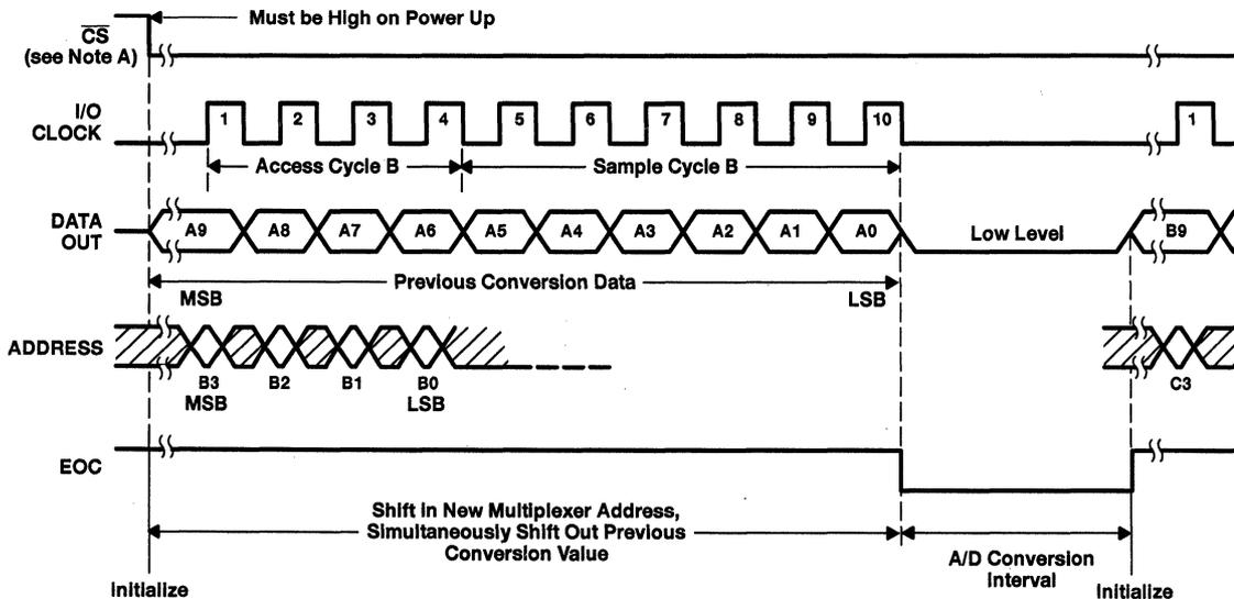
**Figure 10. Timing for 10-Clock Transfer Not Using  $\overline{CS}$**
