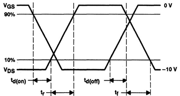
Figure 2. Switching-Time Waveforms
