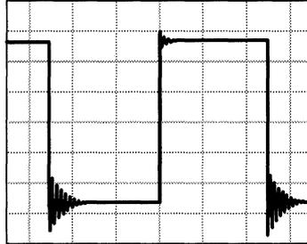
(b)  $C_L = 130 \text{ pF}$ ,  $R_L = \text{NO LOAD}$
