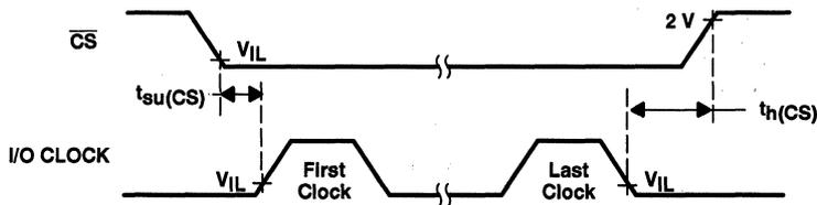
Figure 5. CS and I/O CLOCK Voltage Waveforms
