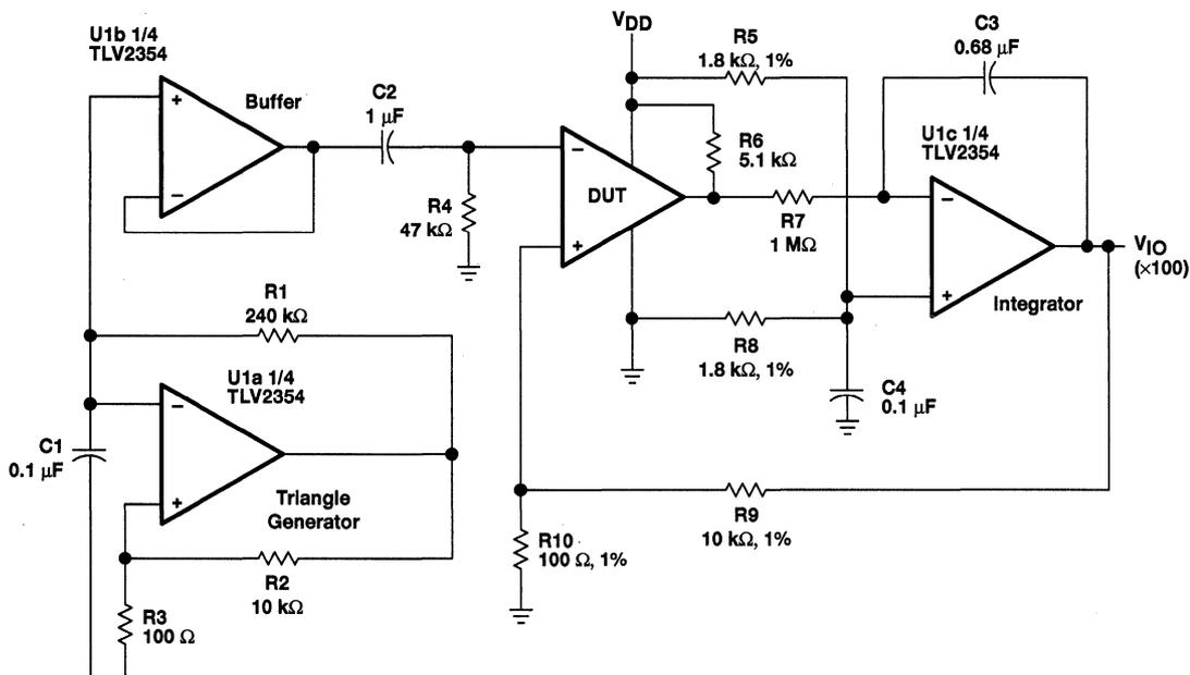
Figure 10. Circuit for Input Offset Voltage Measurement
