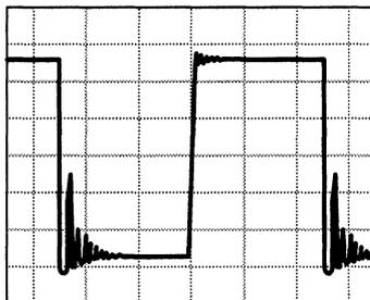
(b)  $C_L = 260 \text{ pF}$ ,  $R_L = \text{NO LOAD}$
