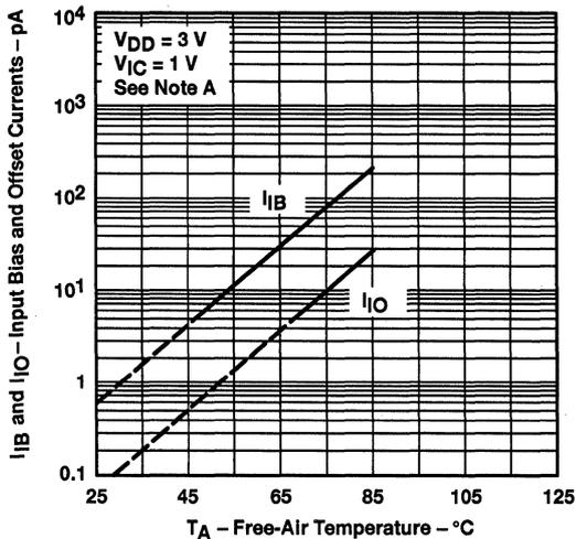
NOTE A: The typical values of input bias current and input offset current below 5 pA were determined mathematically.
