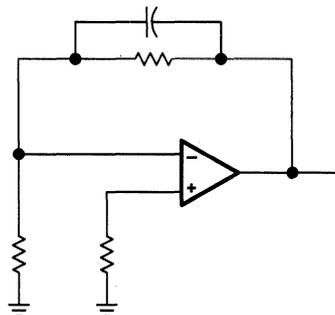
Figure 102. Compensation for Input Capacitance
