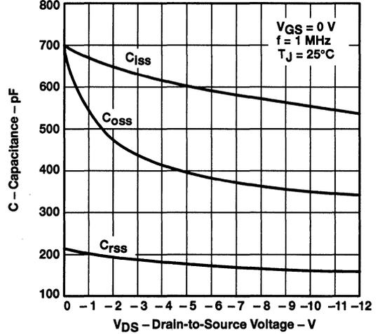
$$^\dagger C_{iss} = C_{gs} + C_{gd}, C_{ds}(\text{shorted}),$$
