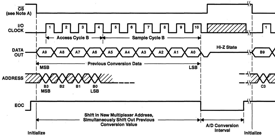
**Figure 9. Timing for 10-Clock Transfer Using  $\overline{CS}$**
