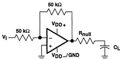
**Figure 55. Series-Resistance Circuit**
