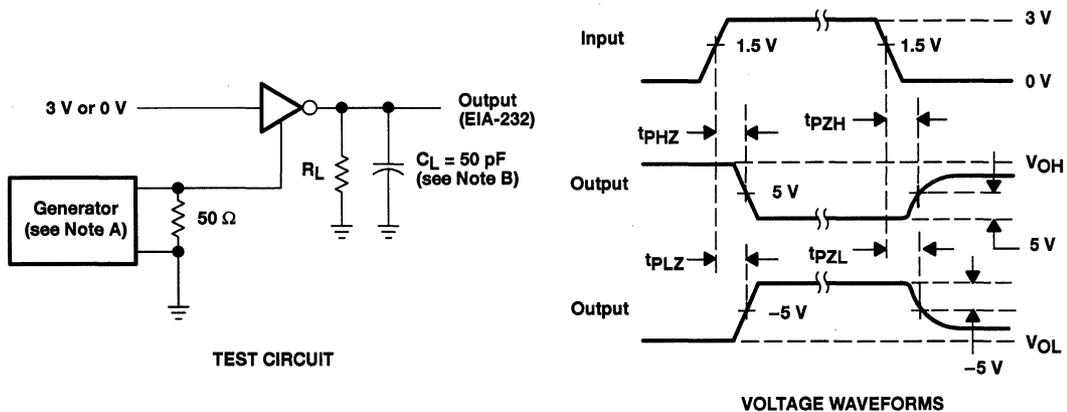
Figure 3. Driver Test Circuit and Voltage Waveforms
