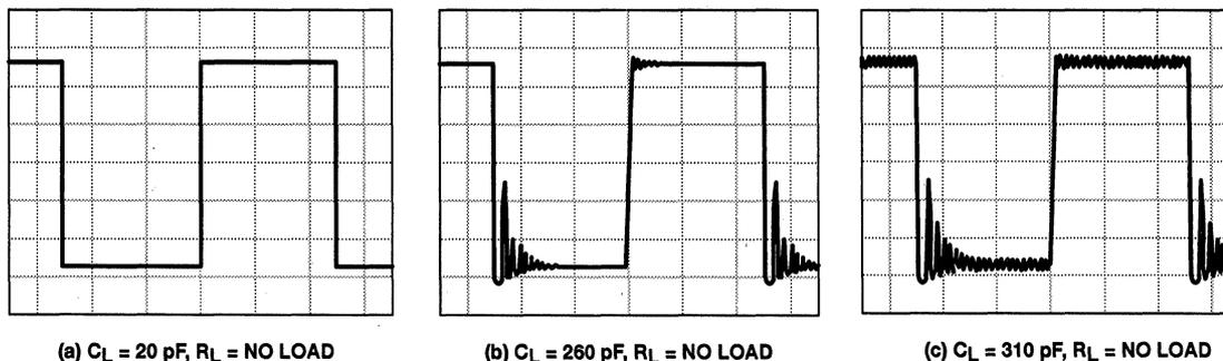
Figure 107. Effect of Capacitive Loads in Low-Bias Mode
