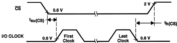
**Figure 4.  $\overline{\text{CS}}$  to I/O CLOCK Voltage Waveforms**
