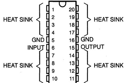
HEAT SINK – These pins have an internal resistive connection to ground and should be grounded.
