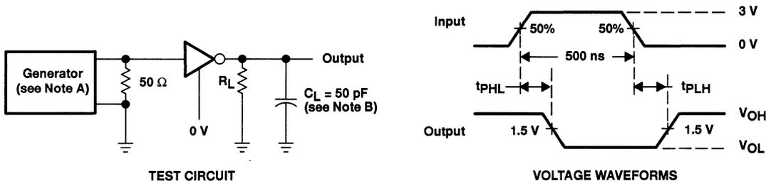
Figure 5. Receiver Test Circuit and Voltage Waveforms
