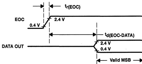
**Figure 8. EOC and DATA OUT Voltage Waveforms**
