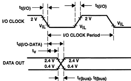
**Figure 6. DATA OUT and I/O CLOCK Voltage Waveforms**
