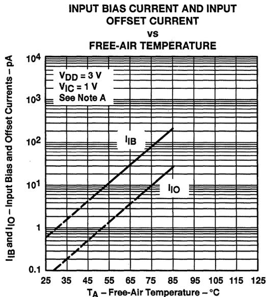
NOTE: The typical values of input bias current and input offset current below 5 pA were determined mathematically.
