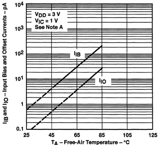
NOTE: The typical values of input bias current and input offset current below 5 pA were determined mathematically.
