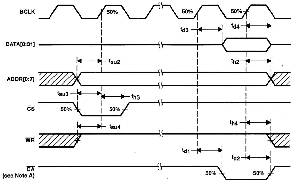
NOTE A: When back-to-back read cycles are done, a maximum of 9 BCLK cycles may be required after the falling edge of  $\overline{CS}$  and before  $\overline{CA}$  is asserted (low). ADDR[0:7] and  $\overline{WR}$  need to remain valid until  $\overline{CA}$  is asserted (low).
