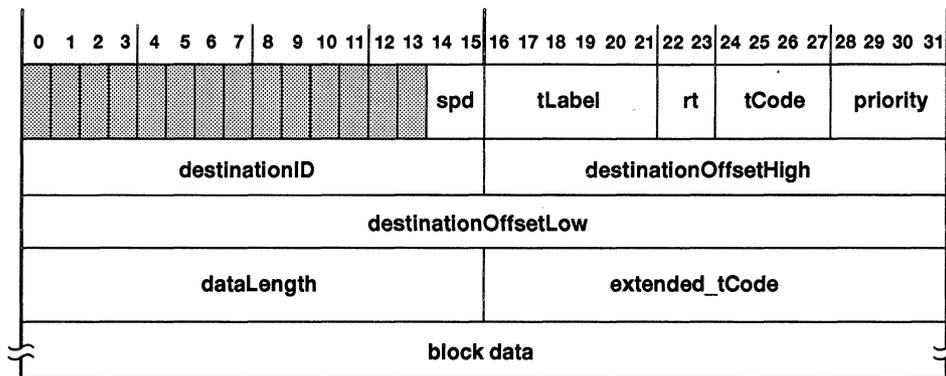
**Figure 4–2. Block-Transmit Format**
