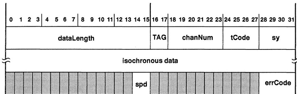
Figure 4–6. Isochronous-Receive Format
