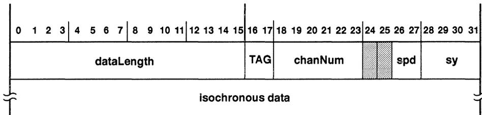
Figure 4–5. Isochronous-Transmit Format
