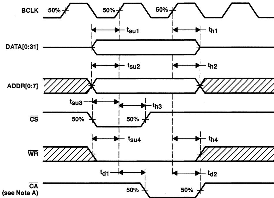
NOTE A: When back-to-back write cycles are done, a maximum of 9 BCLK cycles may be required after the falling edge of  $\overline{CS}$  before  $\overline{CA}$  is asserted (low). DATA[0:31], ADDR[0:7], and  $\overline{WR}$  need to remain valid until  $\overline{CA}$  is asserted (low).
