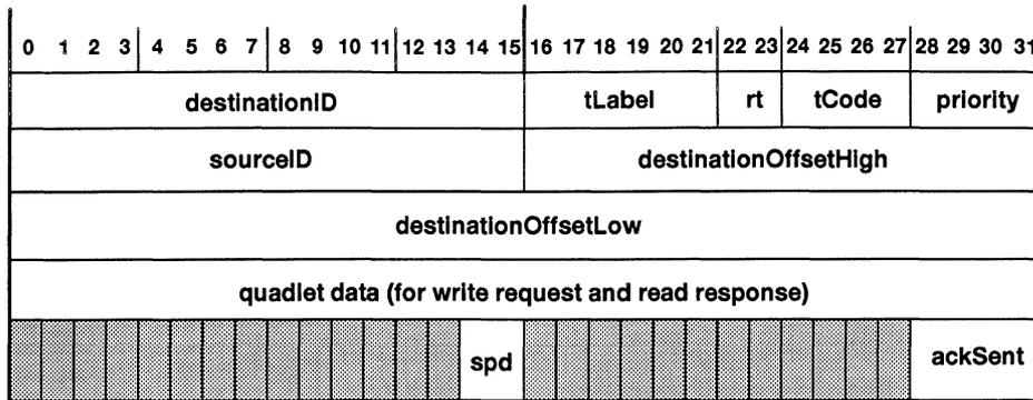
Figure 4–3. Quadlet-Receive Format
