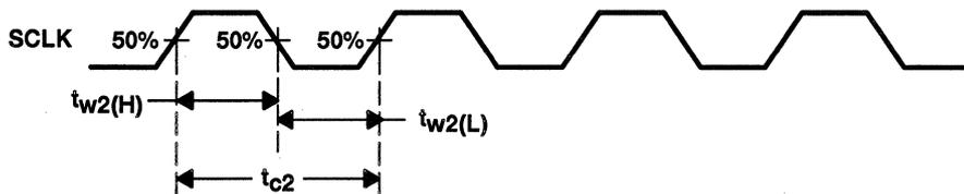
Figure 6-4. SCLK Waveform
