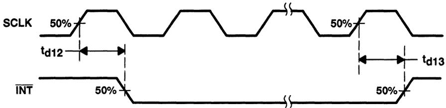
Figure 6-8. Interrupt Waveform
