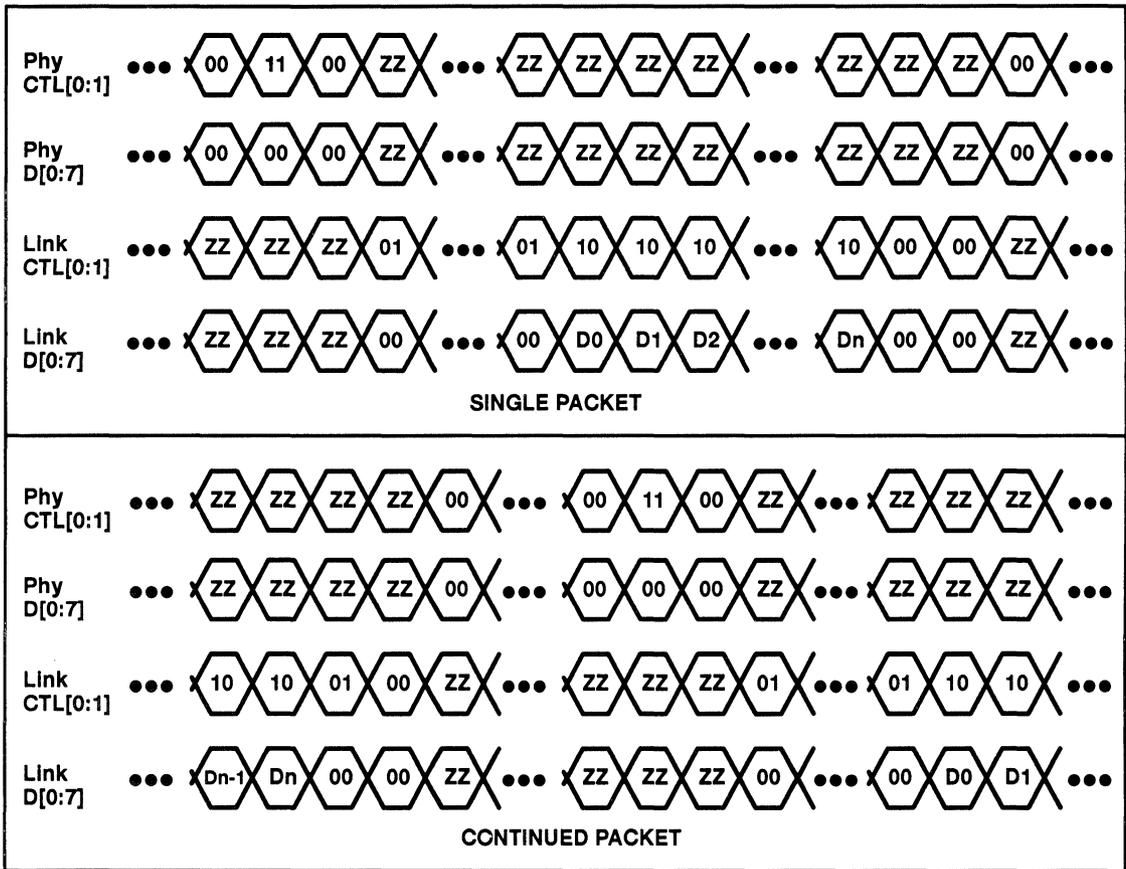
NOTE A: ZZ = high-impedance state, D0 – Dn = packet data
