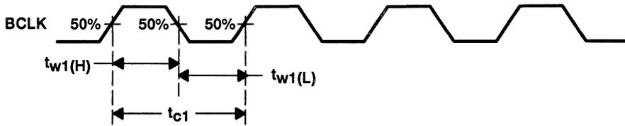
Figure 6-1. BCLK Waveform
