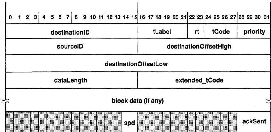
**Figure 4–4. Block-Receive Format**
