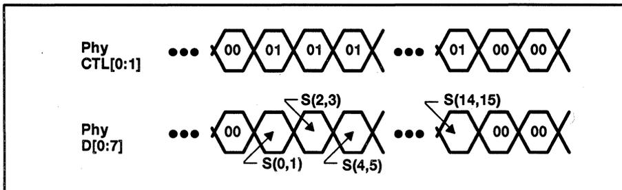
**Figure 7–3. Status-Transfer Timing**
