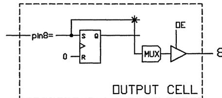
Signal specifications for pin8.s and pin8.r are not permitted. All cells of the reset term are programmed as if
