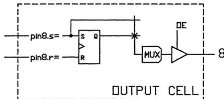
No signal specification for pin8.s and pin8.r is permitted.
