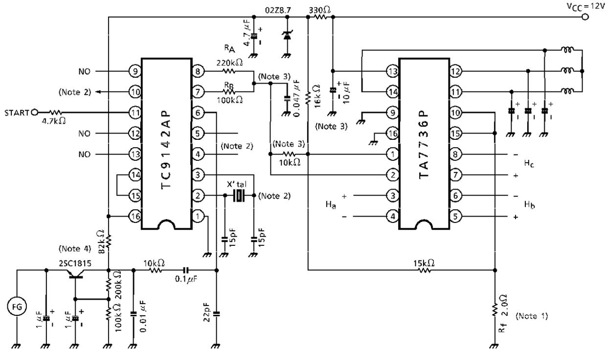
(Note 1)  $R_f$  is a feed back Resistor that's voltage drop is equal to Input Voltage ( $V_2 - V_1$ ) in this application with feed back by Zener Diode.
