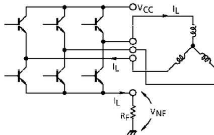
Further, if inputs (pin①, ⑤, pin②, ⑥) are shorted or  $V_1 \geq V_2$ , torque at the circuit, becomes zero. However, this zero torque state also can be obtained by setting FRS input (pin⑩, ④) to specified voltage or by placing the circuit in open state and this is rather advantageous as current consumption is less.
