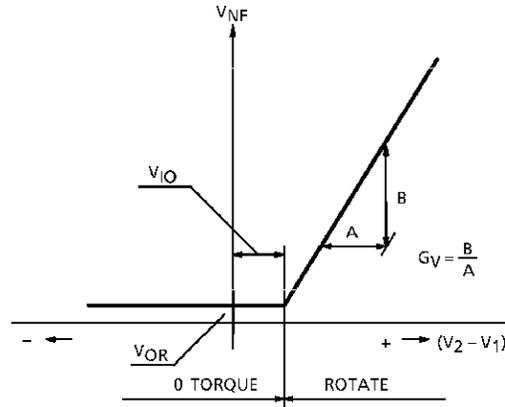
$V_{NF}$  shows voltage drop at  $R_F$ .
