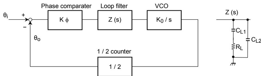
The transfer function ( $F(S)$ ), the angular frequency ( $\omega_n$ ), and the dumping factor ( $\zeta$ ) of the above composition are defined as following (However  $C_{L2}$  is ignored as  $C_{L2} \ll C_{L1}$ ):
