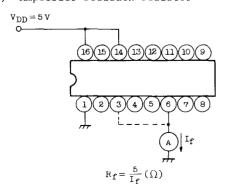
(6) D/A Converter ladder resistor  $\overline{R_L}$
