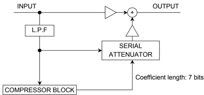
**Figure 6 Dynamic Digital Bass Boost Circuit Block**
