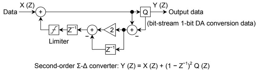
**Figure 9  $\Sigma$ - $\Delta$  Modulation DA Converter**
