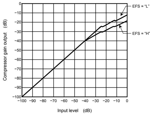
**Figure 7 Dynamic Digital Bass Boost Compressor I/O Characteristics**
