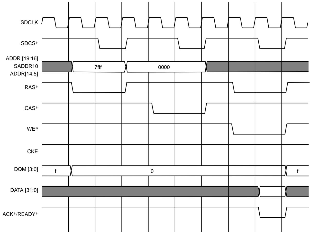
Figure 9.5.2 Single Read ( $t_{RCD} = 3$ ,  $t_{CASL} = 3$ ,  $t_{DA} = 1$ , 32-bit Bus)
