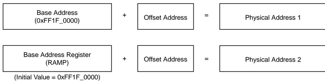
Figure 4.2.1 Generating Physical Address for a Internal Register
