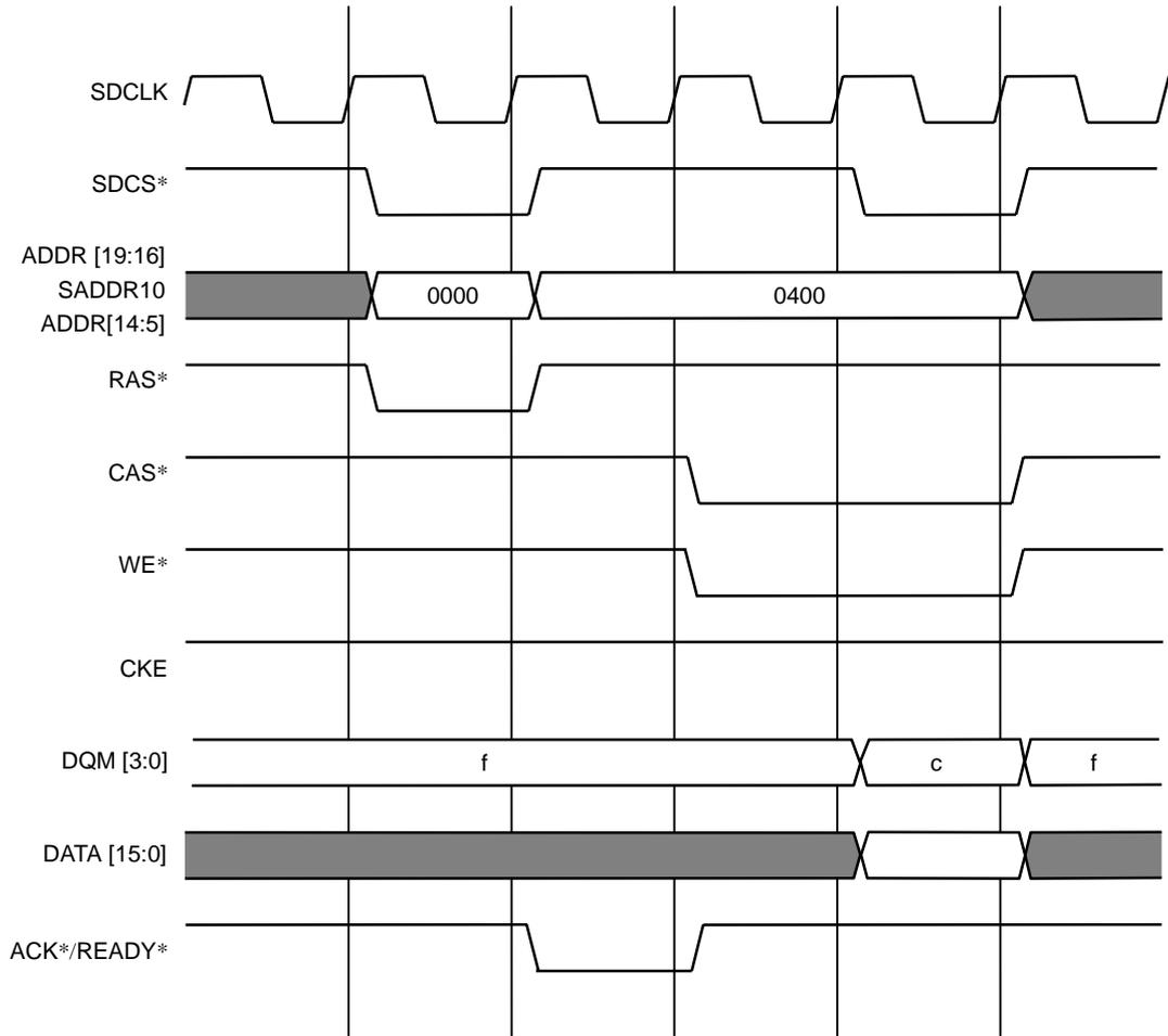
Figure 9.5.11 Half-Word Single Write ( $t_{RCD} = 3$ ,  $t_{DA} = 0$ , 16-bit Bus)
