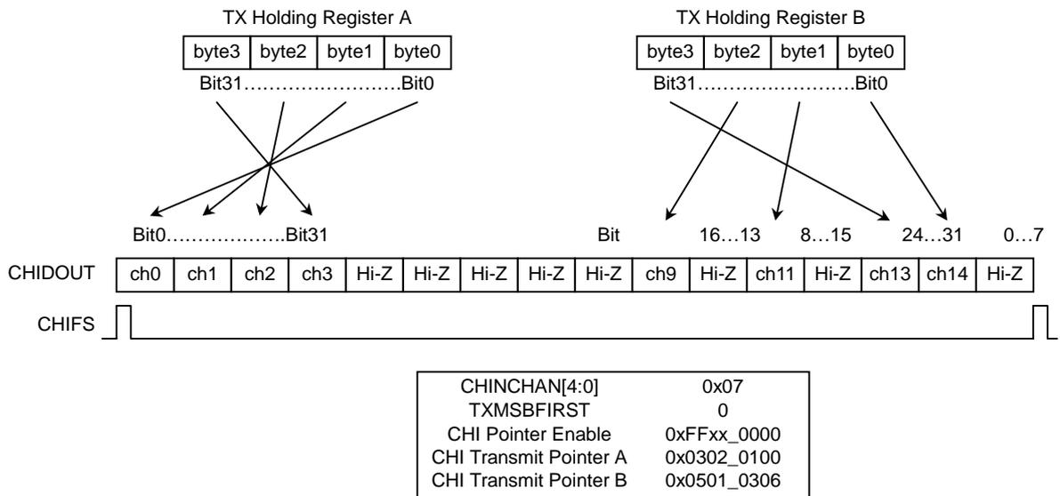
Figure 16.3.1 Transmit TDM Switch Example
