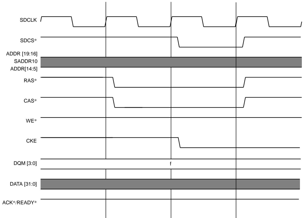
Figure 9.5.12 Transition to Low Power Consumption Mode (SDCTR.ACE = 0)
