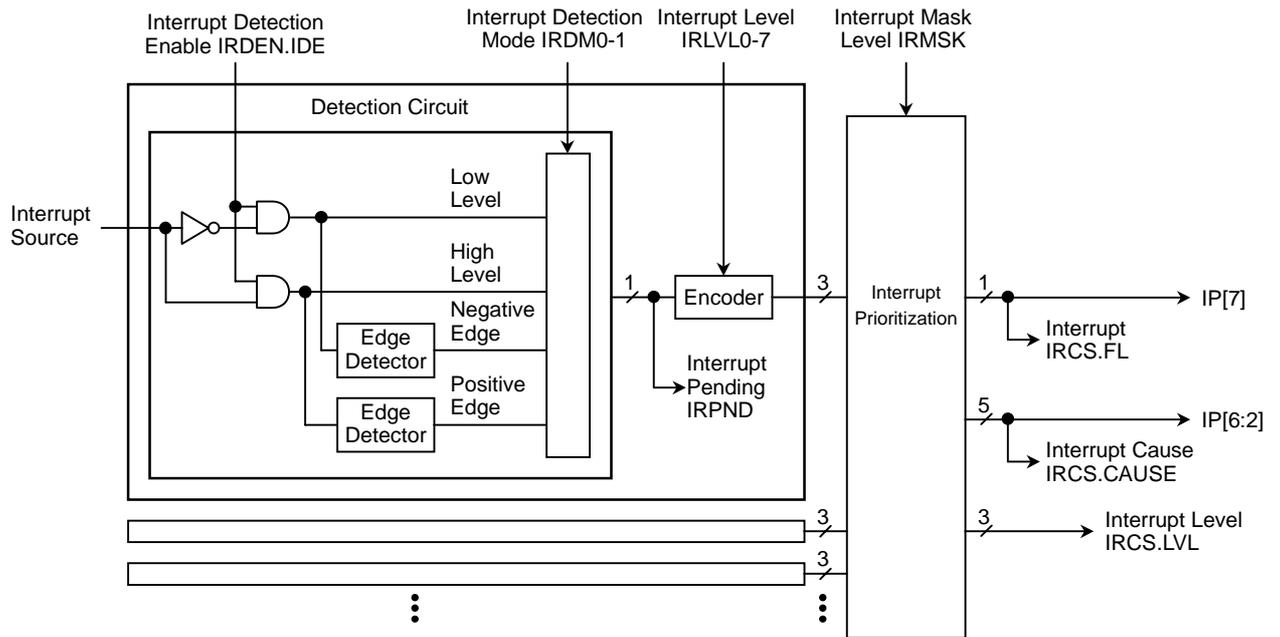
Figure 15.2.2 Internal Block Diagram of Interrupt Controller
