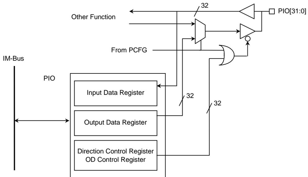
Figure 13.2.1 Parallel I/O Block Diagram
