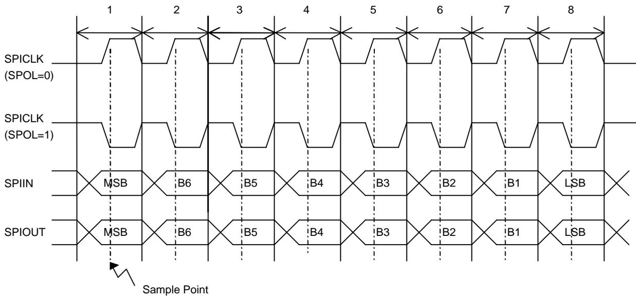
Figure 17.3.1 Transfer format when SPHA is "0".
