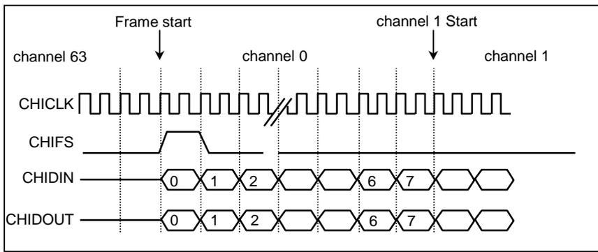
Figure 16.3.8 CHI Frame Structure Example
