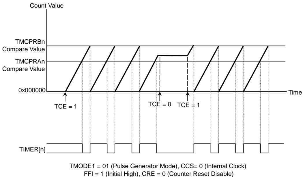
Figure 12.3.3 Operation Example of the Pulse Generator Mode
