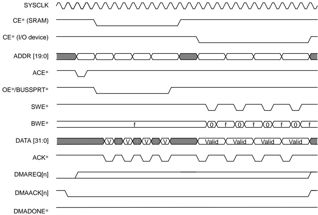
Figure 8.5.17 Dual Address Transfer from SRAM to External I/O Device
