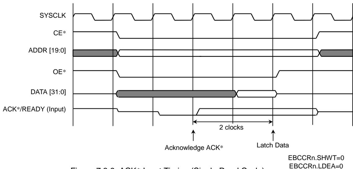
Figure 7.3.9 ACK\* Input Timing (Single Read Cycle)
