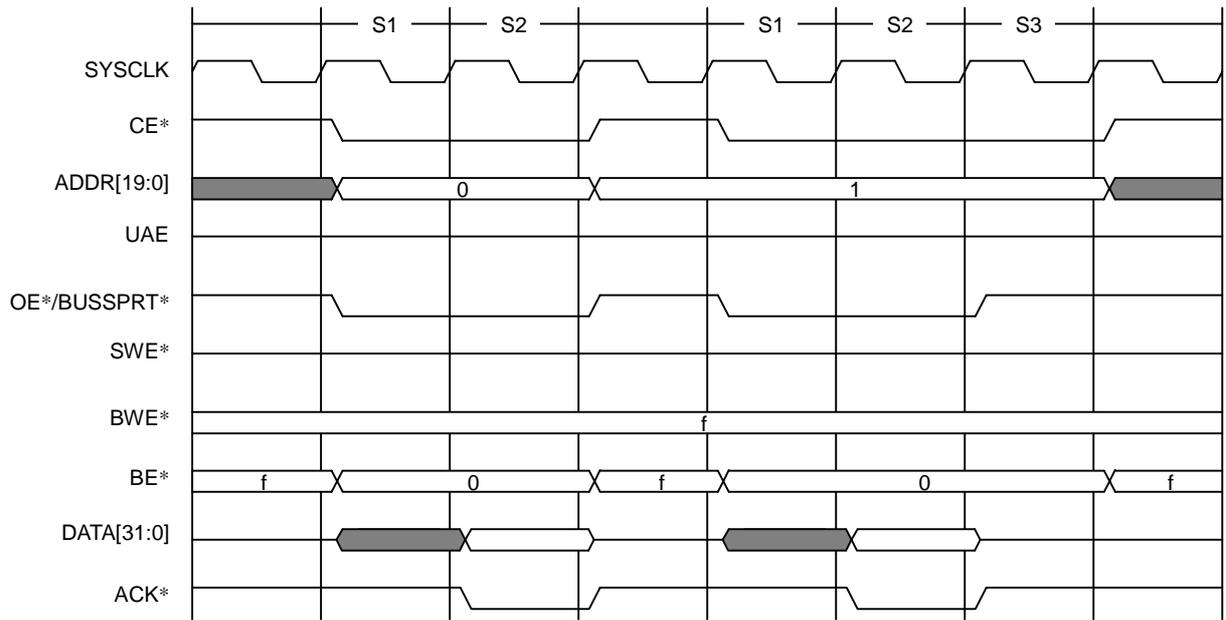
Figure 7.5.4 Double-word Single Read (PWT: WT=0, SHWT=0, Normal, 32-bit Bus)
