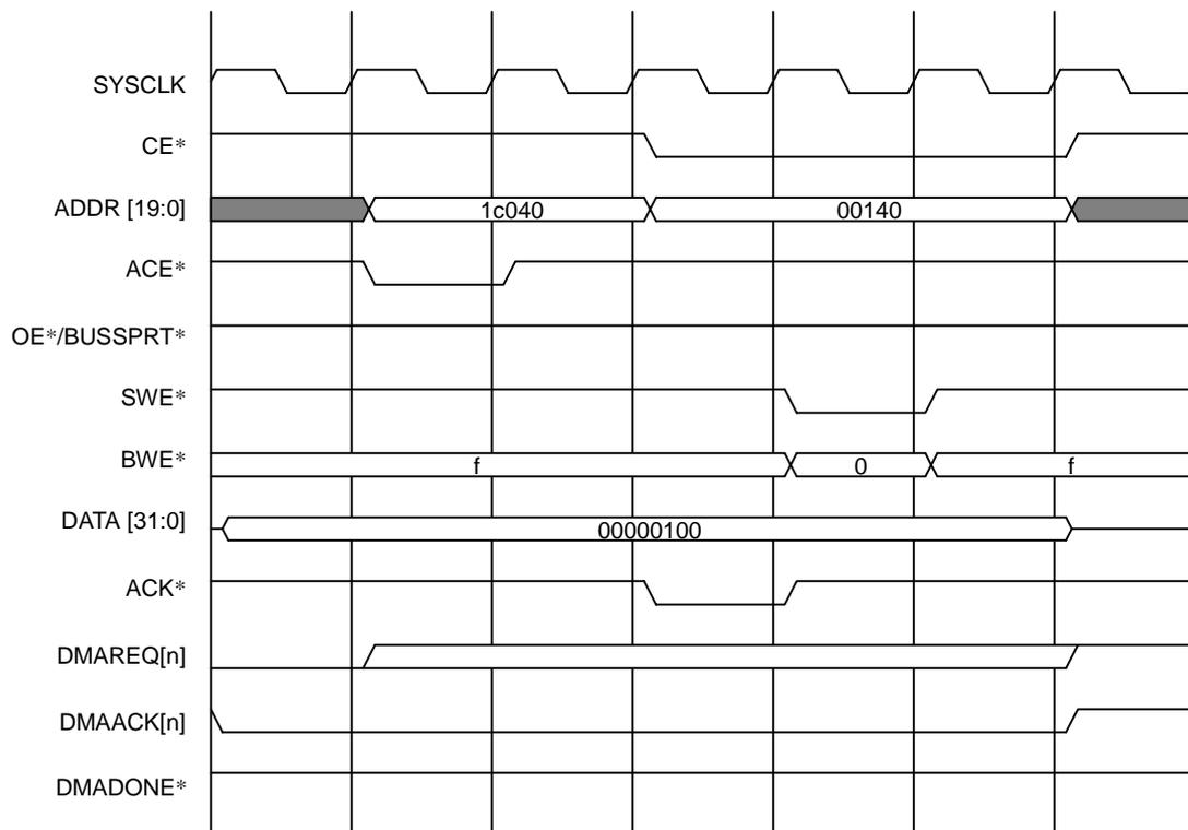
Figure 8.5.3 Single Address Single Transfer from I/O to Memory
