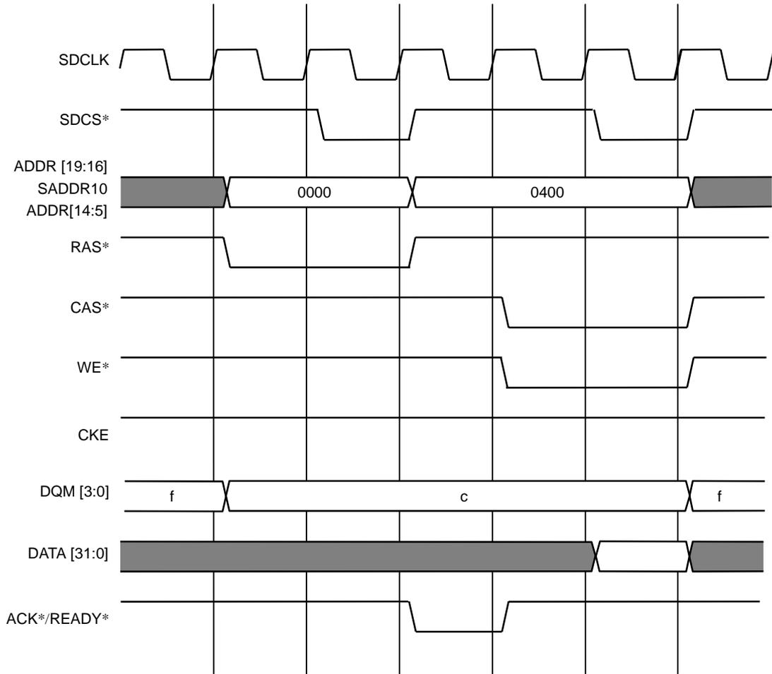
Figure 9.5.4 Half-Word Single Write ( $t_{RCD} = 3$ ,  $t_{DA} = 1$ , 32-bit Bus)
