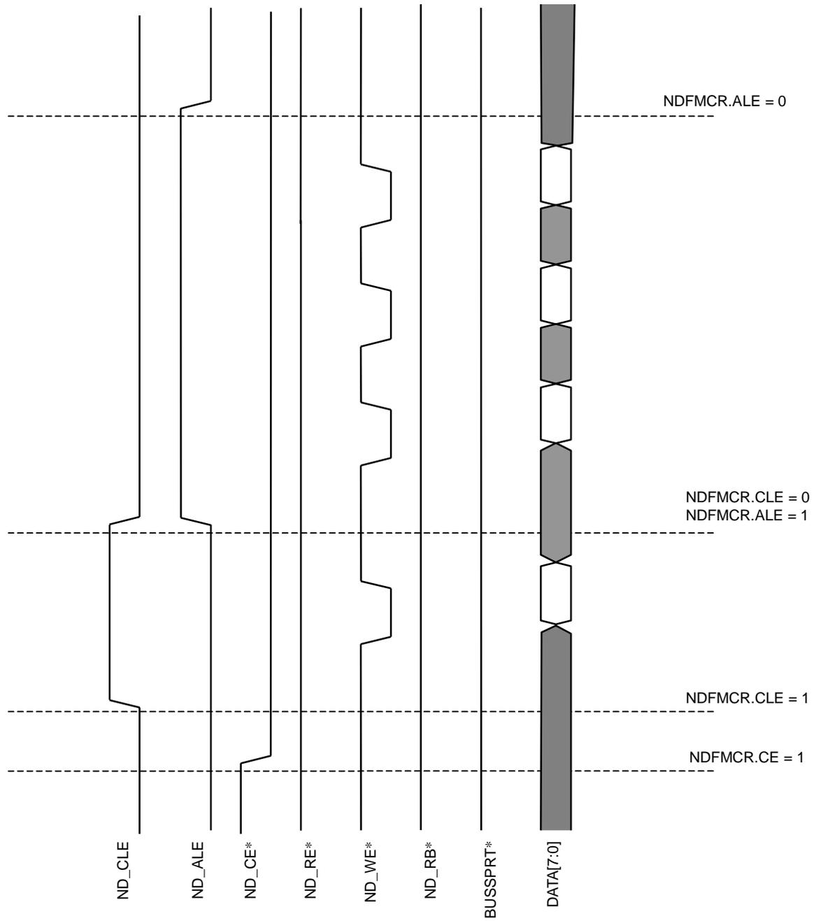
Figure 18.5.1 Command and Address Cycle (NDFMCR.BSPRT = 0)
