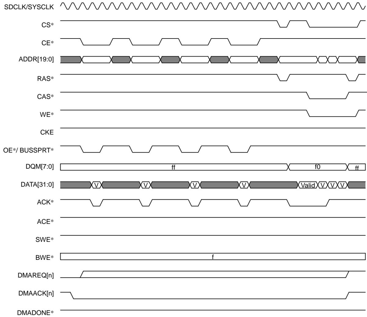
Figure 8.5.20 Dual Address Transfer from External I/O Device (Non-Burst) to SDRAM
