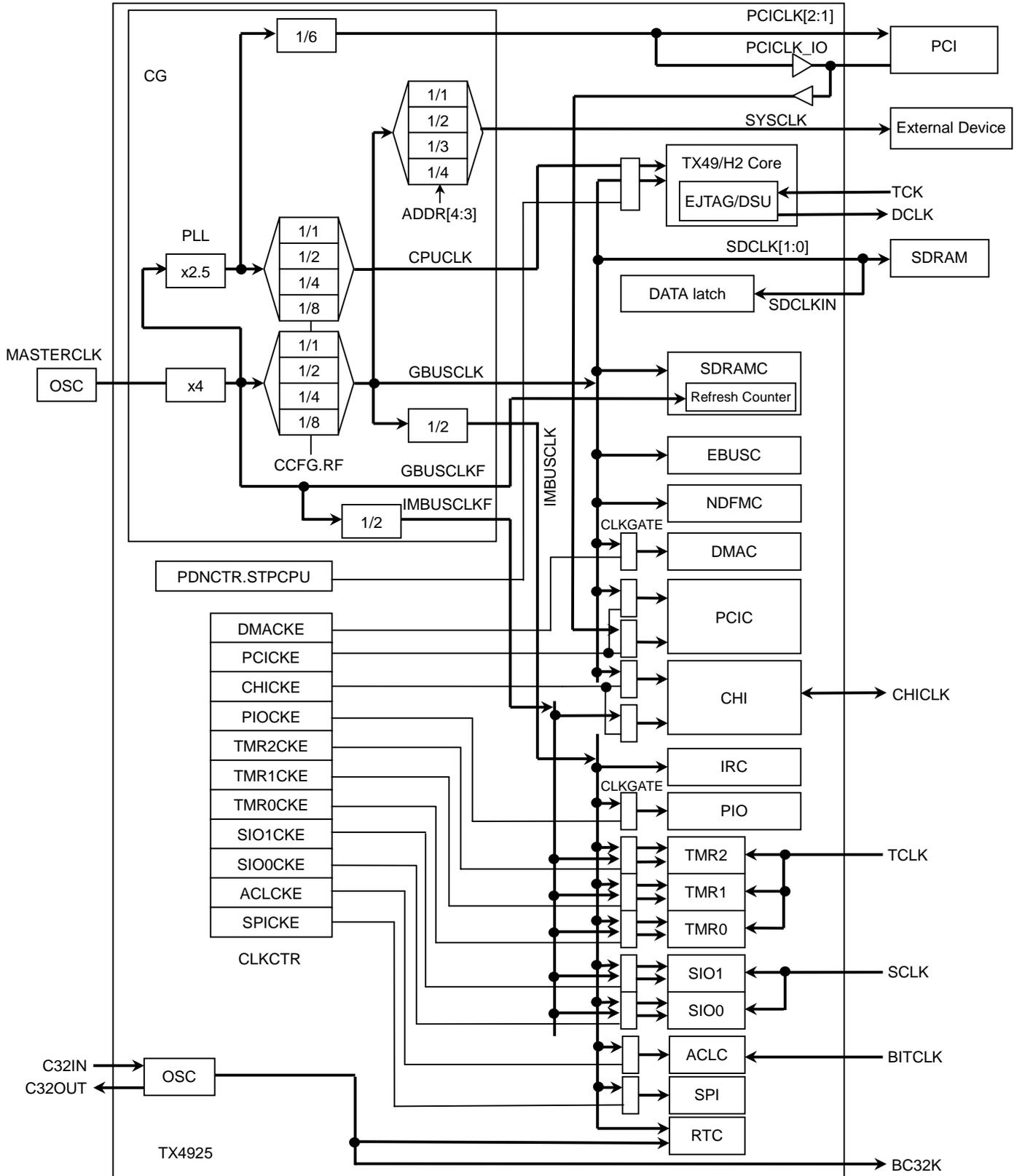
Figure 6.1.1 TX4925 Block and Clock Configuration
