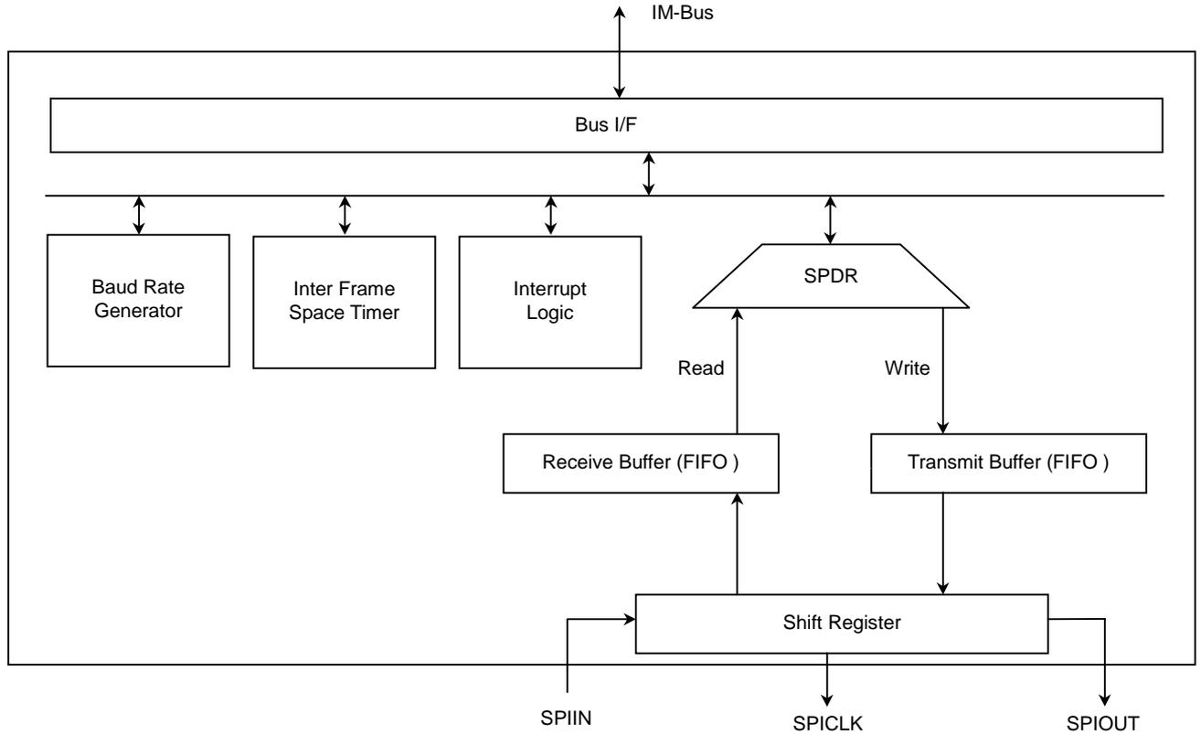
Figure 17.2.1 SPI Block Diagram
