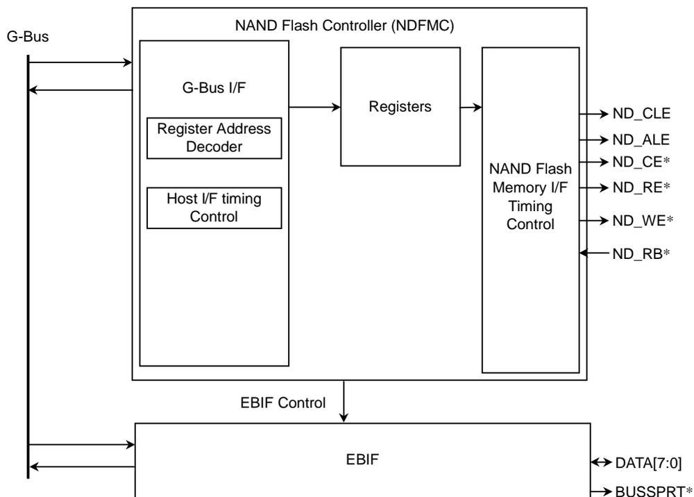
Figure 18.2.1 NAND Flash Memory Controller Block Diagram
