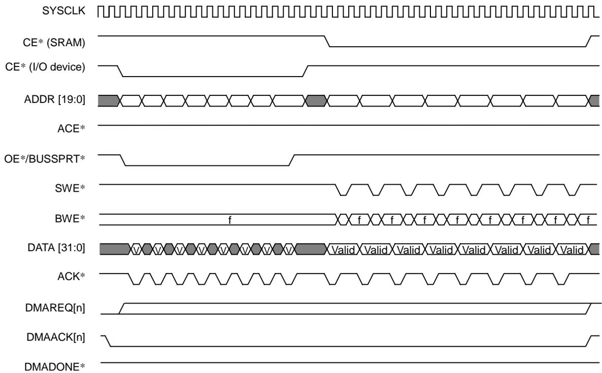
Figure 8.5.16 Dual Address Transfer from External I/O Device to SRAM
