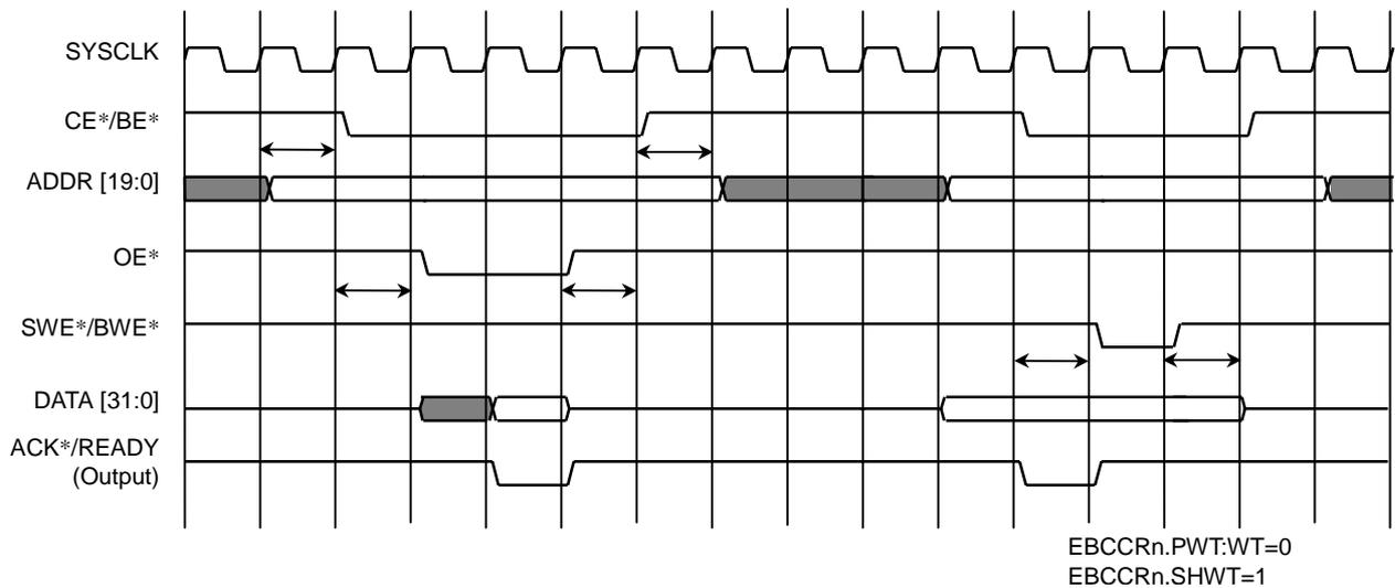
Figure 7.3.6 SHWT 1 Wait (Normal Mode, Single Read/Write Cycle)
