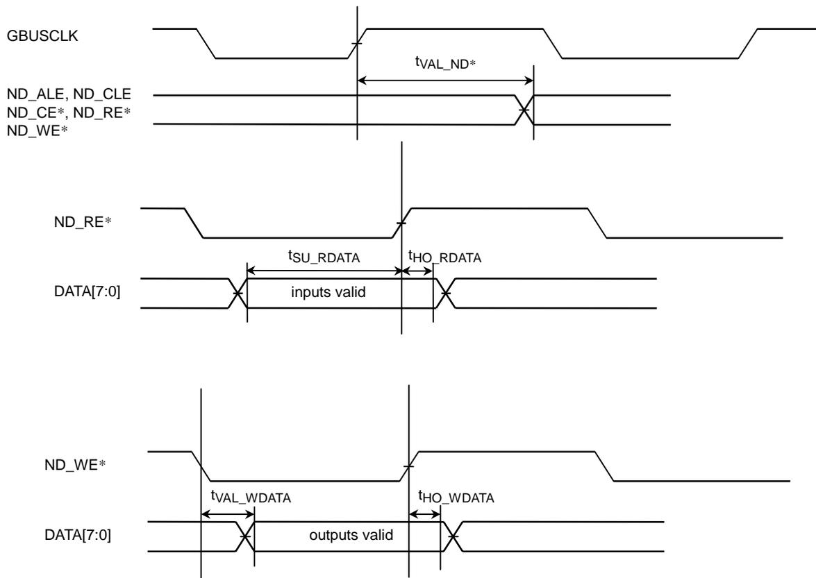
Figure 22.5.14 Timing Diagrams: NAND Flash Memory Interface
