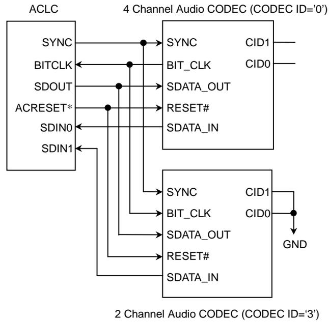
Figure 14.3.2 5.1 Channel Audio Connection Diagram
