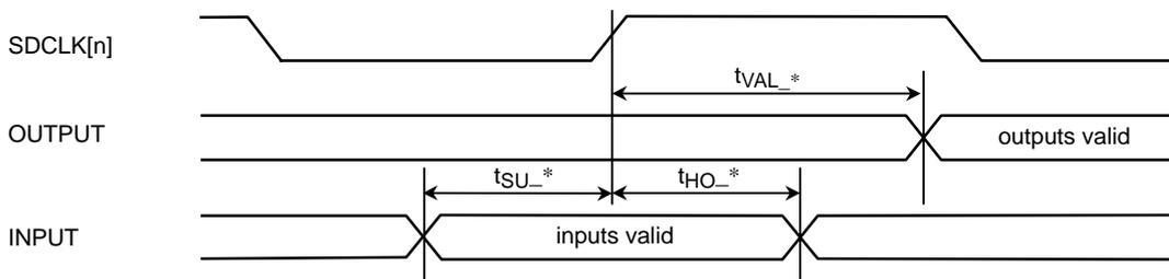
Figure 22.5.3 Timing Diagrams: Output Signals and When Bypass Mode Input Signals (SDCLK Basis)
