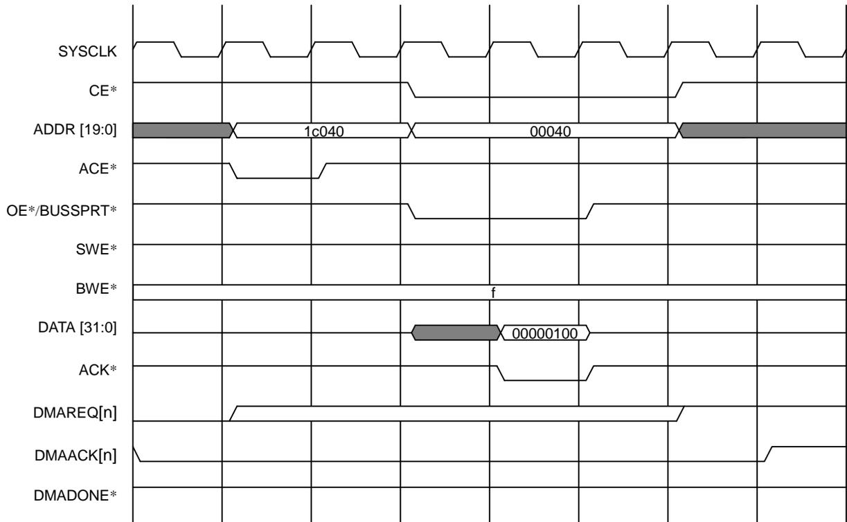
Figure 8.5.1 Single Address Single Transfer from Memory to I/O
