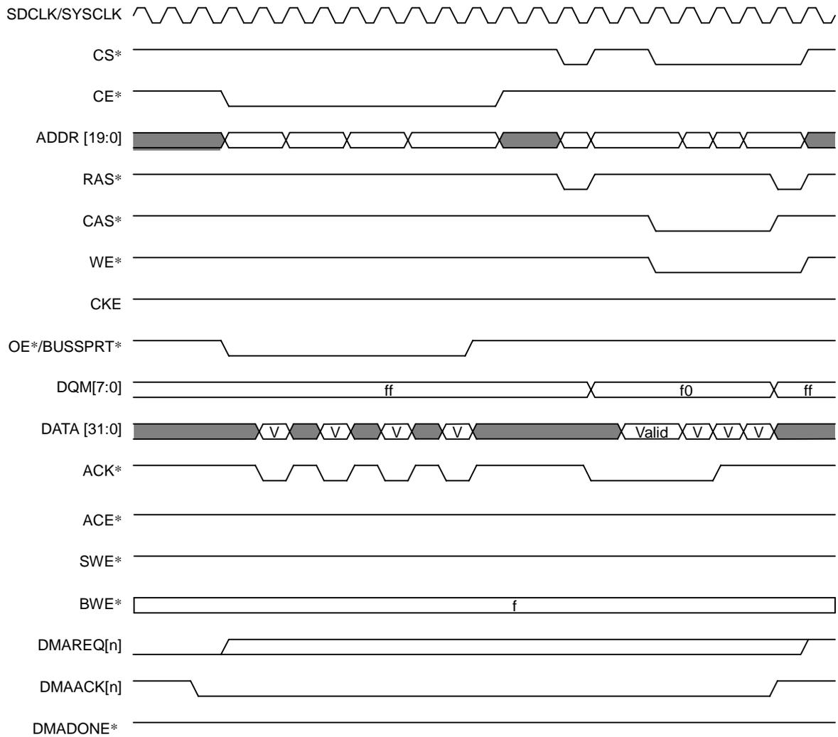
Figure 8.5.18 Dual Address Transfer from External I/O Device to SDRAM
