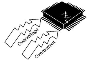
If the voltage or current on any pin exceeds the absolute maximum rating, the device's internal circuitry can become degraded. In the worst case, heat generated in internal circuitry can fuse wiring or cause the semiconductor chip to break down.
