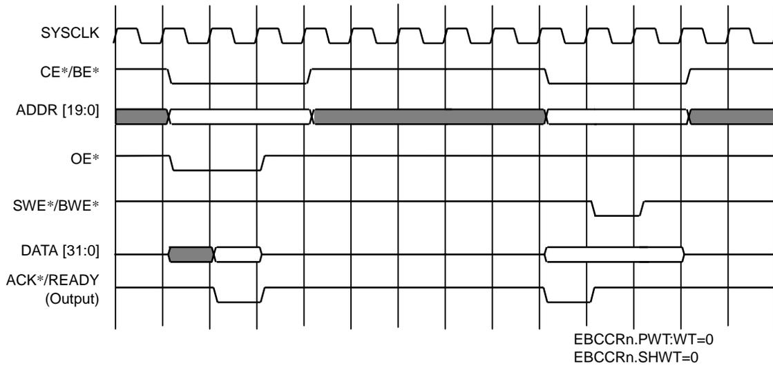
Figure 7.3.5 SWHT Disable (Normal Mode, Single Read/Write Cycle)
