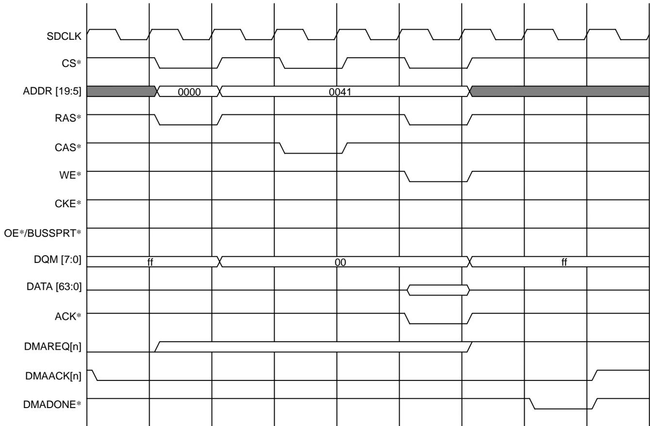
Figure 8.5.13 Single Address Single Transfer from Memory to I/O
