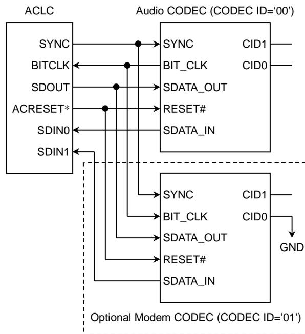
Figure 14.3.1 Stereo Audio and Optional Modem Connection Diagram
