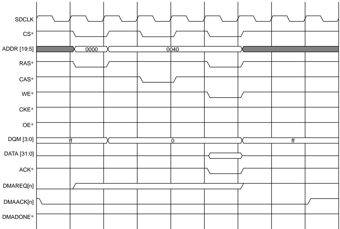
Figure 8.5.11 Single Address Single Transfer from Memory to I/O
