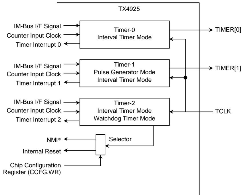
Figure 12.2.1 Connecting Timer Module Inside the TX4925
