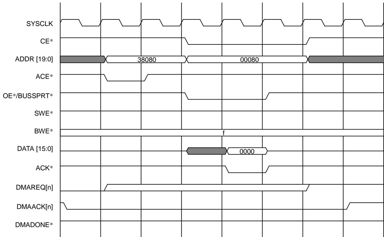
Figure 8.5.7 Single Address Single Transfer from Memory to I/O
