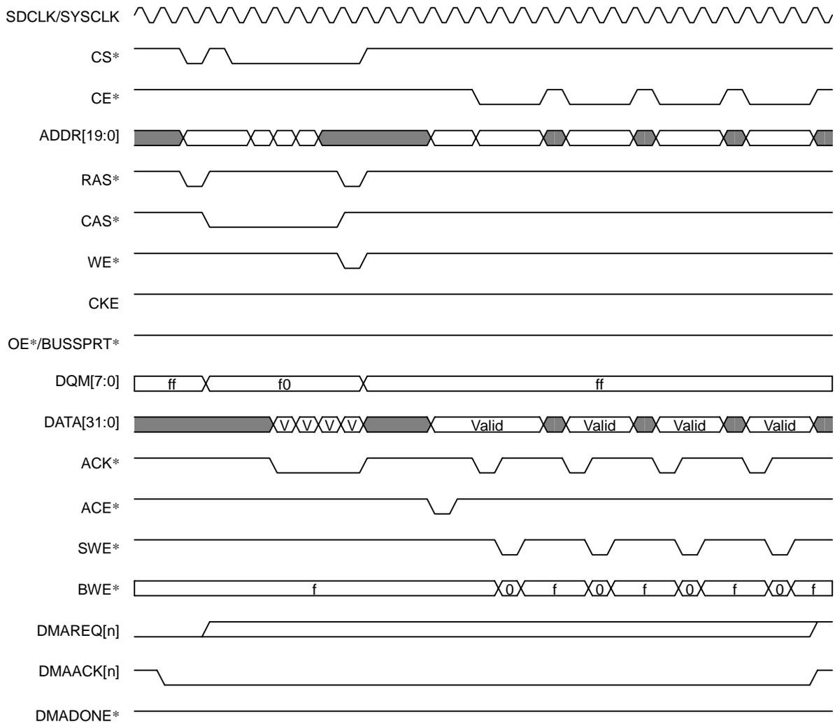
Figure 8.5.21 Dual Address Transfer from SDRAM to External I/O Device
