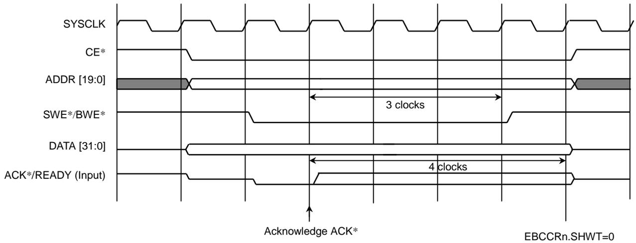
Figure 7.3.11 ACK\* Input Timing (Single Write Cycle)
