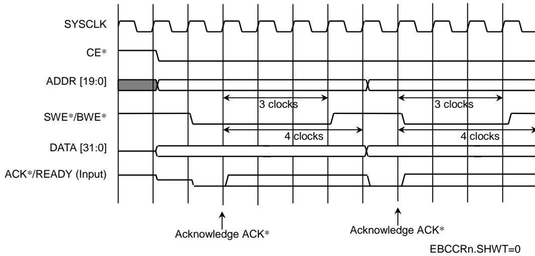
Figure 7.3.13 ACK\* Input Timing (Burst Write Cycle)
