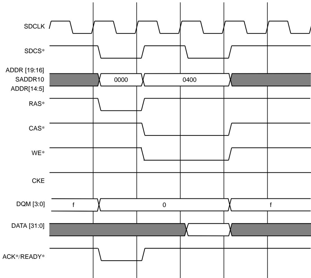
Figure 9.5.3 One-Word Single Write ( $t_{RCD} = 2$ ,  $t_{DA} = 0$ , 32-bit Bus)
