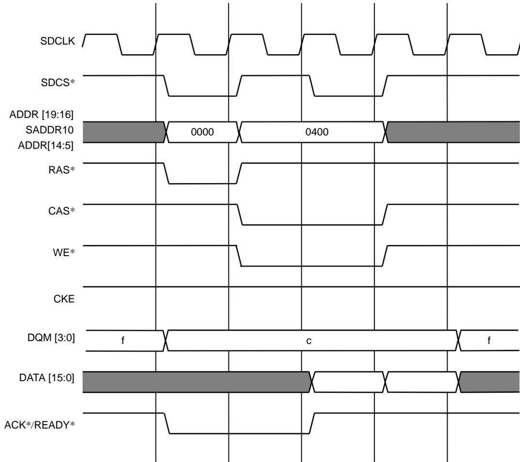
Figure 9.5.10 One-Word Single Write ( $t_{RCD} = 2$ ,  $t_{DA} = 0$ , 16-bit Bus)
