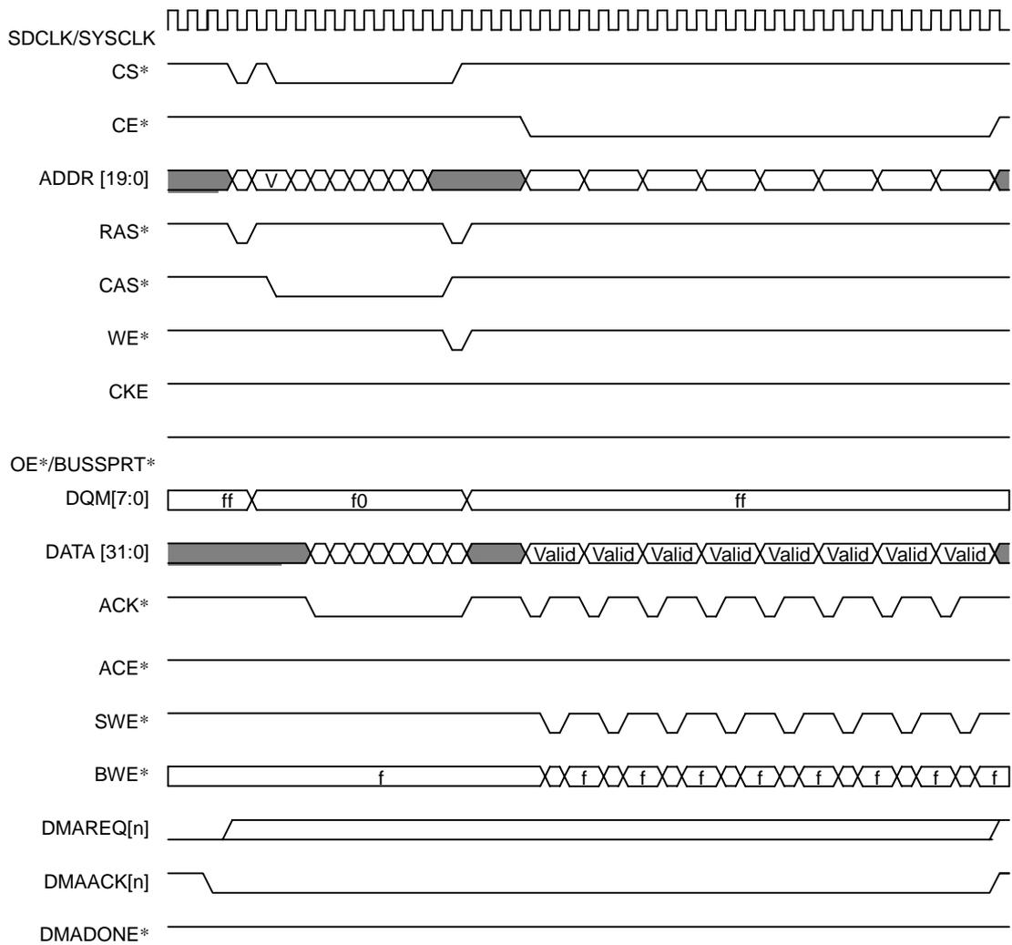
Figure 8.5.19 Dual Address Transfer from SDRAM to External I/O Device
