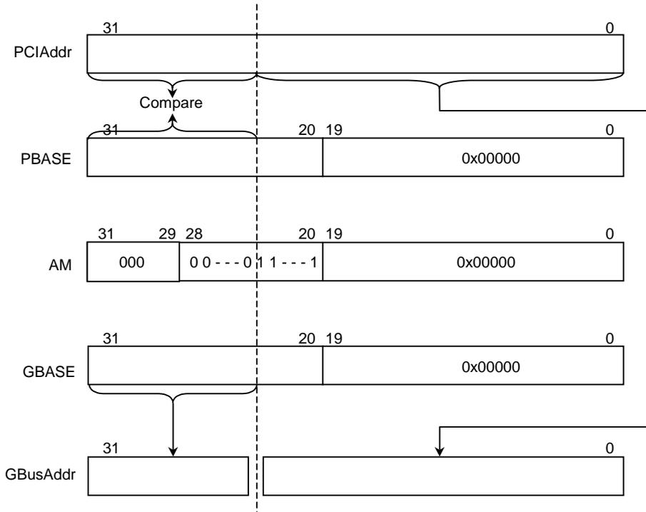
Figure 10.3.6 Memory Address Conversion for Target (PCI Bus → G-Bus Address Conversion)
