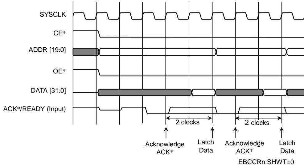
Figure 7.3.12 ACK\* Input Timing (Burst Read Cycle)
