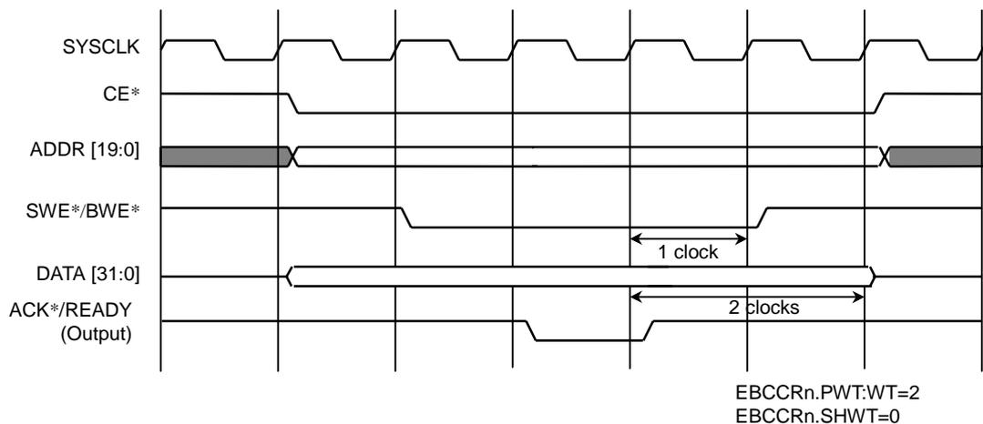
Figure 7.3.8 ACK\* Output Timing (Single Write Cycle)
