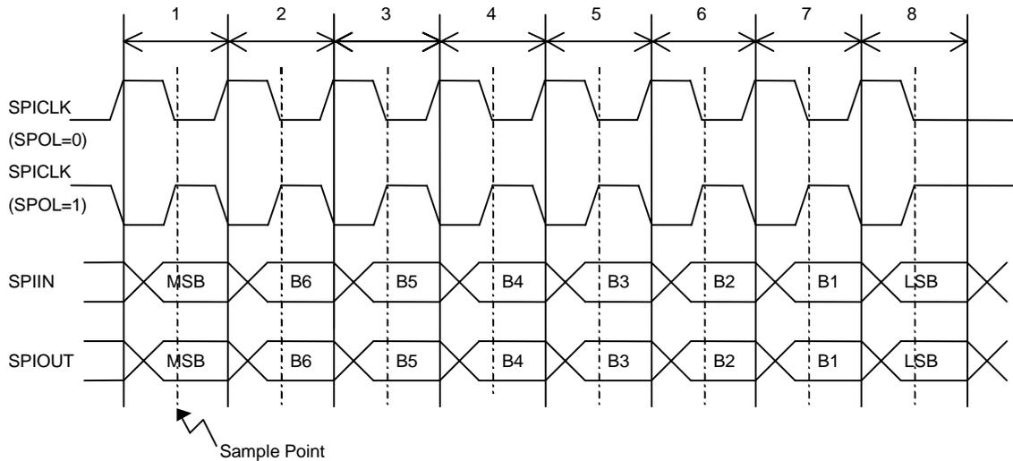
Figure 17.3.2 Transfer format when SPHA is "1".
