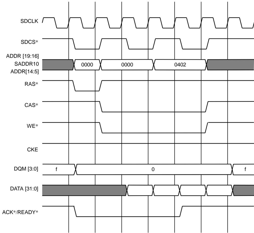
Figure 9.5.6 Four-Word Burst Write ( $t_{RCD} = 2$ ,  $t_{DA} = 0$ , 32-bit Bus)
