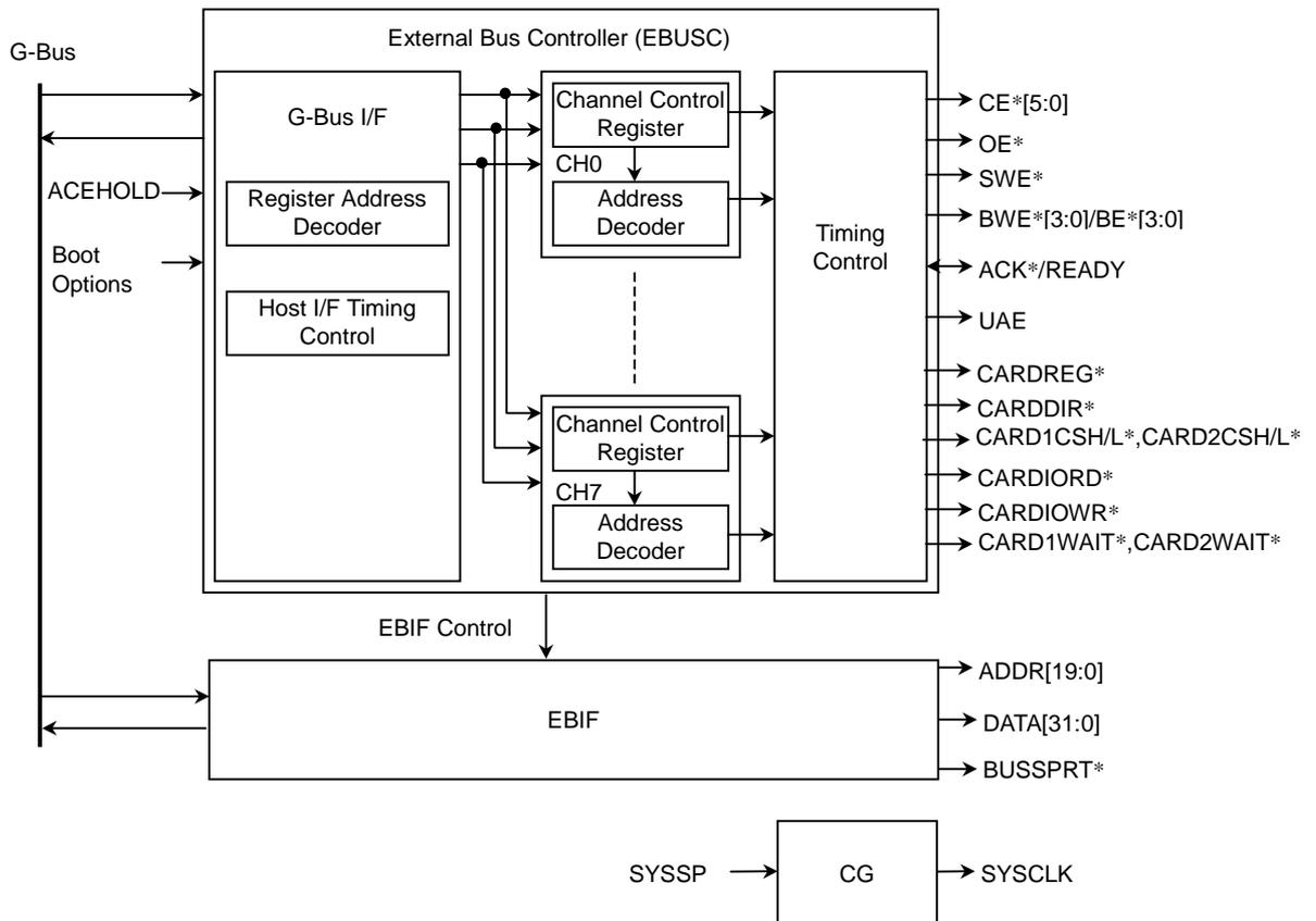
Figure 7.2.1 Block Diagram of External Bus Controller
