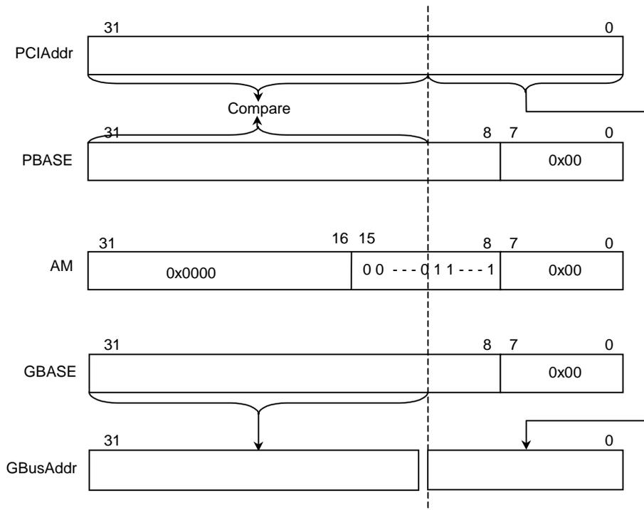
Figure 10.3.7 I/O Address Conversion for Target (PCI Bus → G-Bus Address Conversion)
