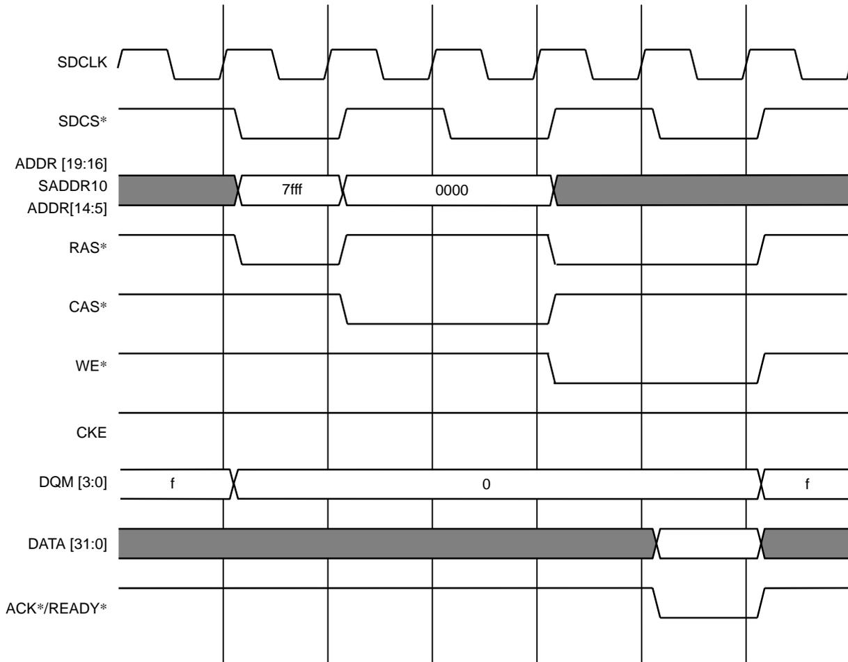
Figure 9.5.1 Single Read ( $t_{RCD} = 2$ ,  $t_{CASL} = 2$ ,  $t_{DA} = 0$ , 32-bit Bus)
