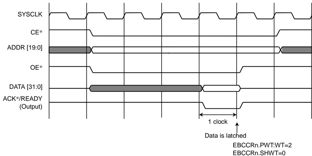
Figure 7.3.7 ACK\* Output Timing (Single Read Cycle)
