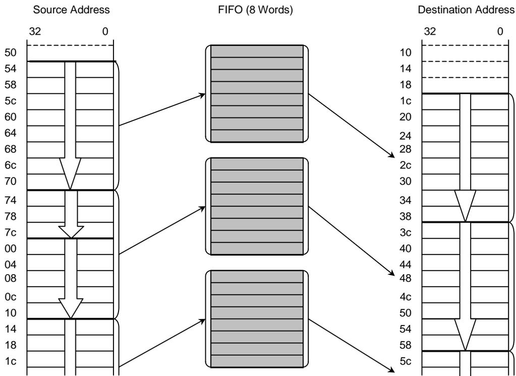
Figure 8.3.3 Dual Address Burst Transfer (DMCCRn.USEXFSZ = 1)
