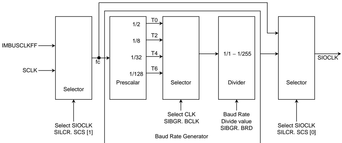
Figure 11.3.2 Baud Rate Generator and SIOCLK Generator
