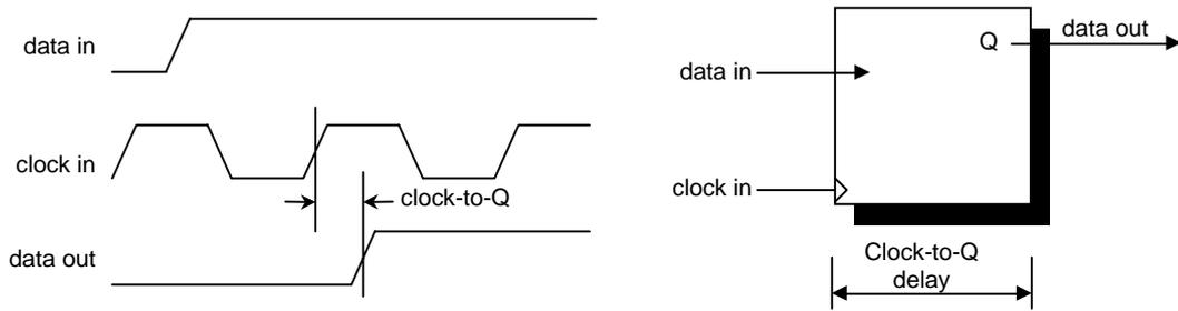
Figure 4.1.2 Clock-to-Q Delay
