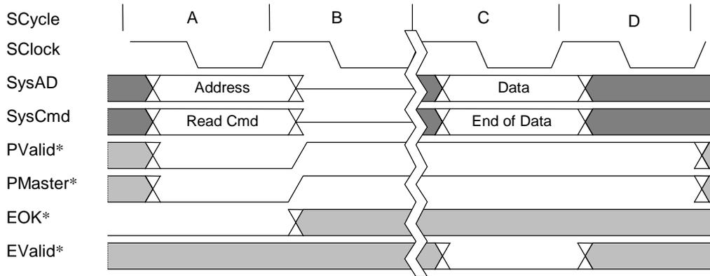
Figure 6.3.12 Sample Cycle with Assertion of *EReq*
