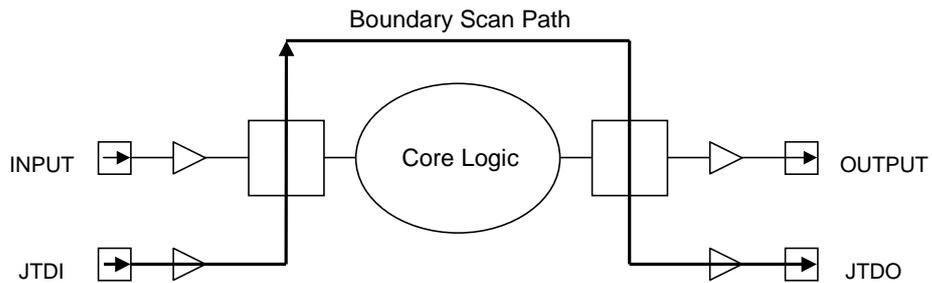
Figure 7.4.3 Test Data Flow While PRELOAD is Selected
