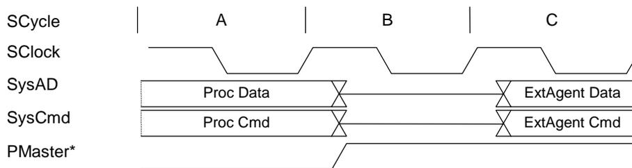
Figure 6.3.4 Sample Cycle with **PMaster\*** Asserted, Then Deasserted
