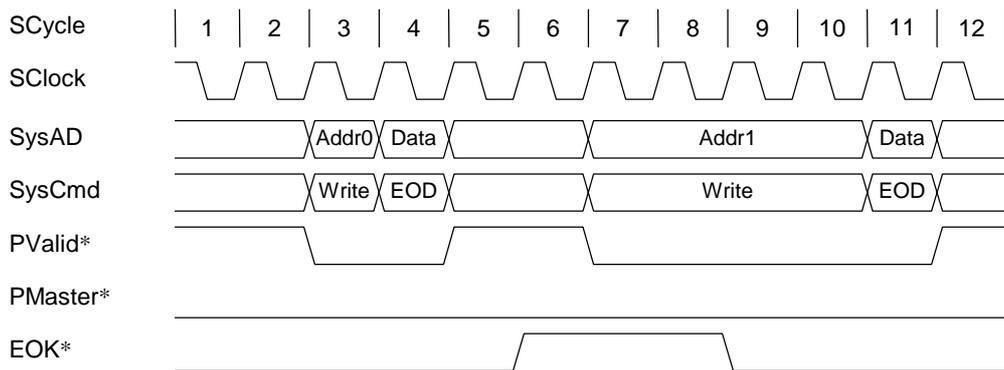
Figure 6.3.24 Two Processor Write Requests, Second Write Delayed
