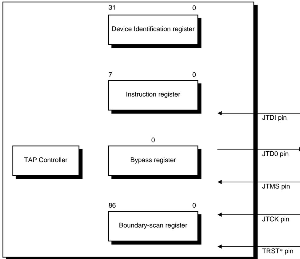
Figure 7.2.1 JTAG Interface Signals and Registers
