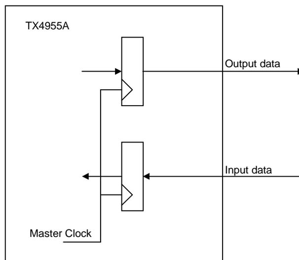
Figure 6.2.4 Operation of the System Interface Between Registers
