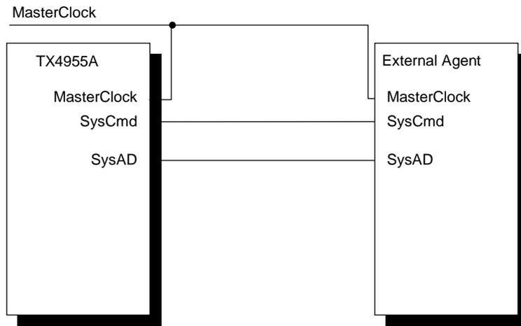
Figure 4.3.1 The TX4955A Processor Phase-Locked System
