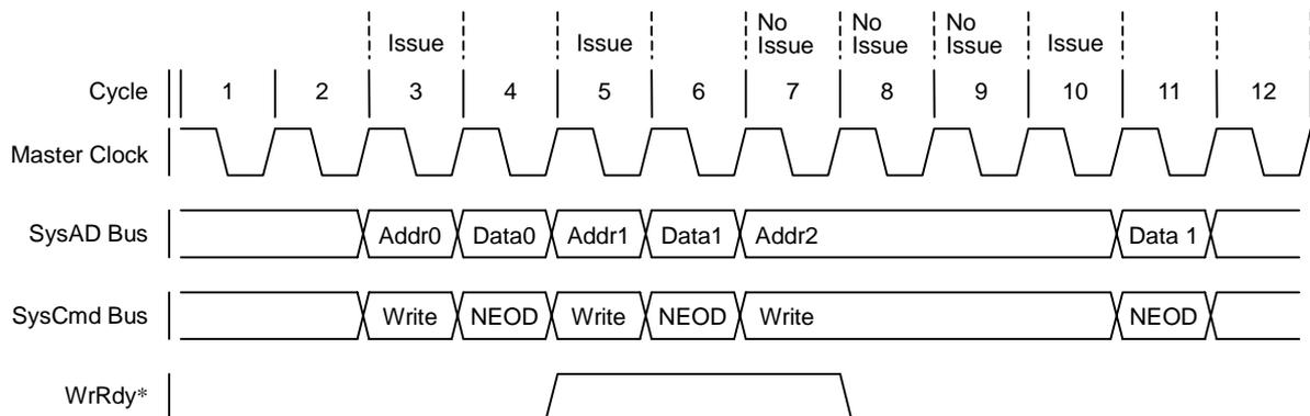
Figure 6.2.16 Pipeline Write Protocol
