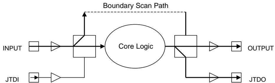
Figure 7.4.2 Test Data Flow While SAMPLE is Selected
