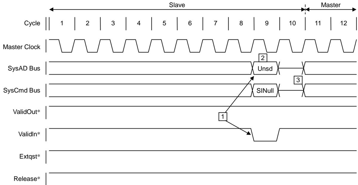
Figure 6.2.20 System Interface Release External Null Request
