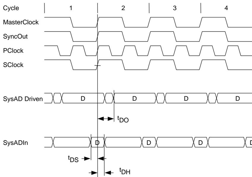
Figure 4.2.2 Processor Clock, PClock-to-SClock Divisor of 2
