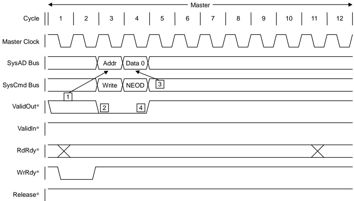
Figure 6.2.13 Processor Non-coherent Single Word Write Request Protocol
