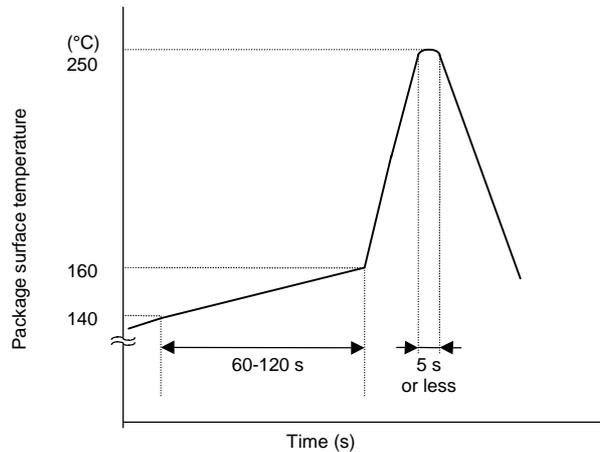
Figure 5 Sample temperature profile for solder flow
