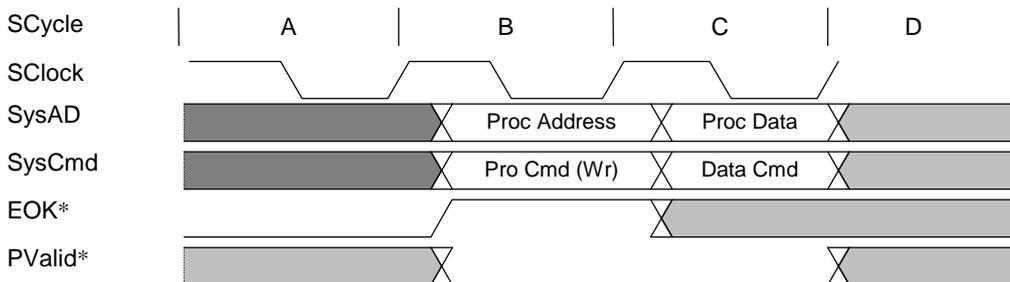
Figure 6.3.9 Sample Cycle with **EOK\*** Asserted, Then Deasserted
