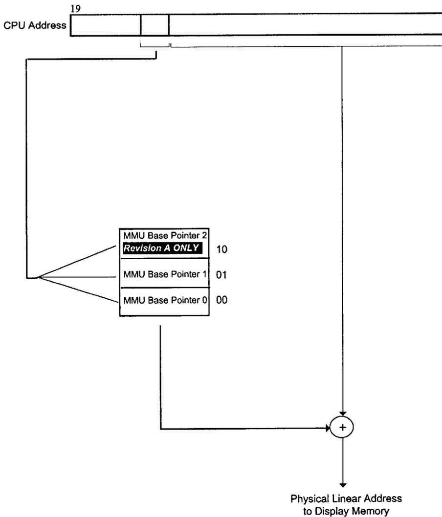
Figure 2.11.1-1 Three MMU Aperture Mapping
