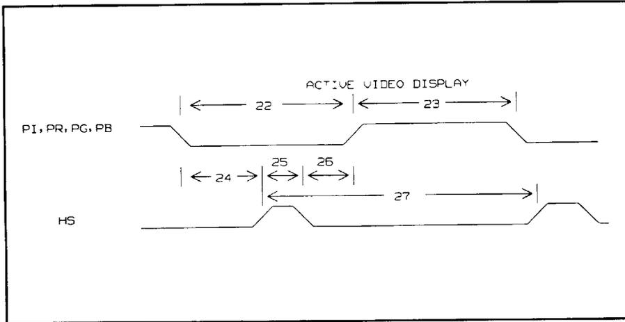
Figure 6.6.3-5 Display Horizontal Timing, 40/80 Column, no Border
