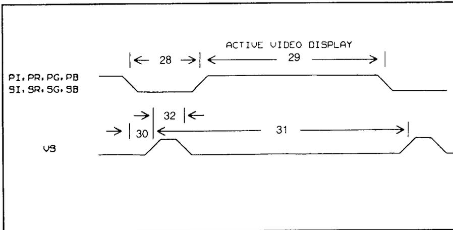
Figure 6.6.3-6 Display Vertical Sync Timing, 768 Lines
