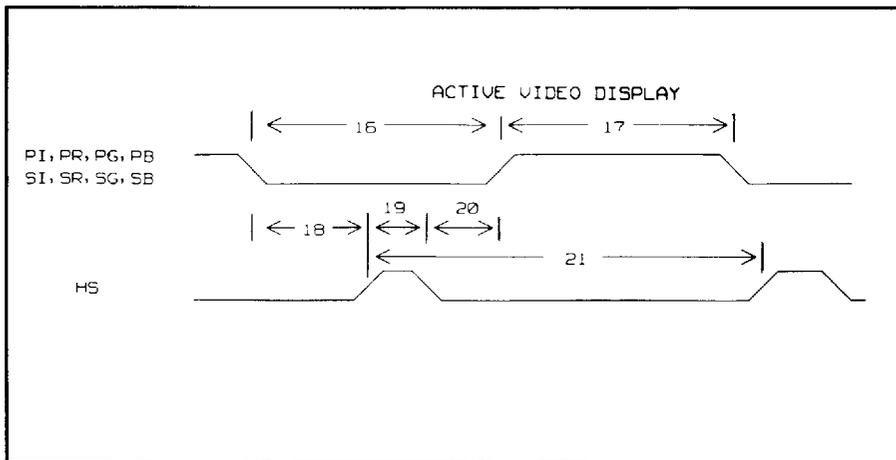
**Figure 6.6.3-4 Display Horizontal Timing, 80 Column with Border**
