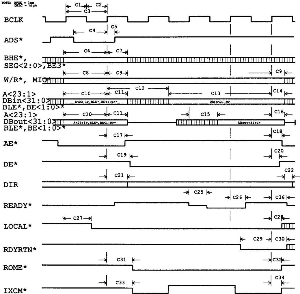
Figure 4.11-1 Local Bus Read/Write Timing
