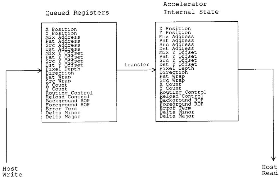
**Figure 2.12-2 ET4000/W32p Queued Registers and ACL Internal State**
