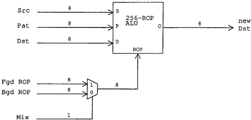
**Figure 2.12-1 ET4000/W32p Graphics Accelerator Data Path**
