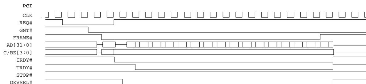
**Figure 41: Multiple PCI Read Transactions During DMA Operation**
