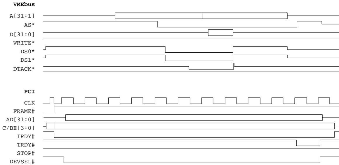
**Figure 30: Several Coupled Read Cycles - Universe II as VME Master**
