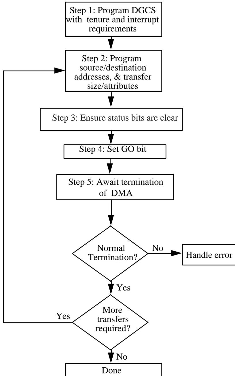
In Step 1, the DGCS register is set up
