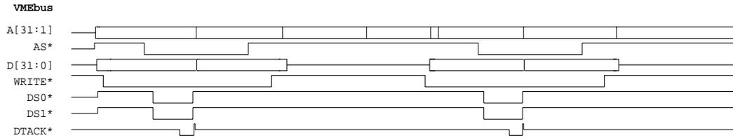
**Figure 33: BLT Decoupled Write - Universe II as VME Master**
