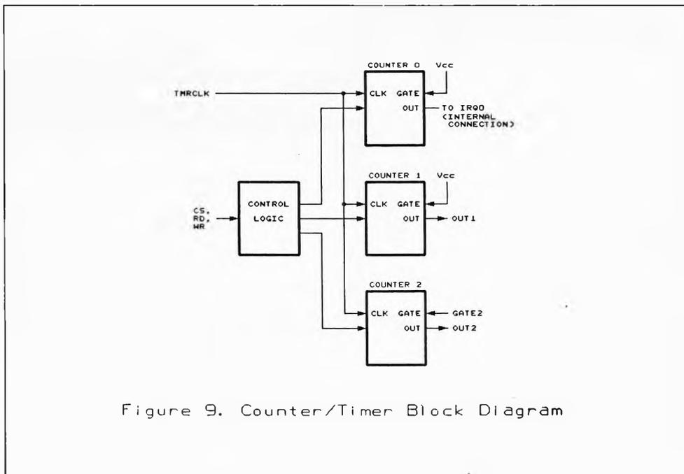
Figure 9. Counter/Timer Block Diagram
