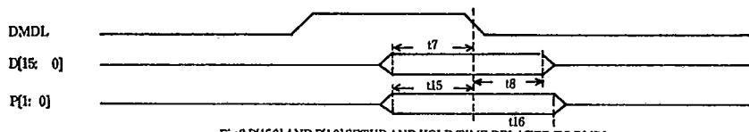
Fig 3 D[15:0] AND P[1:0] SETUP AND HOLD TIME RELATED TO DMDL
