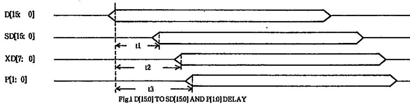
Fig 1 D[15:0] TO SD[15:0] AND P[1:0] DELAY
