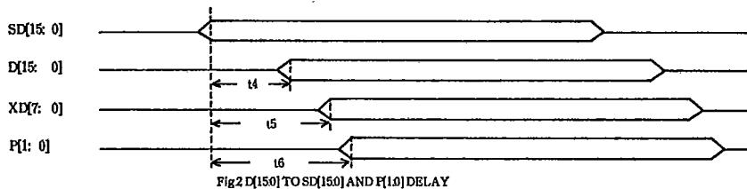
Fig 2 D[15:0] TO SD[15:0] AND P[1:0] DELAY
