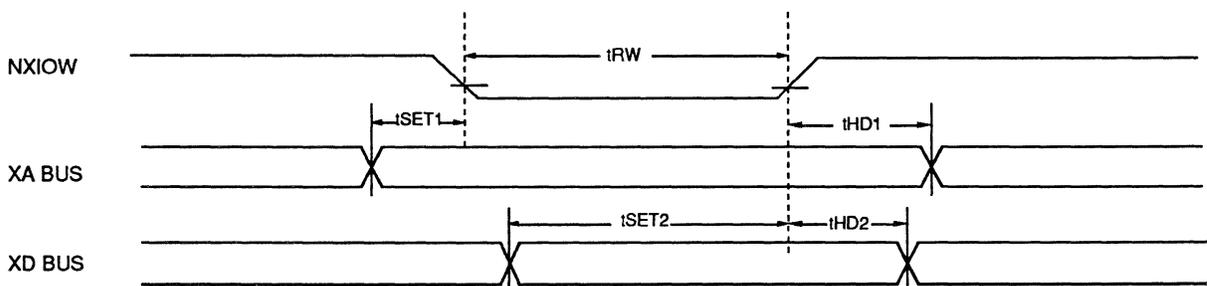
Fig. 5. WRITE TIMING
