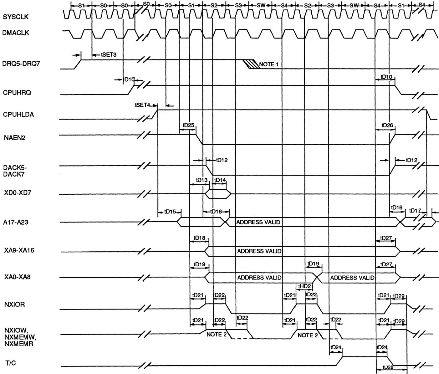
Figure 10. 16 BIT DMA TIMING
