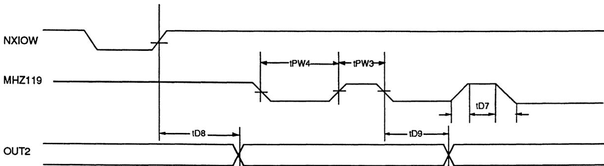
Fig. 8. TIMER/COUNTER TIMING
