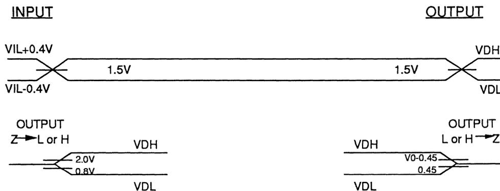
A.C. Testing: All A.C. Parameters tested as per test circuits. Input RISE and FALL times are driven at  $1ns/V$ .
