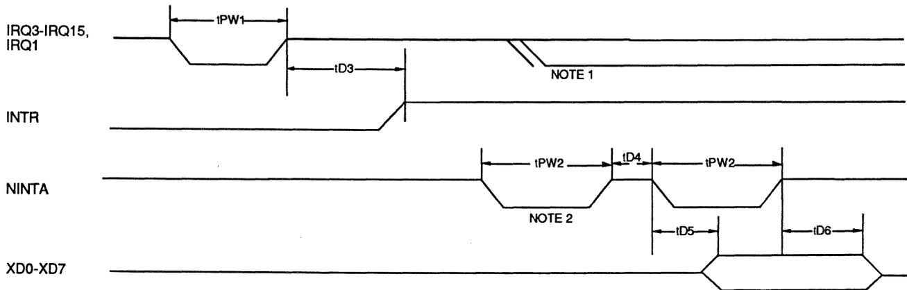
Fig. 7. INTERRUPT TIMING
