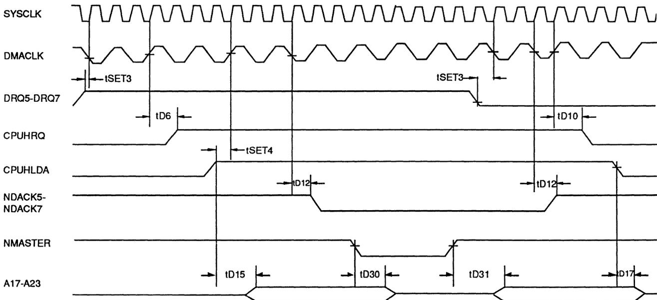
Figure 12. NMASTER TIMING
