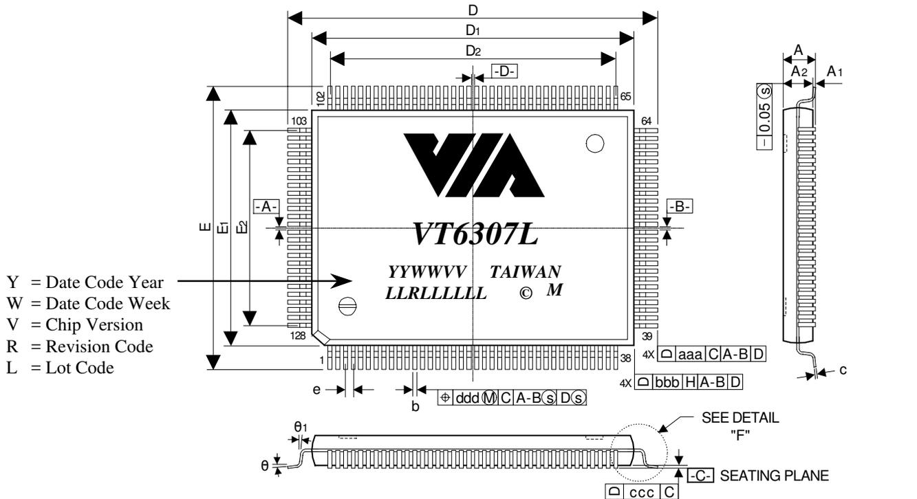
CONTROL DIMENSIONS ARE IN MILLIMETERS.
