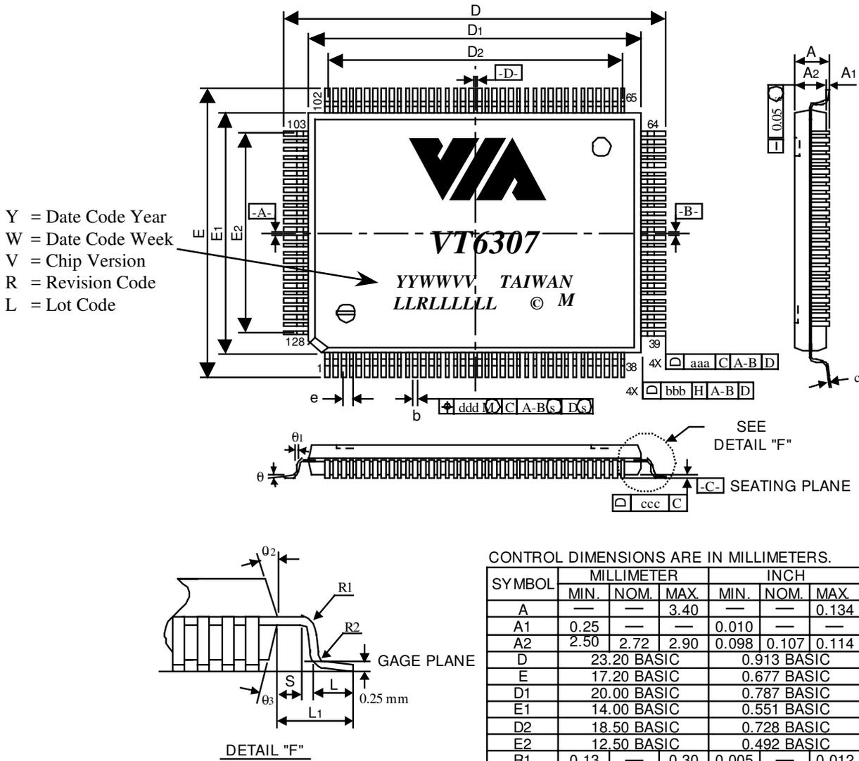
CONTROL DIMENSIONS ARE IN MILLIMETERS.
