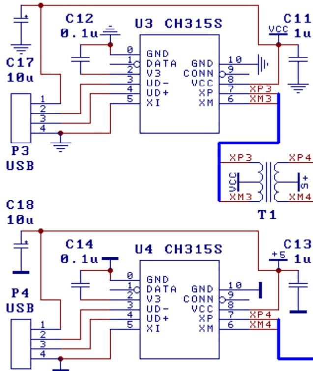
The figure above is a simplified version of the USB isolation extension line realized by two sets of CH315S.
