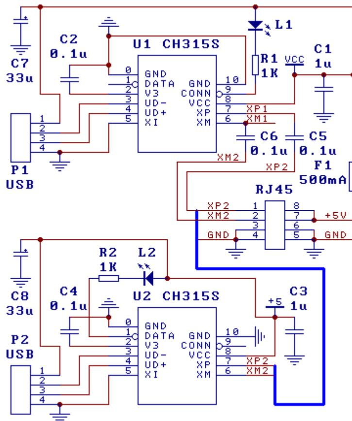
The figure above is a capacitive coupling USB extension line realized by two sets of CH315S.
