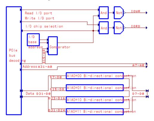
The figure above is the main structure of CH367. After CH367 decodes various signals of PCIE bus, it generates internal data buses D31~D0, internal address buses A31~A0, read I/O port signal and write I/O port signal, etc. The transmission direction of each signal has been marked in the figure.
