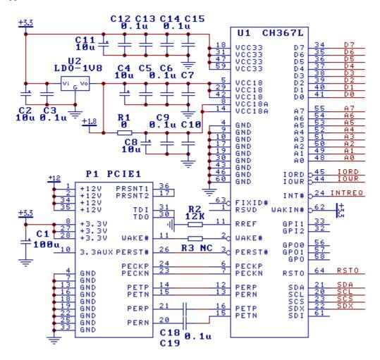
If the wake-up function is not used, it can remove R3 and make WAKE# pin suspended, but WAKIN# pin is
