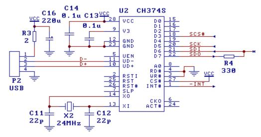
If RD# and WR# pins of CH374 are at the low level (grounded) and the CS# pin is at the high level (connected to a positive power source), then CH374 will work in SPI serial mode. In the SPI serial port mode, CH374 only needs to be connected to 5 signal lines with DSP/MCU: SCS# pin, SCK pin, SDI pin, SDO pin, and INT# pin. Other pins can be suspended.
