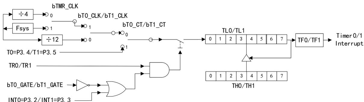
Mode3: Timer0 is divided into 2 separate 8-bit timer/counter, and borrowed TR1 of Timer1. Timer1 substitutes the borrowed TR1 control bit by whether starting mode3. Timer1 stops when it gets into mode3.
