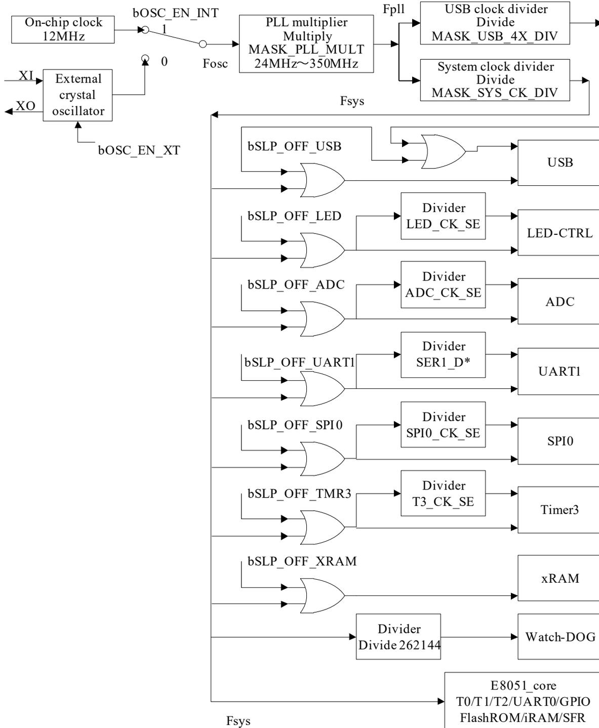
Select one of internal clock or external clock as source clock, then generate high frequency Fpll after frequency multiplier PLL. Generate system clock Fsys and USB module clock Fusb4x after 2 frequency dividers. The system clock Fsys is provided to different modules of CH558 directly or after clock gate, to reduce power dissipation, set sleep control register to close unused modules clocks.
