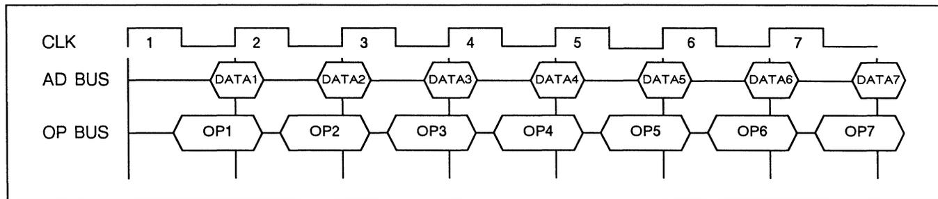
Figure 19. External I/O timing (for data transfers over the AD bus)
