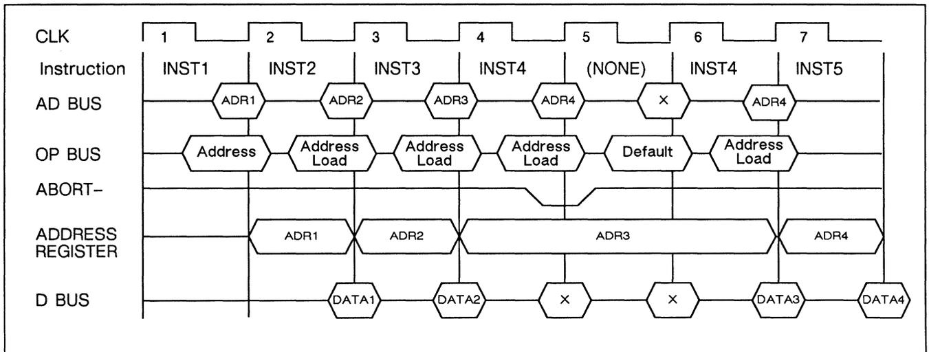
Figure 17. Data memory timing—loads. "ADDRESS REGISTER" is the external data address register
