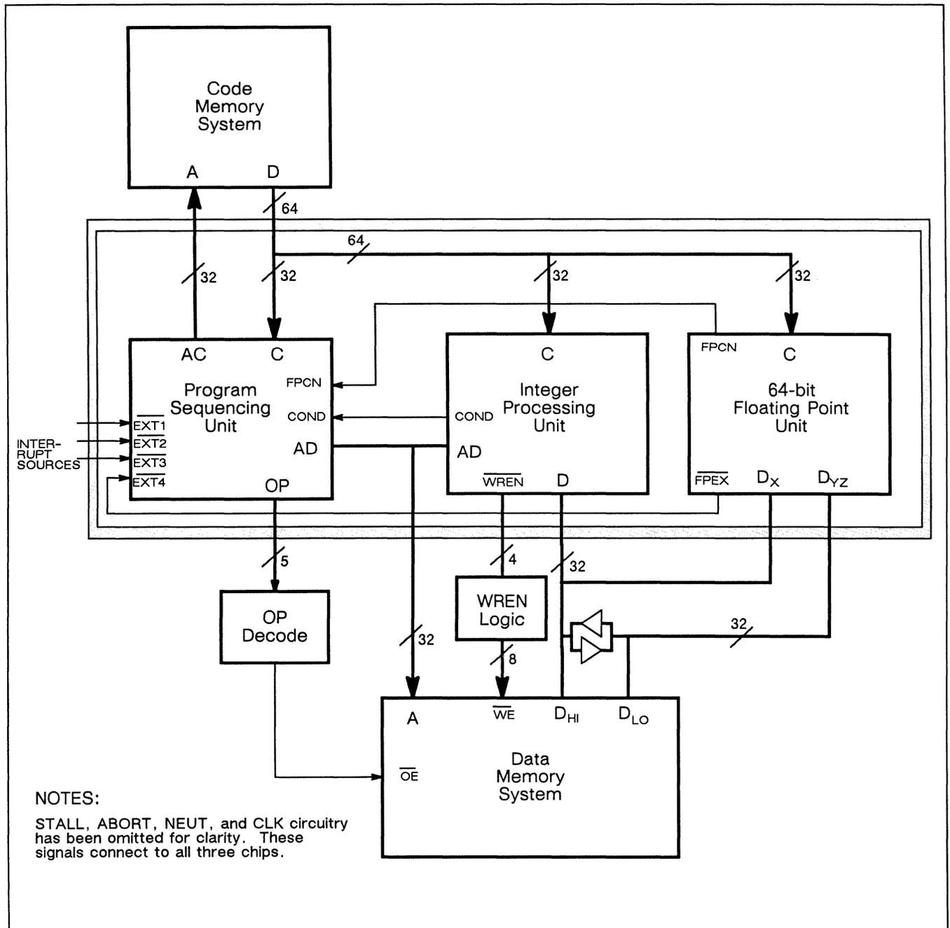
Figure 13. Block diagram of an XL-8364 system (64-bit FPU with a 64-bit data bus)
