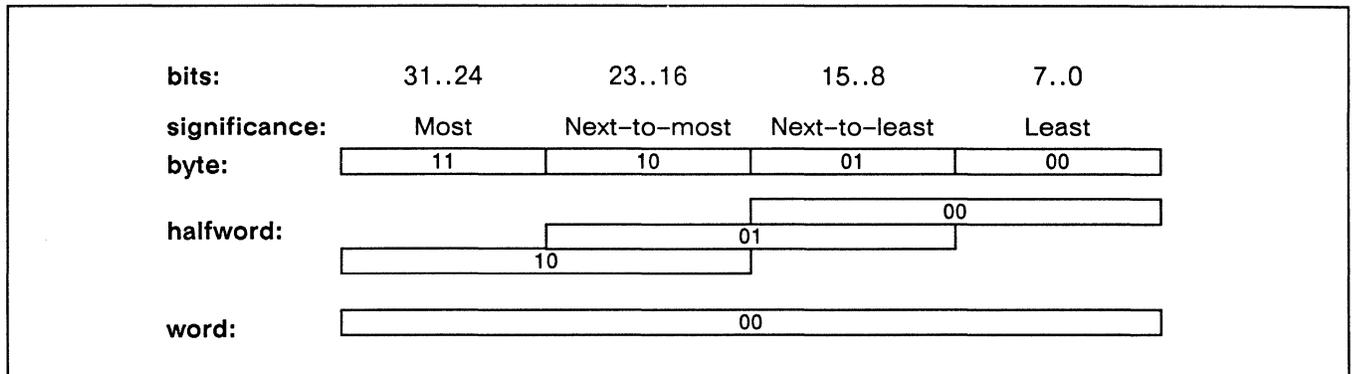
Figure 3. Data memory addressing and byte ordering
