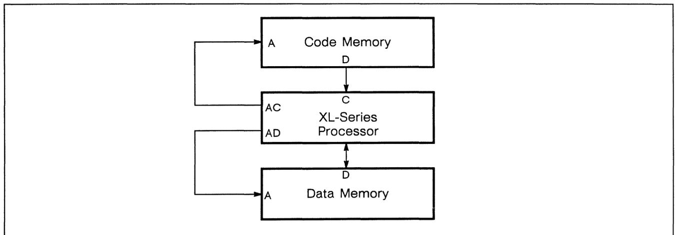
Figure 1. Simplified block diagram of an XL-series processor
