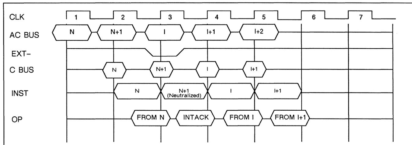
Figure 20. Interrupt sequence. ("INST" identifies which instruction is being executed.)
