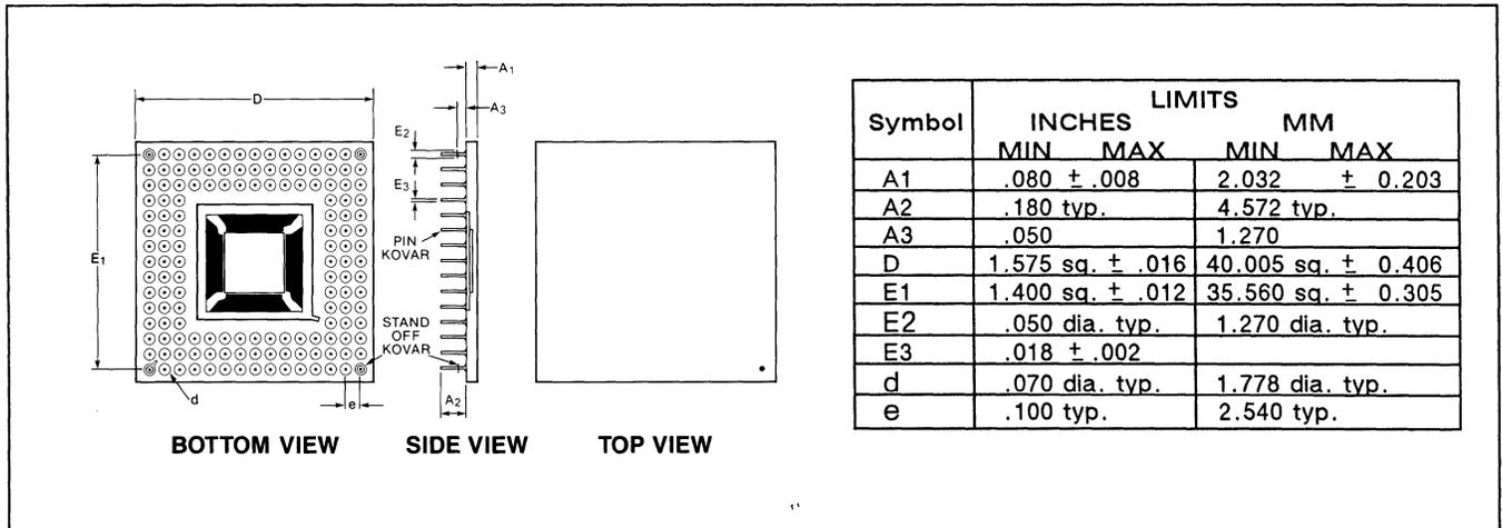
Figure 21. Physical dimensions for all XL-Series devices except the XL-8364 floating point unit
