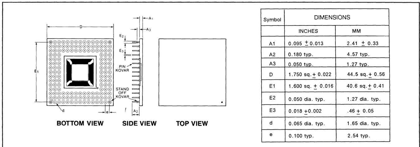
Figure 22. Physical dimensions for the XL-8364 floating point unit
