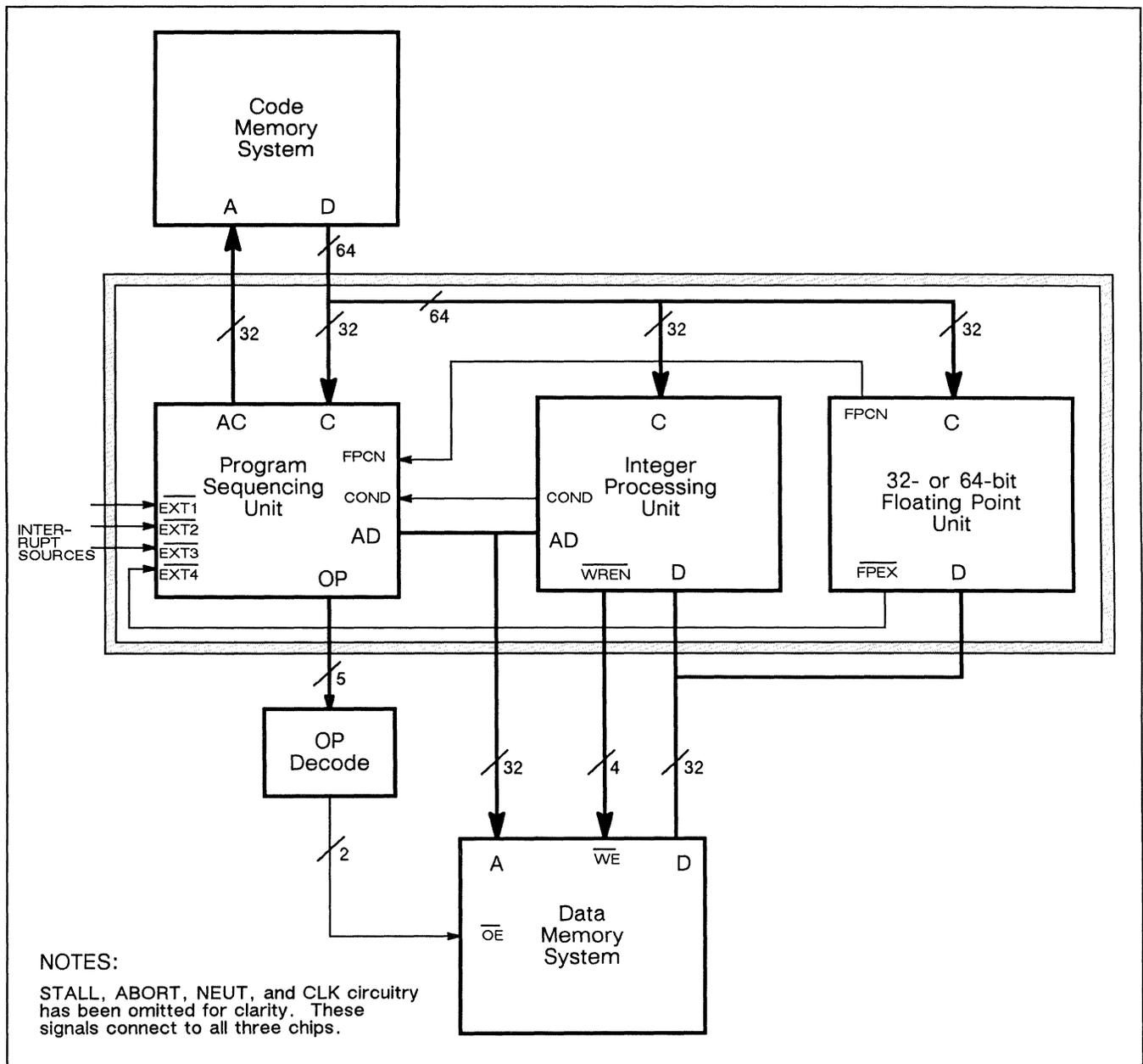
Figure 12. Block diagram of an XL-8032 (32-bit FPU) system or an XL-8164 (64-bit FPU, 32-bit bus) system.
