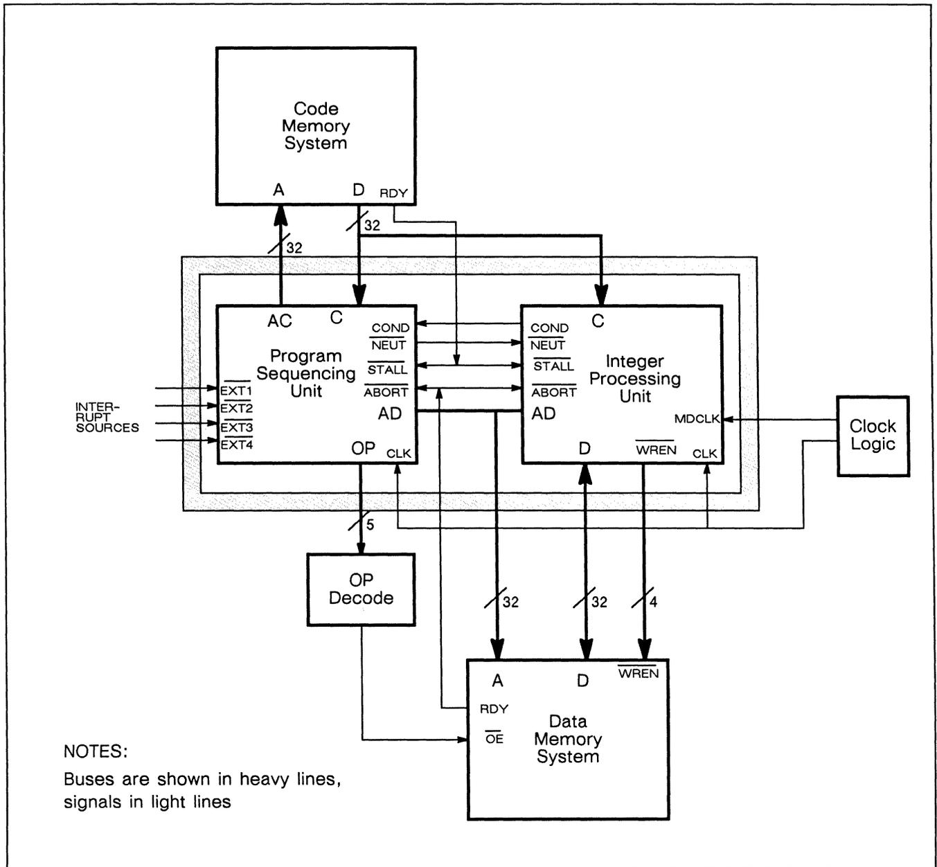
Figure 11. Block diagram of an XL-8000 system
