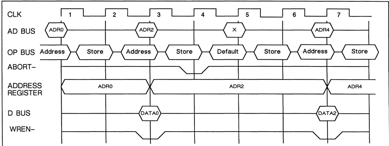
Figure 18. Data memory timing—stores. "ADDRESS REGISTER" is the external data address register
