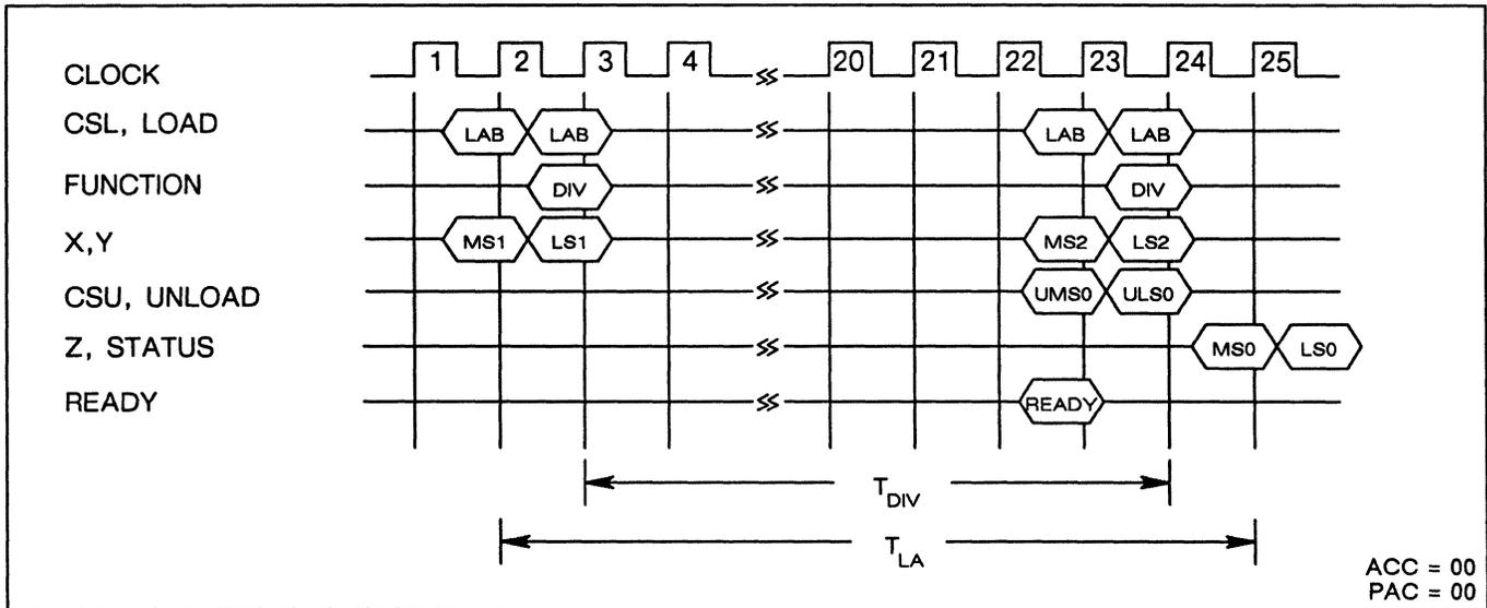
Figure 10. WTL 2264-50, -60 or -75 64-bit Divide Operation
