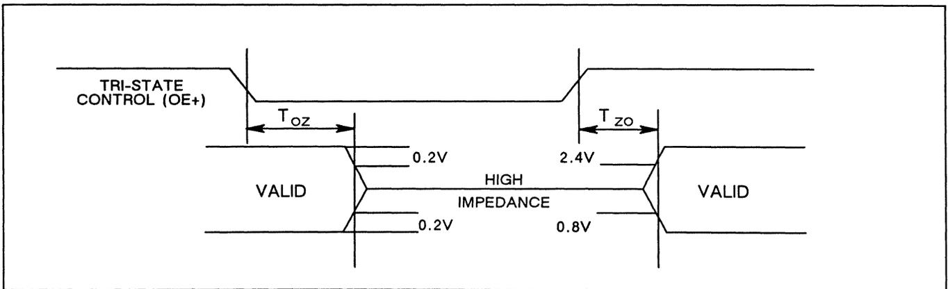
Figure 17. Tri-state Enable/Disable Timing Diagram
