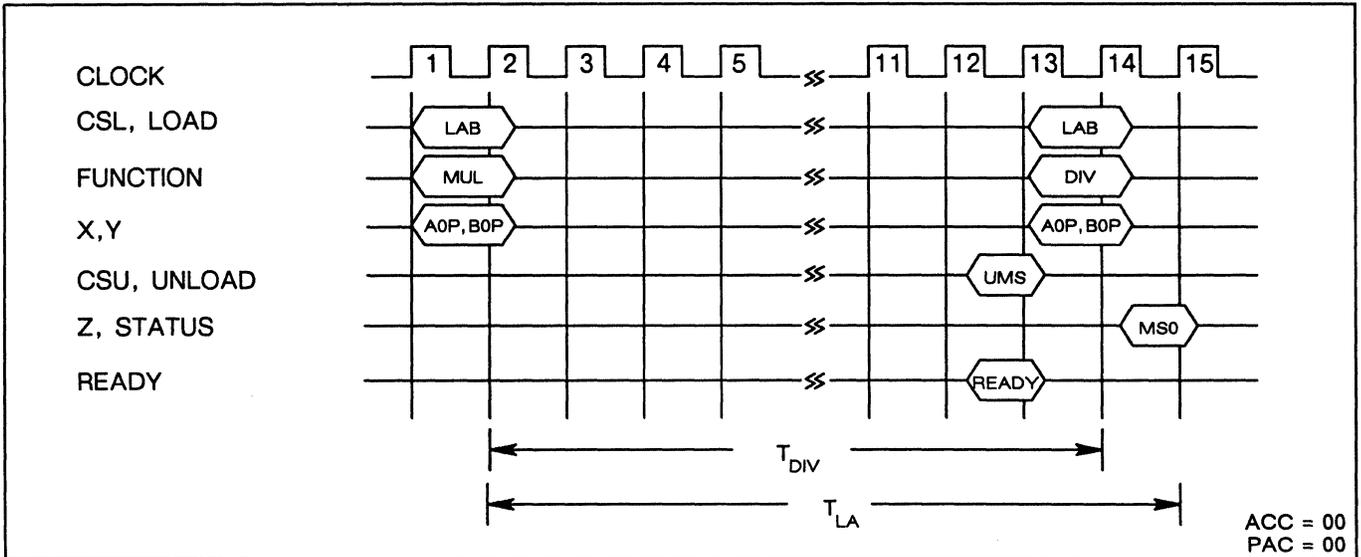
Figure 9. WTL 2264-50, -60 or -75 32-bit Divide Operation
