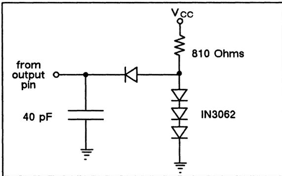
Figure 15. Normal Load Circuit for Delay Measurement
