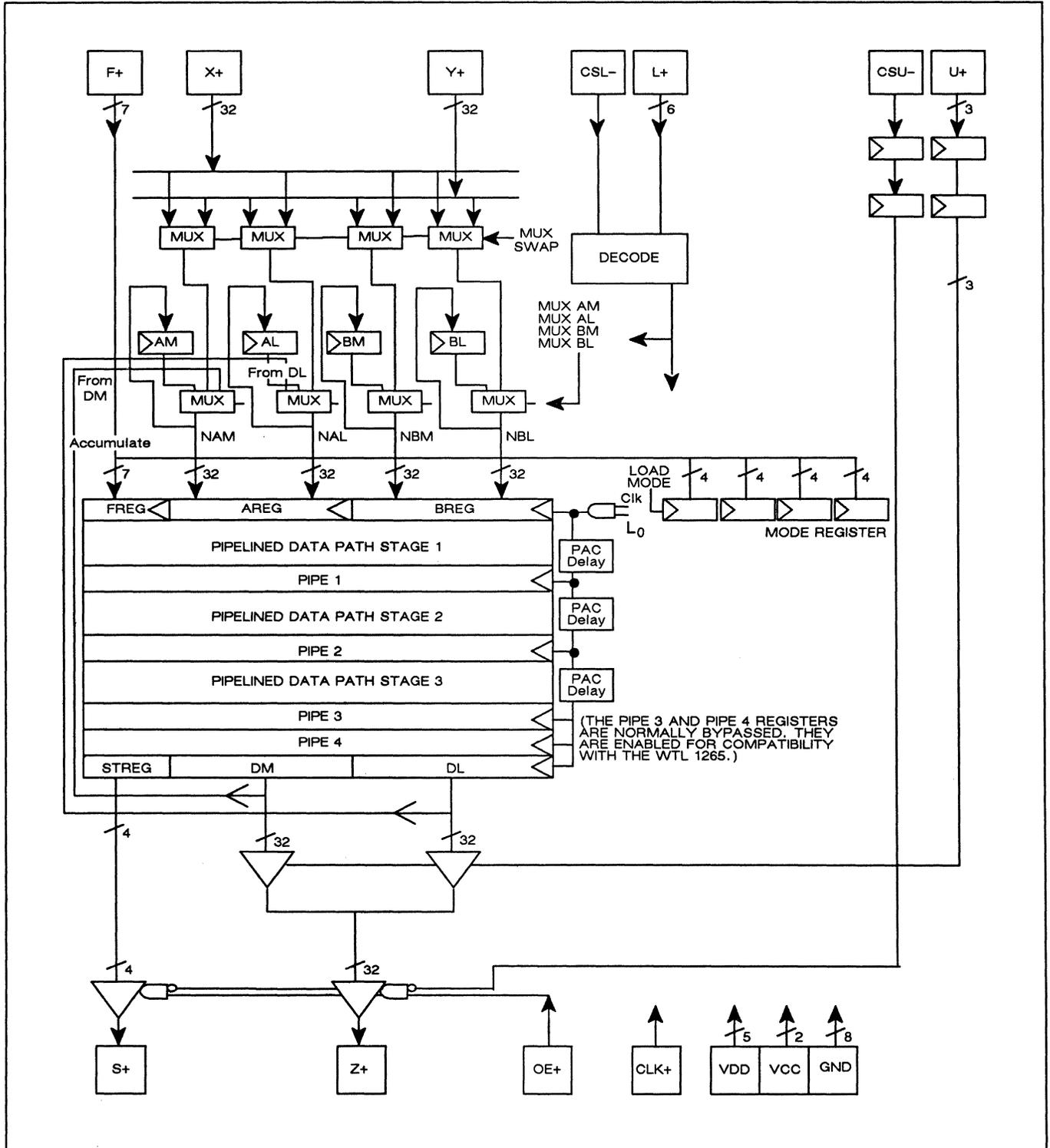
Figure 2. WTL 2265 Block Diagram
