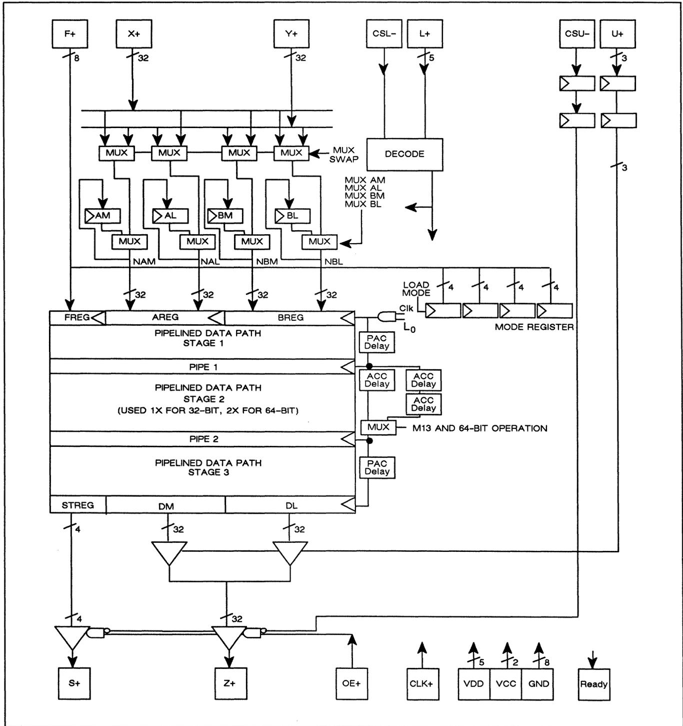
Figure 1. WTL 2264 Block Diagram
