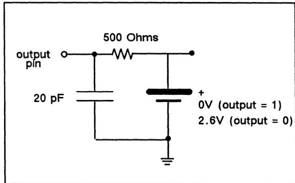
Figure 16. Tri-state Delay Load Circuit
