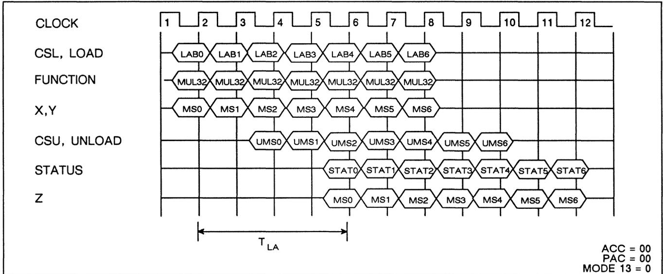
Figure 5. WTL 2264-50, -60 or -75 32-bit Pipelined Operation Timing
