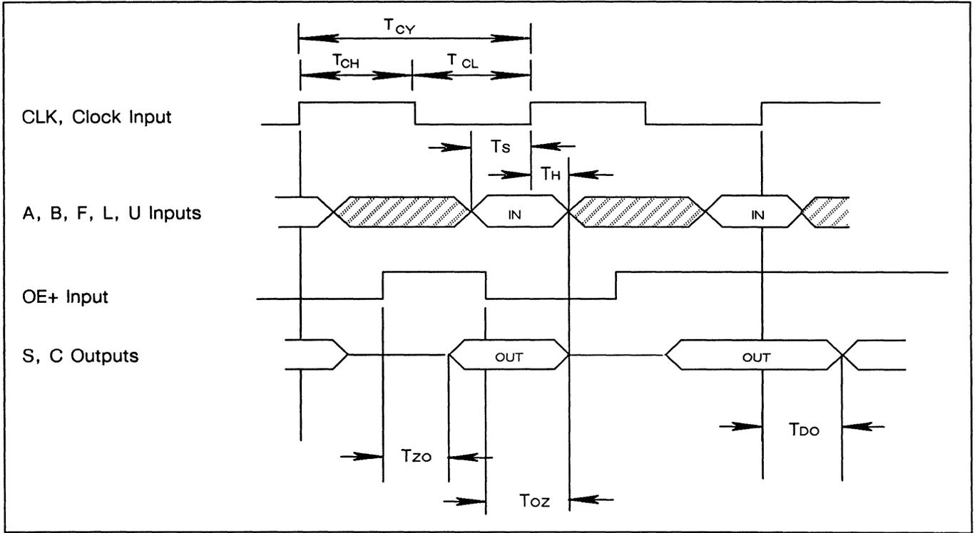
Figure 16. Input/Output Timing
