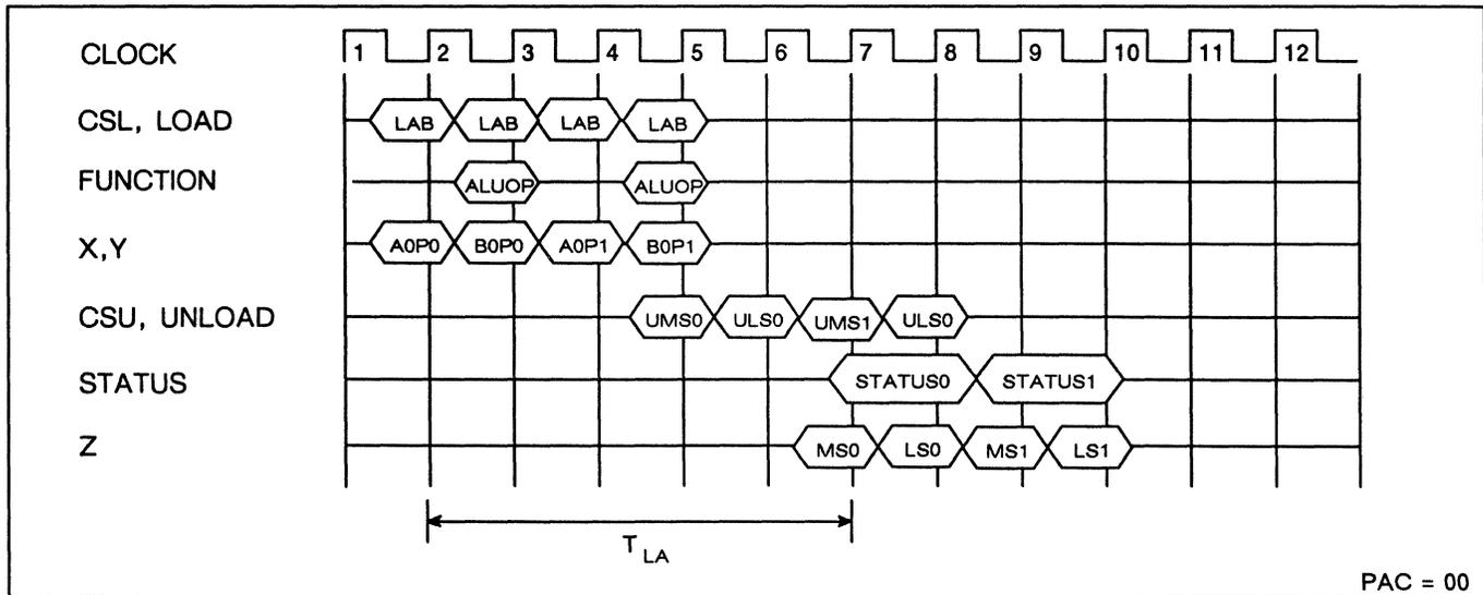
Figure 8. WTL 2265-50, -60 or -75 Pipelined ALU Operation Timing
