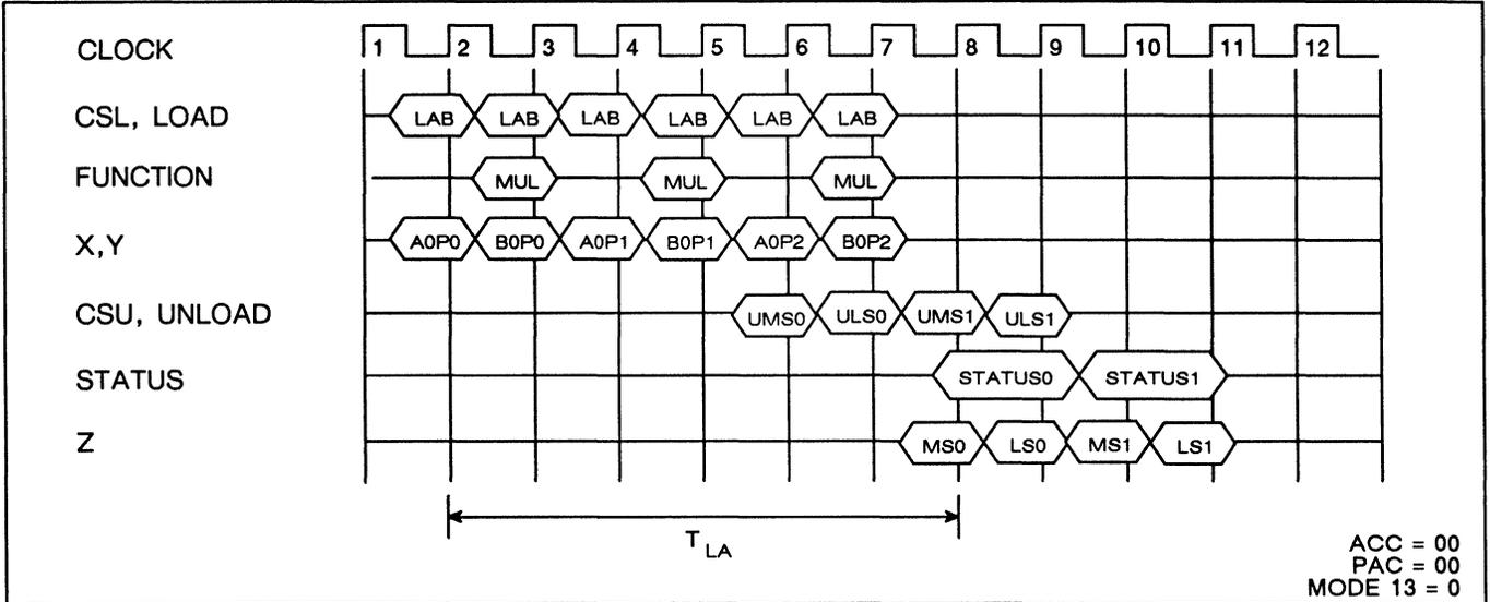
Figure 4. WTL 2264-50, -60 or -75 64-bit Pipelined Operation Timing
