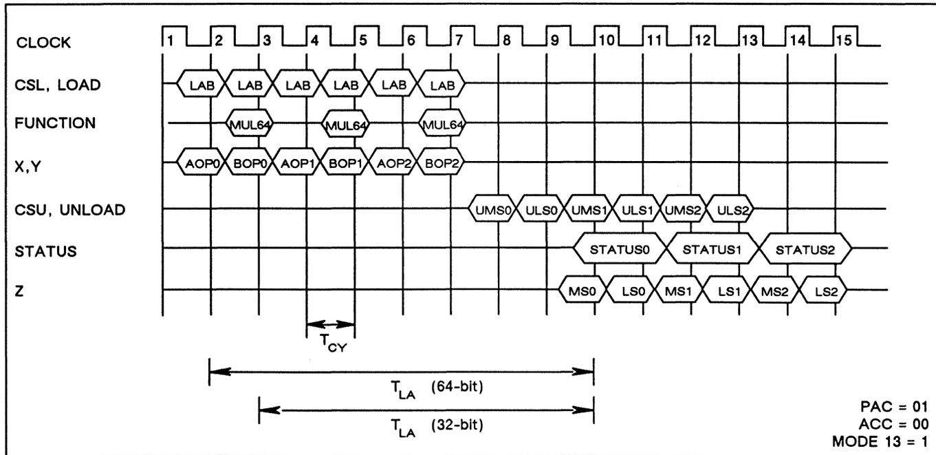
Figure 3. WTL 2264/2265-80 and -100 32- and 64-bit Pipelined Operation Timing
