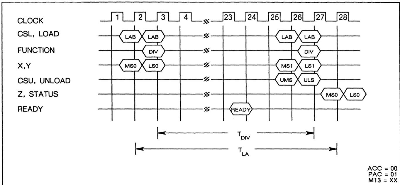
Figure 12. WTL 2264-80 or -100 64-bit Divide Operation
