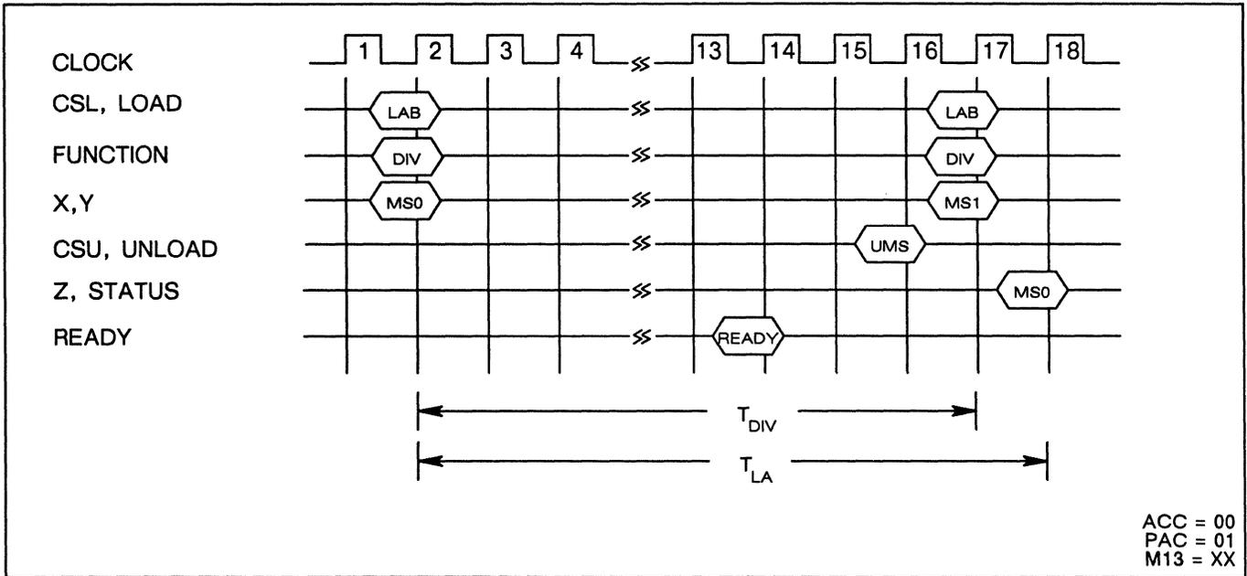
Figure 11. WTL 2264-80 or -100 32-bit Divide Operation
