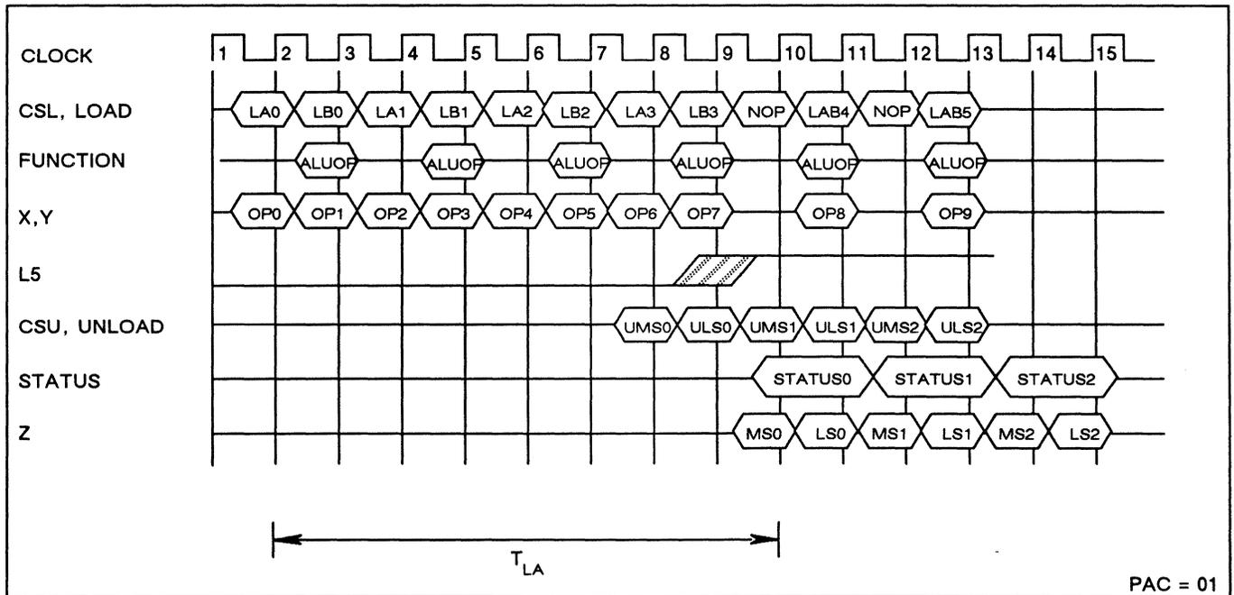
Figure 7. WTL 2265-80 or -100 Accumulate Timing
