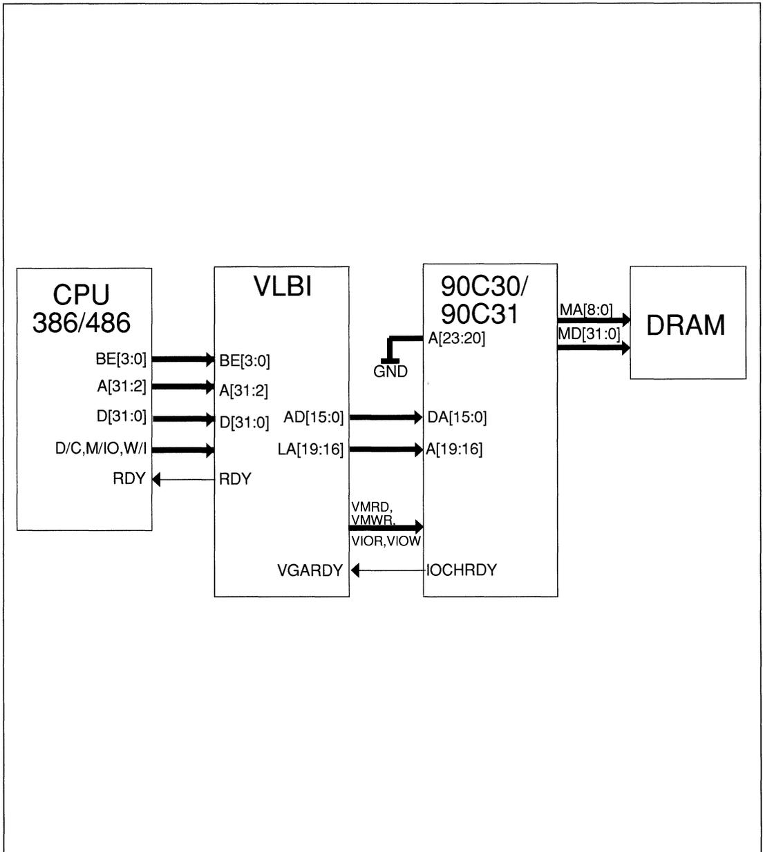
FIGURE B-1. VLBI INTERFACED TO WD90C30/WD90C31
