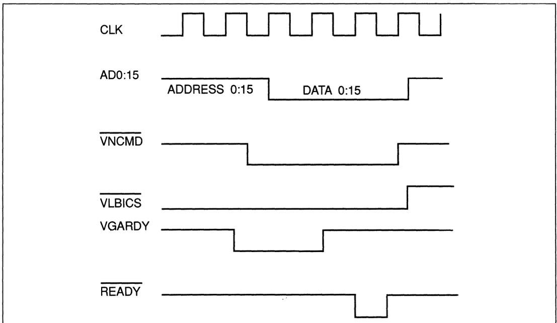
FIGURE 2-3. VLBI SYNCHRONOUS INTERFACE
