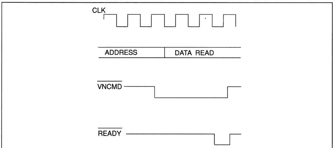
FIGURE 2-1. TYPICAL 16-BIT VGA READ CYCLE
