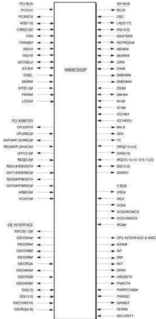
Figure 2-2. W83C553F Logic Symbol Diagram
