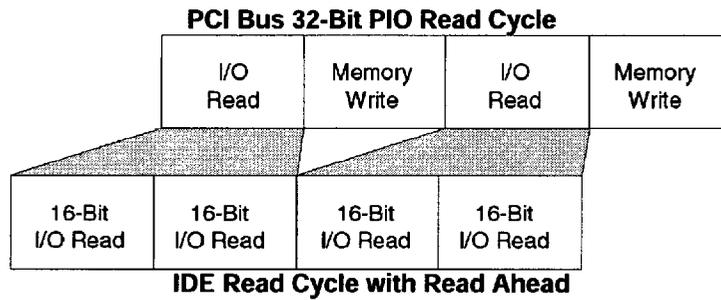
The two drawings shown above show the relationship between the PCI bus and the IDE interface.
