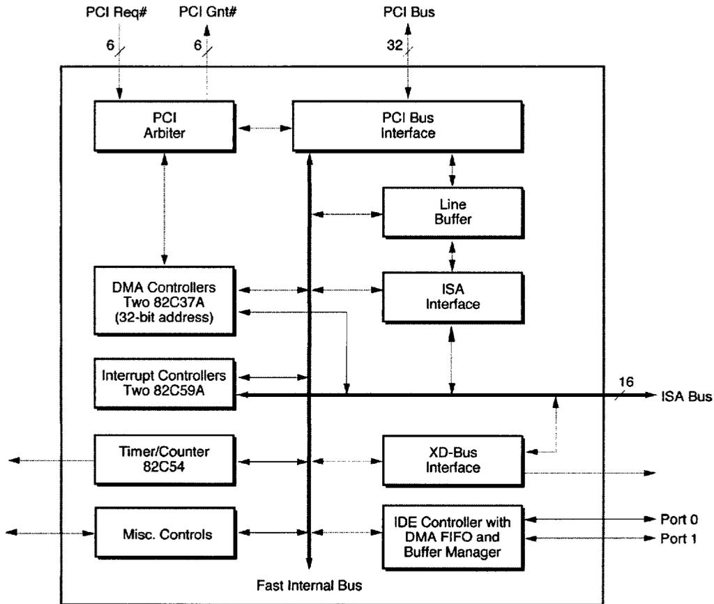
Figure 1-1. W83C553F Enhanced System I/O Controller Block Diagram
