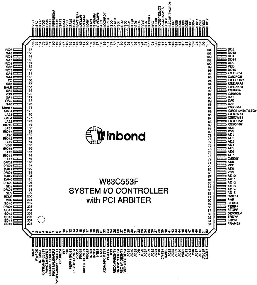
Figure 2-1. Pin Assignments for the W83C553F
