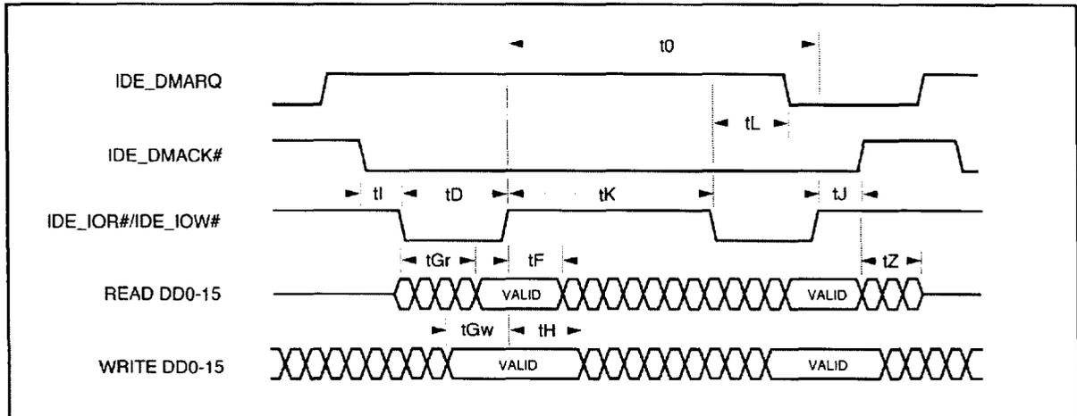
Table 6-8. Multiword DMA ATA Data Transfer Timing
