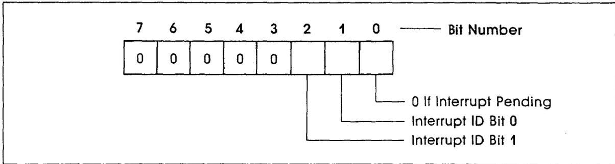
**Bit 0:** The bit can be used in either a hard-wired prioritized or polled environment to indicate whether an interrupt is pending. When bit 0 is logical 0, an interrupt is pending, and the IIR contents may be used as a pointer to the appropriate interrupt service routine. When bit 0 is logical 1, no interrupt
