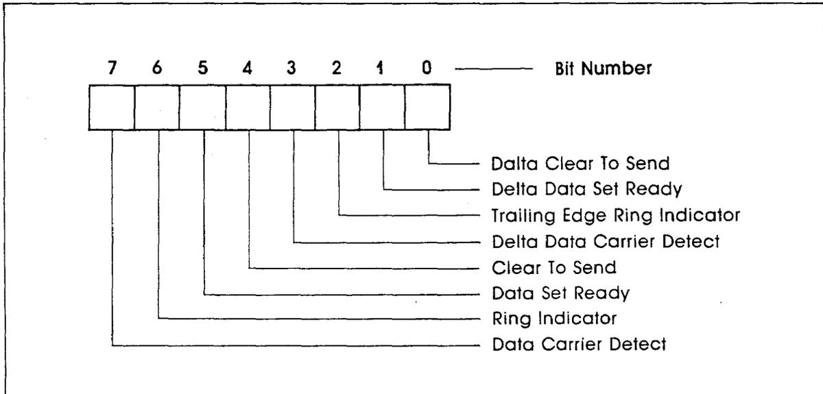
**Bit 0:** This bit is the delta clear-to-send indicator. It indicates the  $\overline{CTS}$  input to the chip has changed state since the last time it was read by the processor.
