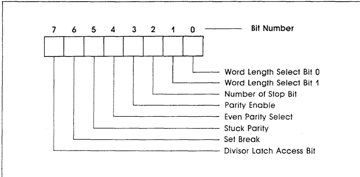
**Bits 0, 1:** These two bits specify the number of bits in each serial character that is sent or received. The encoding of bits 0 and 1 is as follows:
