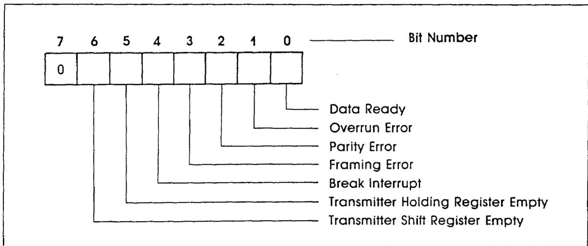
**Bit 0:** This bit is the receiver data ready (DR) indicator. It is set to logical 1 whenever a complete incoming character has been received and transferred into the Receiver Buffer register. Bit 0 may be reset to logical 0 by the processor either reading the data in the Receiver Buffer register or writing logical 0 in it.
