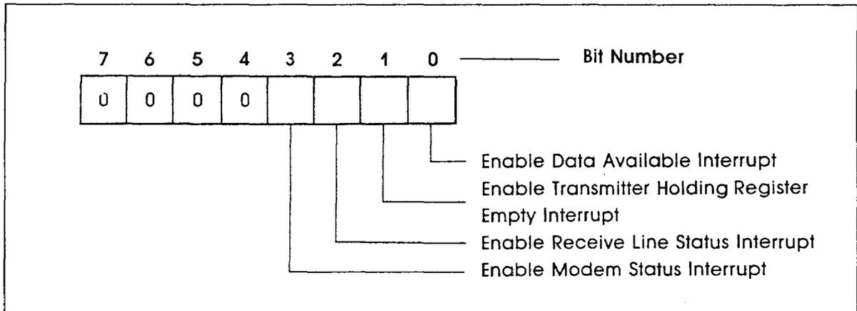
**Bit 0:** When set to logical 1, enables the received-data-available interrupt.
