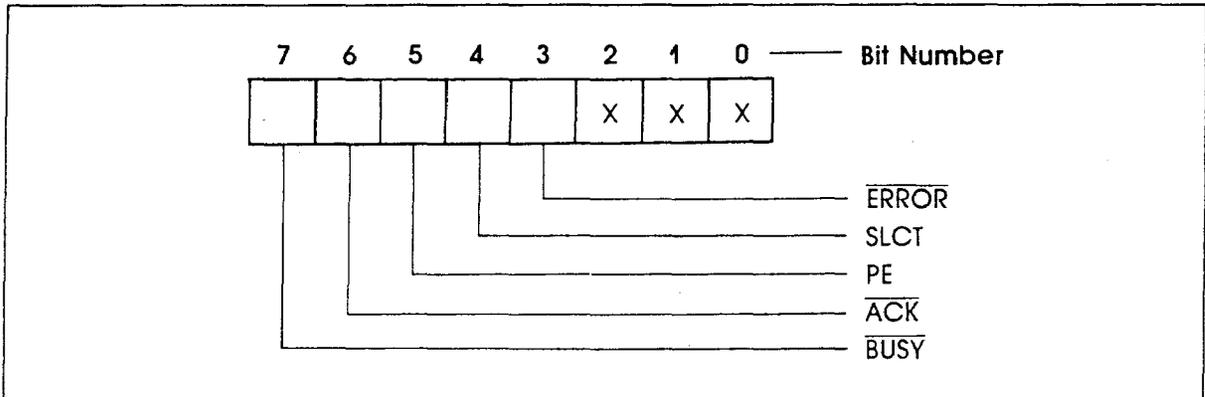
**Bit 7:  $\overline{\text{BUSY}}$** —This signal may become active during data entry, while the printer is offline, during printing, when the print head is changing positions, or while in an error state. When it is active, the printer is busy and can not accept data.
