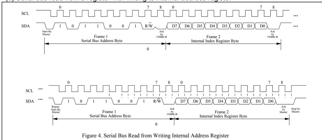
Figure 4. Serial Bus Read from Writing Internal Address Register
