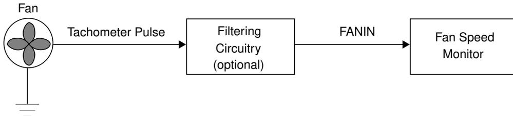
Figure 16. Fan Speed Monitor - System Configuration
