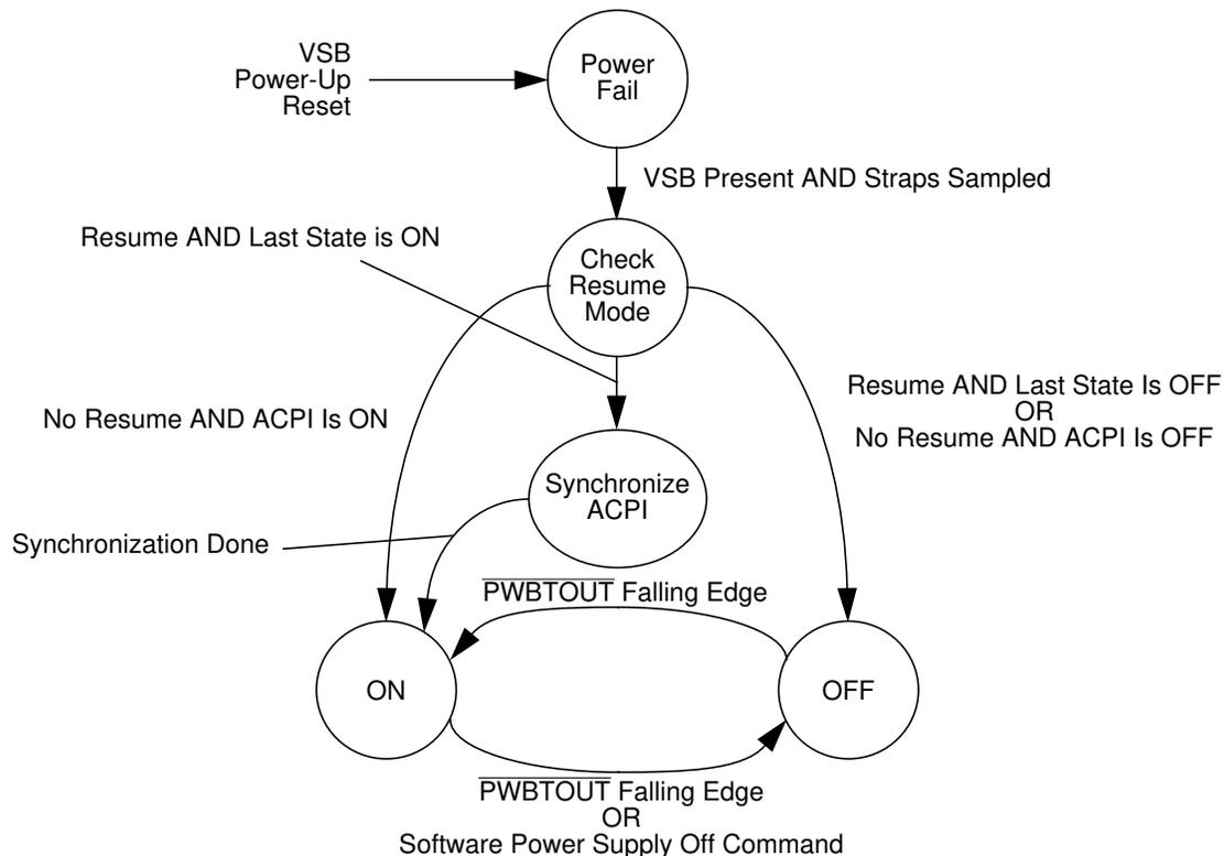
Figure 5. Legacy Power Supply Control State Diagram
