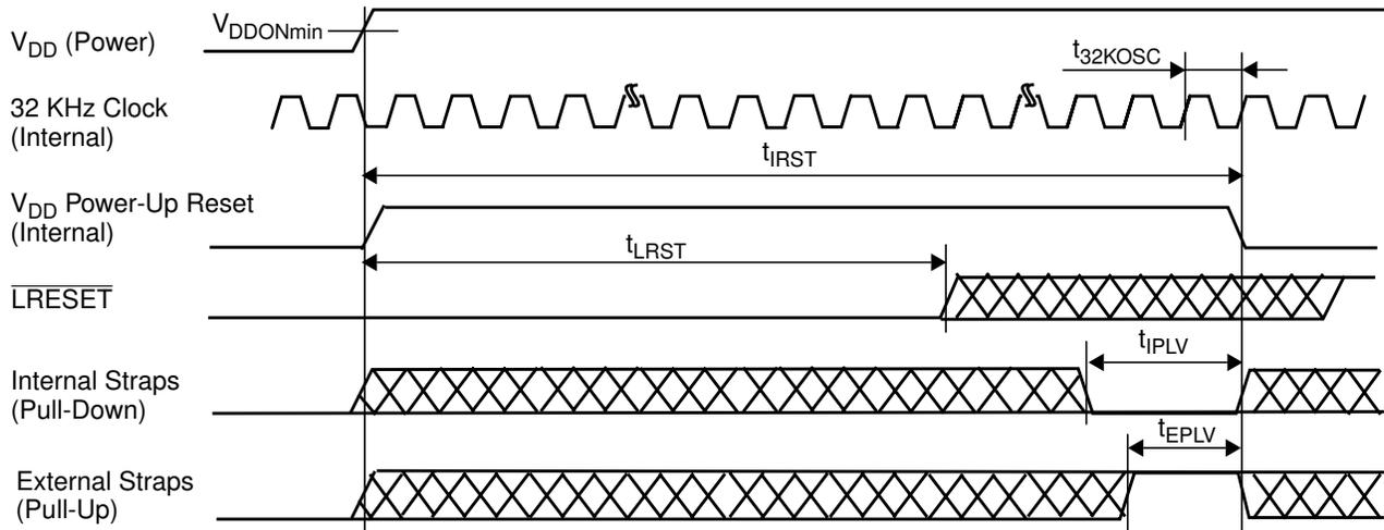
Figure 58. Internal V<sub>DD</sub> Power-Up Reset
