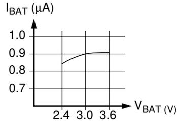
Figure 44. Typical Battery Current During Battery-Backed Power Mode
