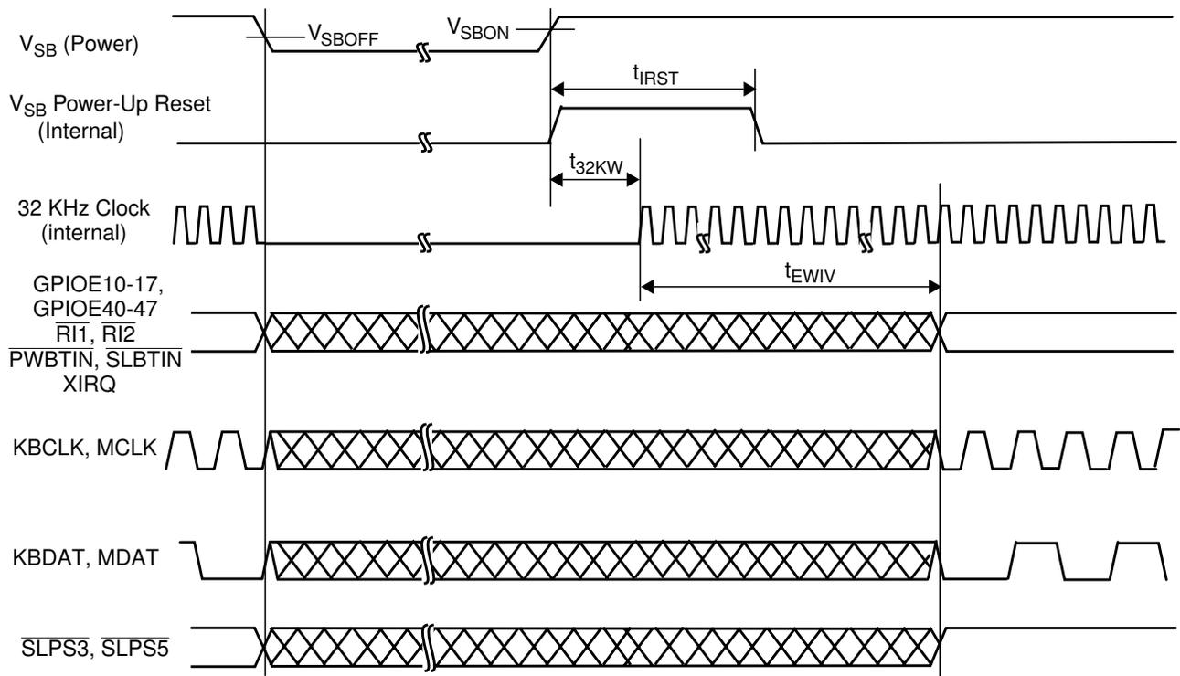
Figure 67. Inputs at  $V_{SB}$  Power Switching (No  $V_{BAT}$ )
