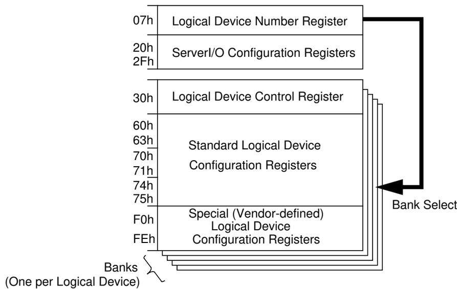
Figure 3. Structure of Standard Configuration Register File
