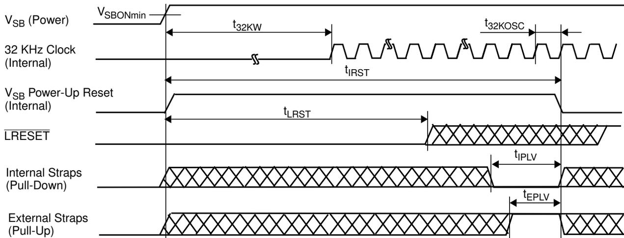
Figure 57. Internal  $V_{SB}$  Power-Up Reset (No  $V_{BAT}$ )
