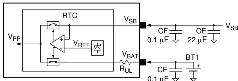
1. Place a 0.1  $\mu\text{F}$  capacitor on each  $V_{SB}$  power supply pin and on  $V_{BAT}$  as close to the pin as possible.
