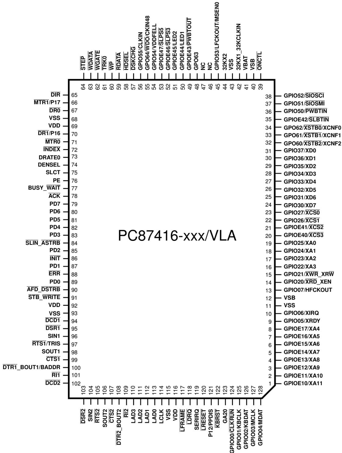
NC - Not Connected (these pins should be left unconnected)
