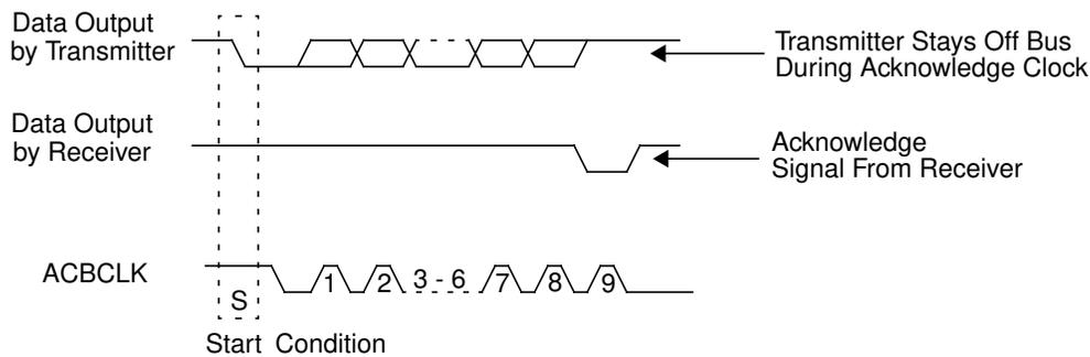
**Figure 33. ACCESS.bus Acknowledge Cycle****6.2.5 Acknowledge after Every Byte Rule**
