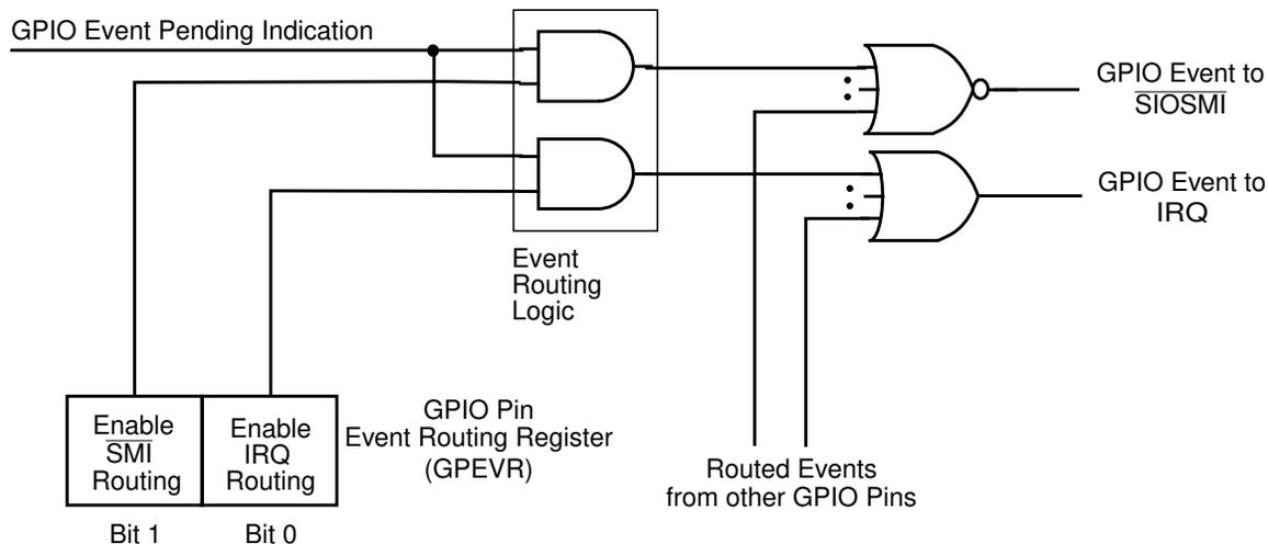
**Figure 38. GPIO Event Routing Mechanism for System Notification**
