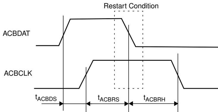
Figure 66. ACB Restart Condition Timing
