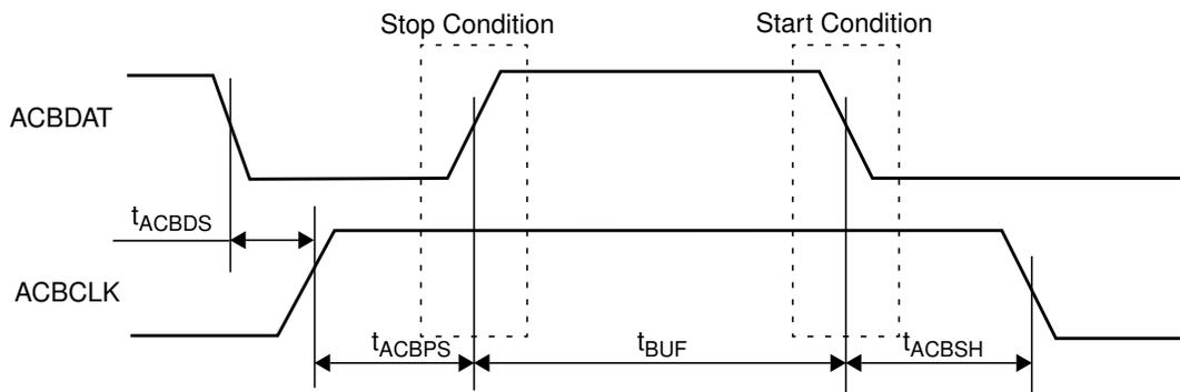
Figure 65. ACB Start and Stop Condition Timing
