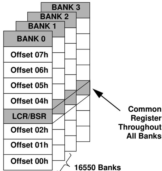
Figure 52. Register Bank Architecture
