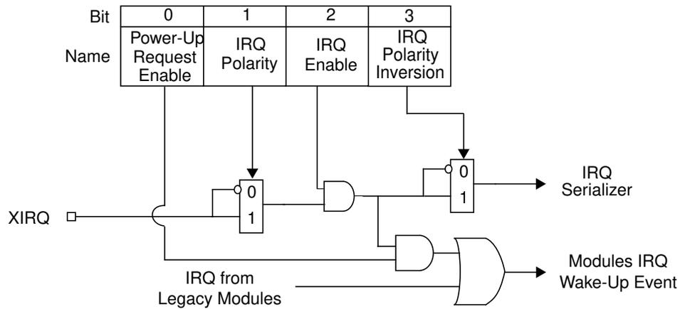
**Figure 28. Functional Illustration of X-Bus IRQ Configuration Register**
