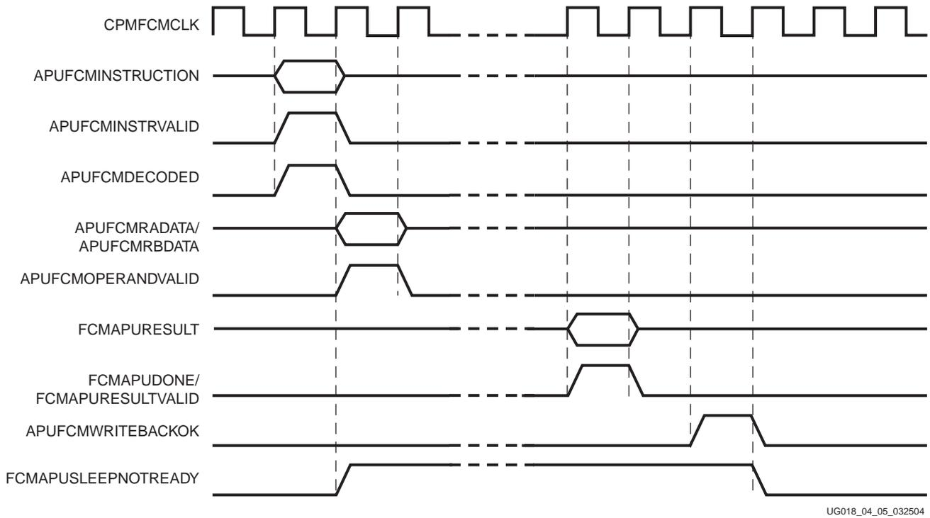
Figure 4-6: APU Controller Decoded Non-Blocking Transaction Example
