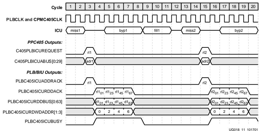
Figure 2-6: ISPLB Non-Pipelined Cacheable Sequential Fetch (Case 1)
