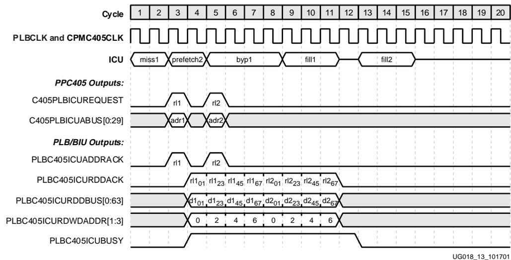
Figure 2-8: ISPLB Pipelined Cacheable Sequential Fetch (Case 1)
