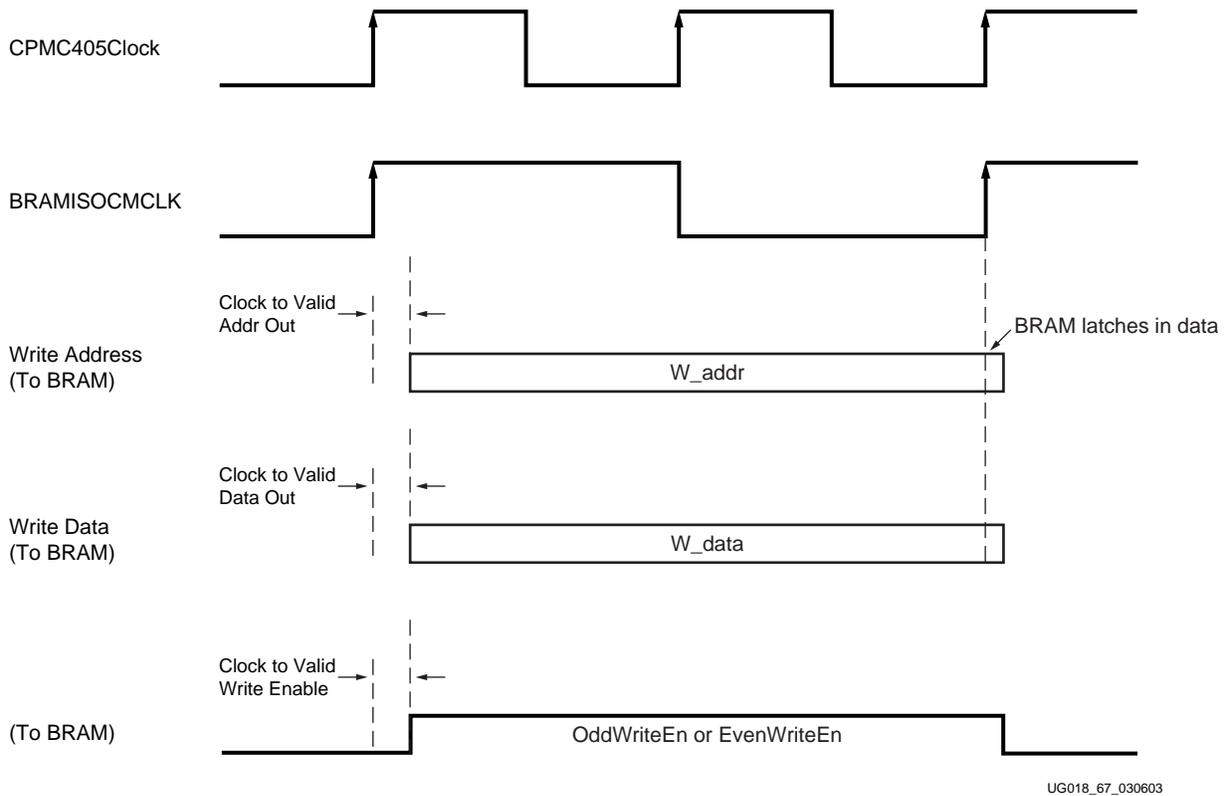
Figure 3-21: Multi Cycle Mode (2:1) ISOCM Write Timing
