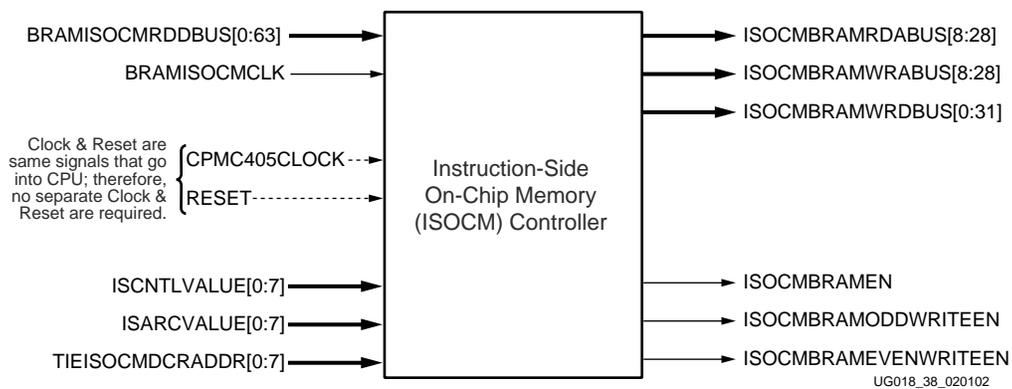
Figure 3-7: ISOCM Interface for Virtex-II Pro
