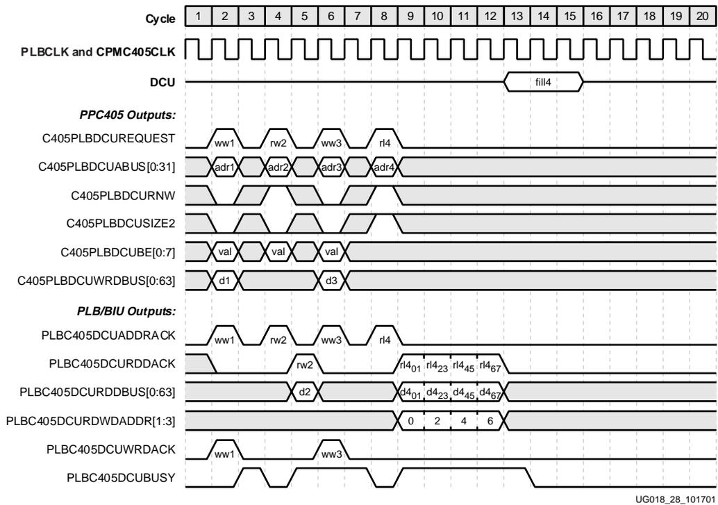
Figure 2-24: DSPLB Word Write/Word Read/Word Write/Line Read
