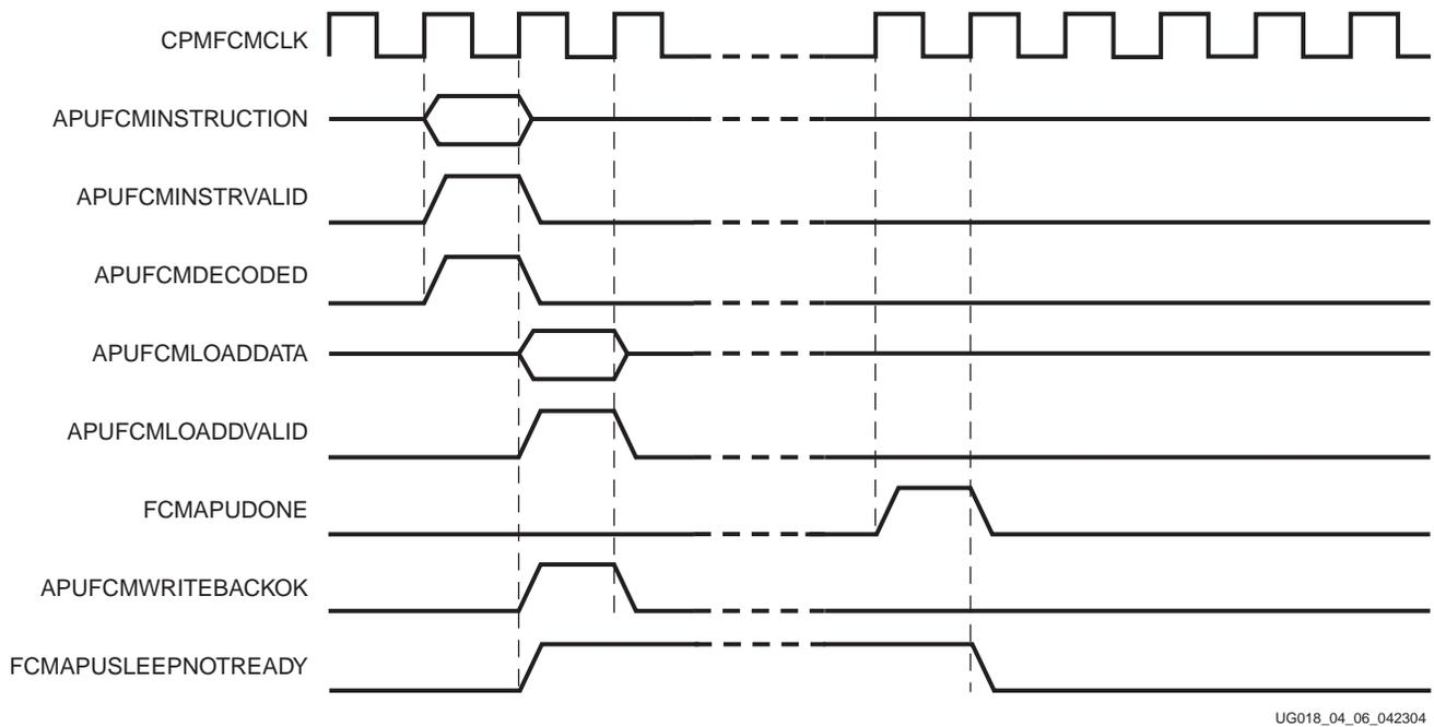
Figure 4-7: APU Controller Decoded Load Instruction Example
