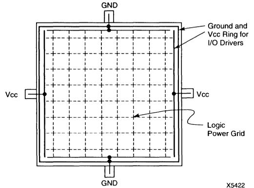
**Figure 10. LCA Power Distribution.**
