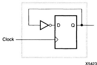
**Figure 6. Toggle Flip-Flop.** This is used to characterize device performance.
