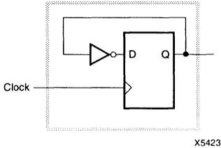
**Figure 9. Toggle Flip-Flop.** This is used to characterize device performance.
