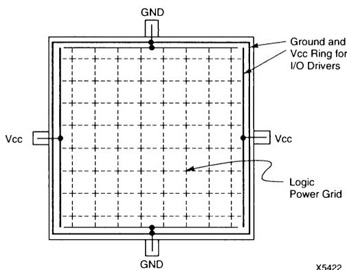
Figure 8. LCA Power Distribution.
