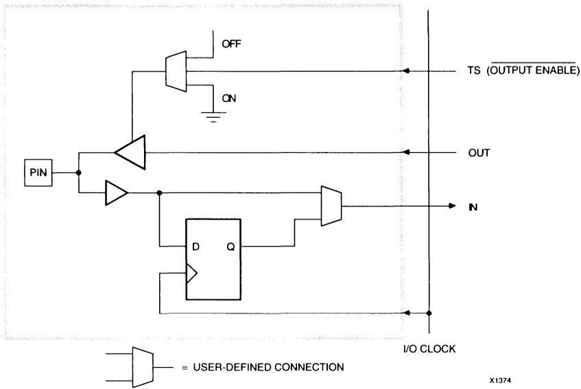
**Figure 5. Input/Output Block.** Each IOB includes an input storage element and I/O options pre-defined by the user. Passive pull-up can only be enabled on inputs, not on outputs. All user inputs are selectable for TTL or CMOS thresholds.
