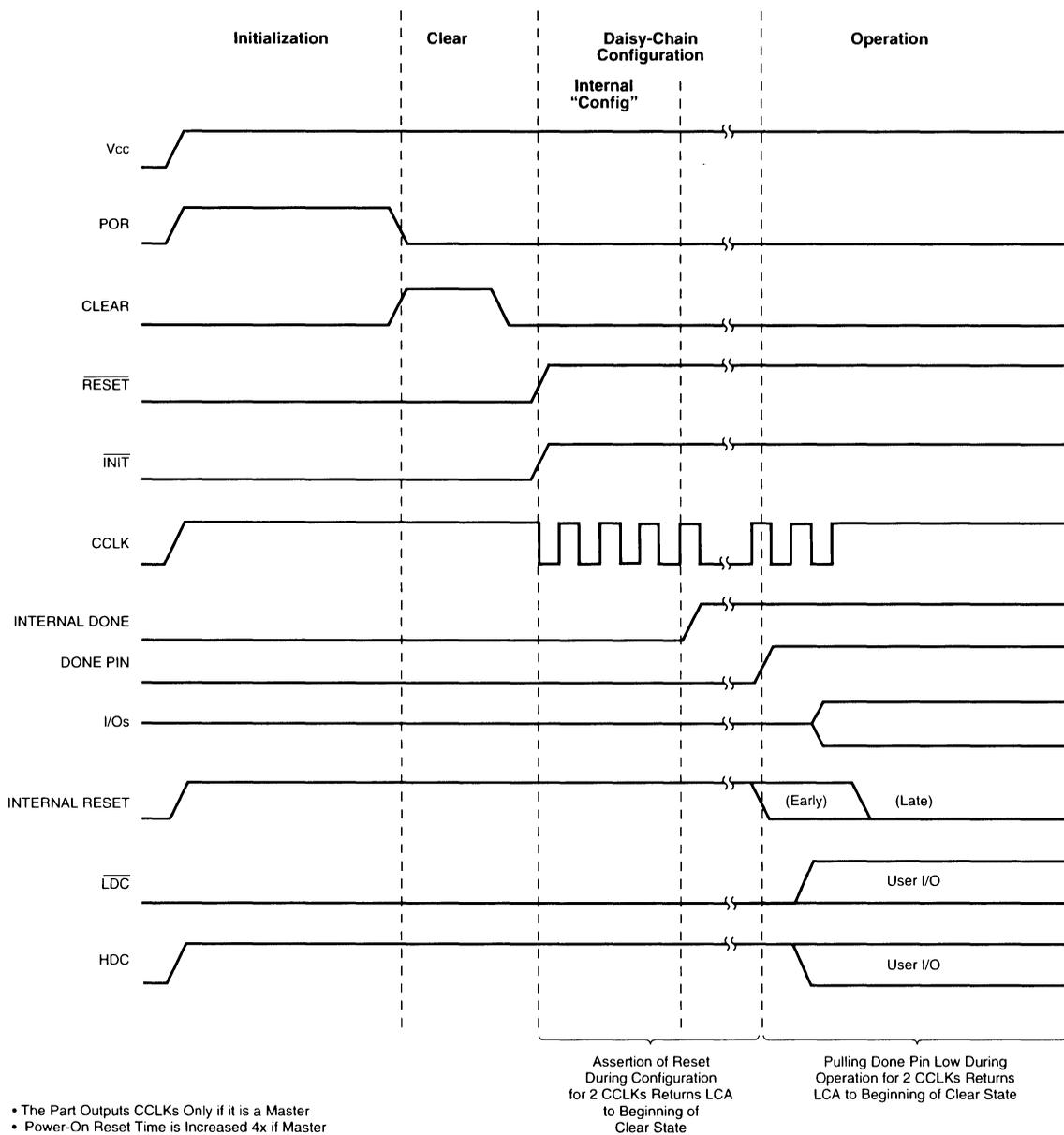
Figure 8. Pseudo-Configuration Waveform (Configuration Delay by Reset)
