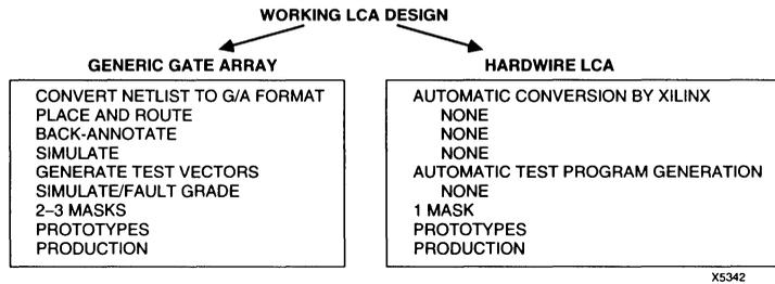
Figure 3. Design Flow Comparison: Gate Array versus Hardwire LCA.
