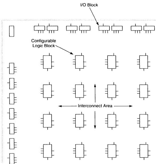
**Figure 1. Logic Cell Array Structure**
