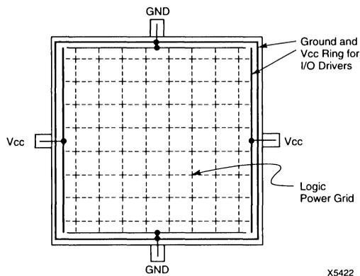
**Figure 7. LCA Power Distribution.**
