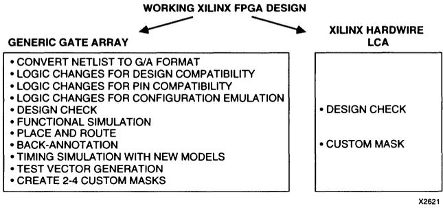
Figure 2. Design Conversion: HardWire LCA vs. Generic Gate Array
