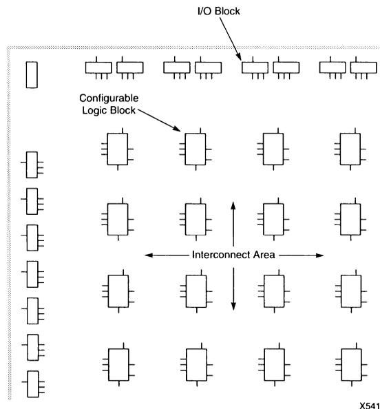
Figure 4. Logic Cell Array Structure
