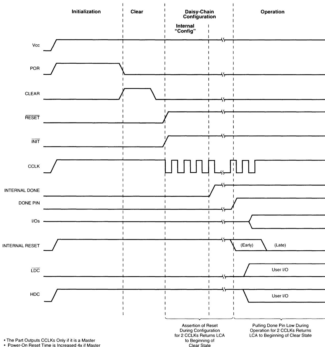
Figure 5. Pseudo-Configuration Waveform (Configuration Delay by Reset)
