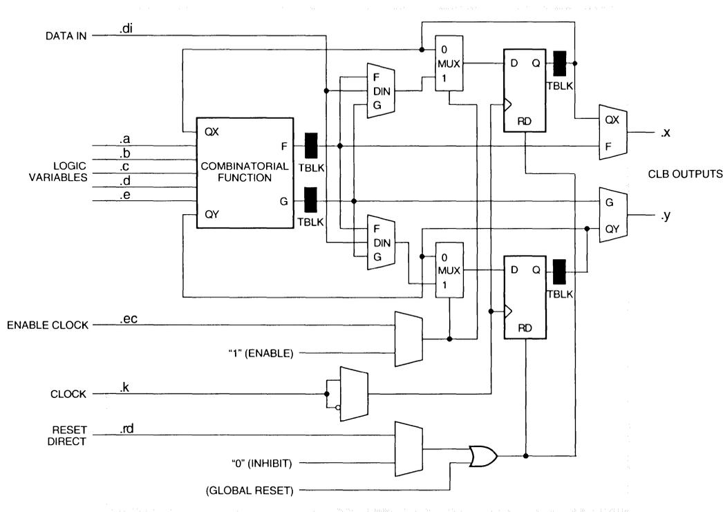
Figure 9. XC3300A, XC3300L, XC4400A HardWire CLB Test Latch Locations
