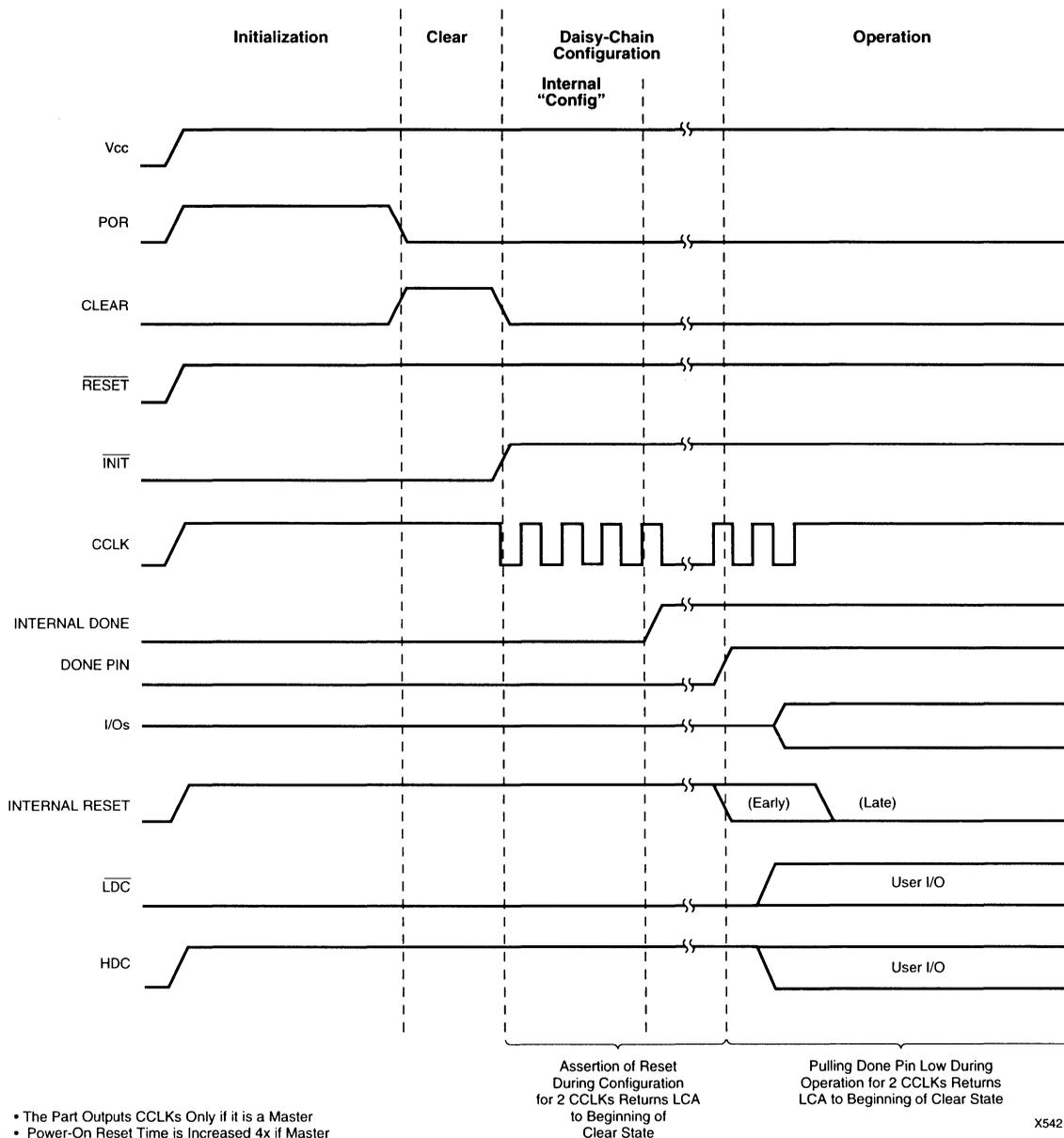
Figure 4. Pseudo-Configuration Waveform (Normal Power-Up)
