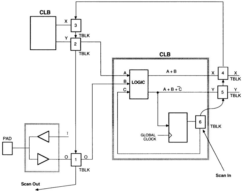
Figure 14. XC2318 Scan Test Example
