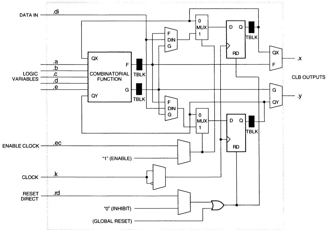
Figure 11. XC3300 HardWire CLB Test Latch Locations
