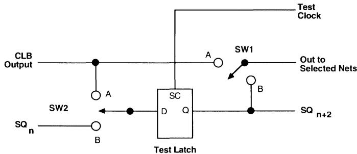
Figure 13. TBLK Block Diagram
