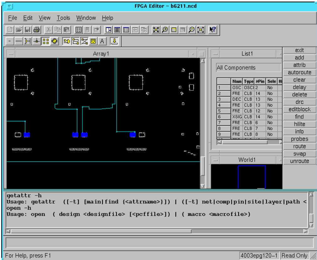
**Figure 2-2 FPGA Editor Main Window**
