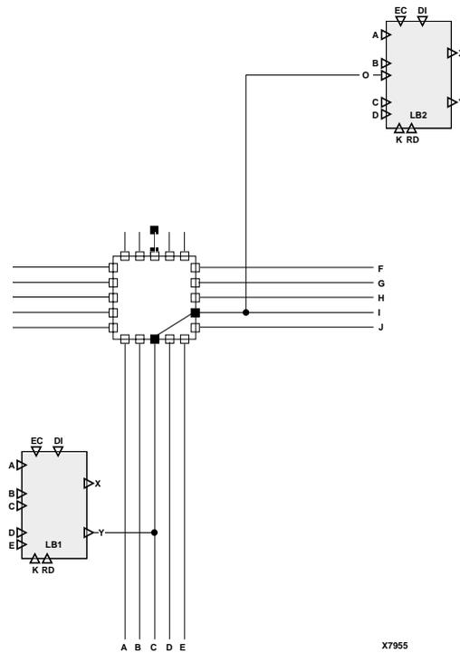
Figure 6-1 Routing Example
