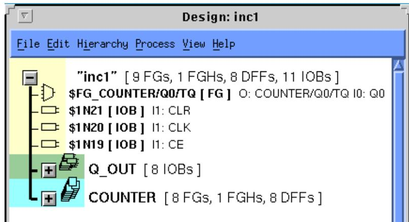
**Figure 4-30 Design Example Design Hierarchy**
