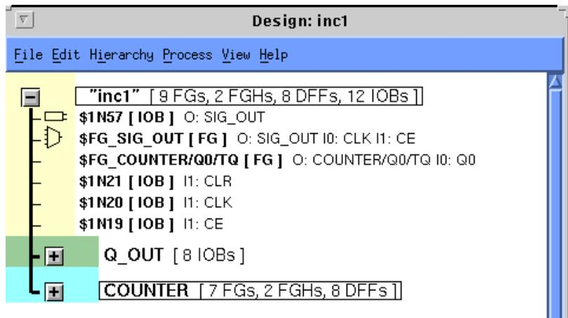
**Figure 4-33 Design Hierarchy of New NCD File**
