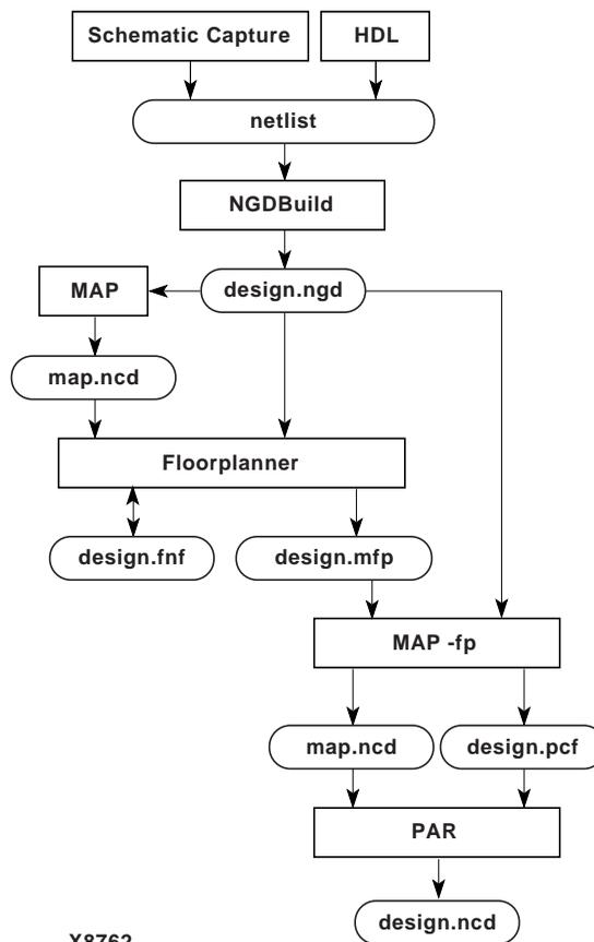
Figure 2-2 Floorplan First Design Flow
