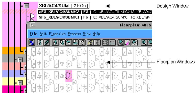
**Figure 4-14 Placed Logic Symbol in the Floorplan Window**
