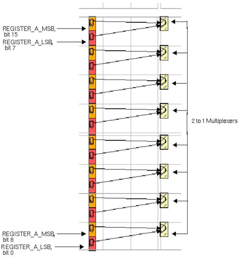
**Figure 4-26 2-in-1 Multiplexers Placed to Align with A/Q Bus**
