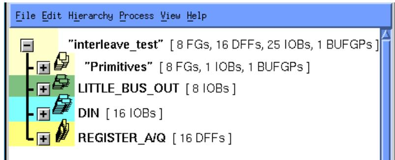
**Figure 4-19 Interleave Design Hierarchy**
