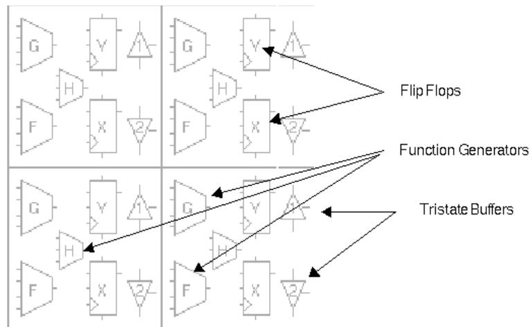
**Figure 4-12** Display of Resources in the Floorplan Window
