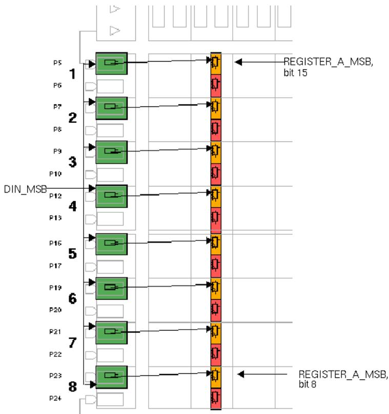
**Figure 4-24** DIN\_MSB Placed to Align with REGISTER\_A\_MSB
