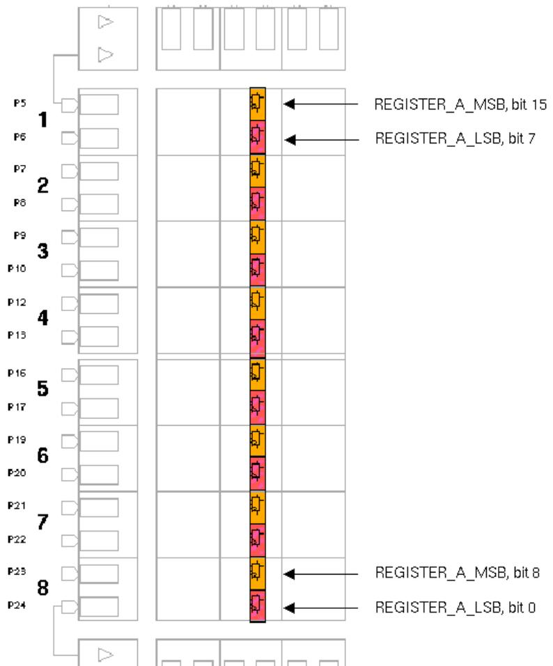
**Figure 4-23 REGISTER\_A\_LSB Group Interleaved with REGISTER\_A\_MSB**
