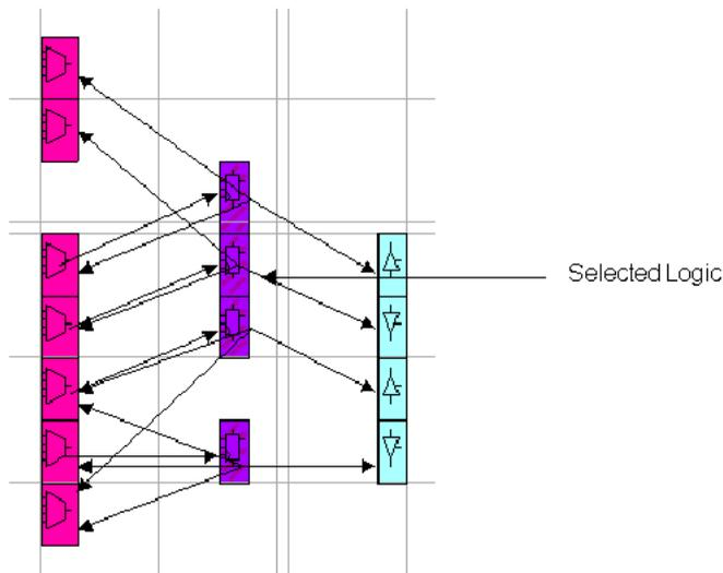
**Figure 4-9 Viewing Placed Logic Symbols Using the Ratsnest**
