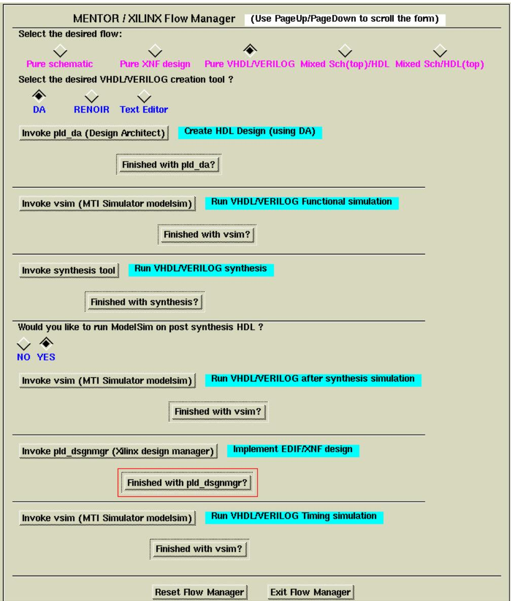
Figure 7-7 Mentor/Xilinx Design Manager Pure VHDL/Verilog Mode Running ModelSim on Post Synthesis HDL
