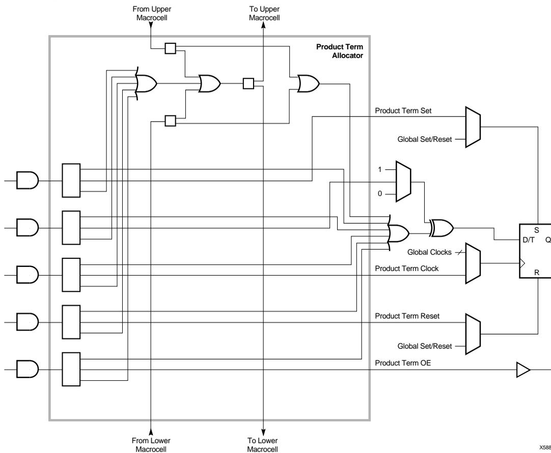
Figure 16: Product Term Allocator Logic
