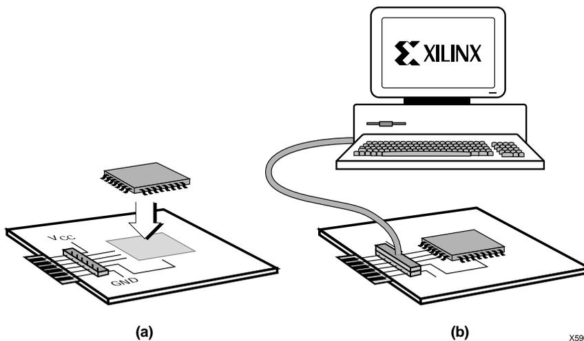
**Figure 21: In-System Programming Operation (a) Solder Device to PCB and (b) Program Using Download Cable**
