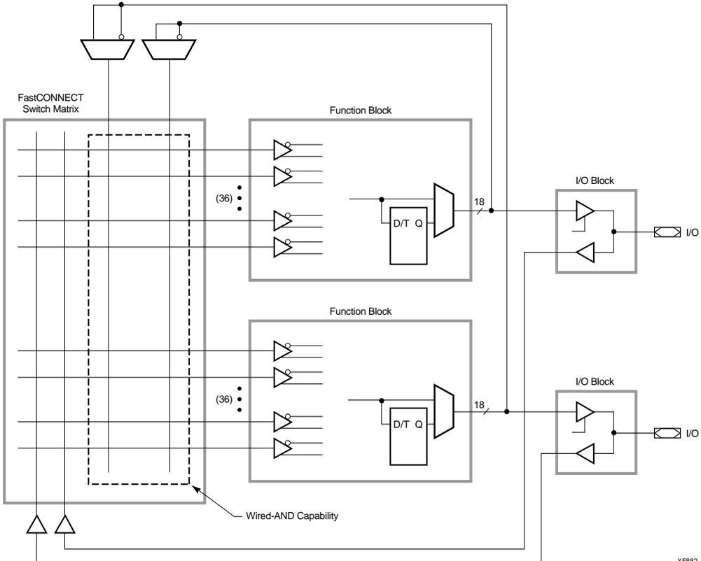
Figure 17: FastCONNECT Switch Matrix
