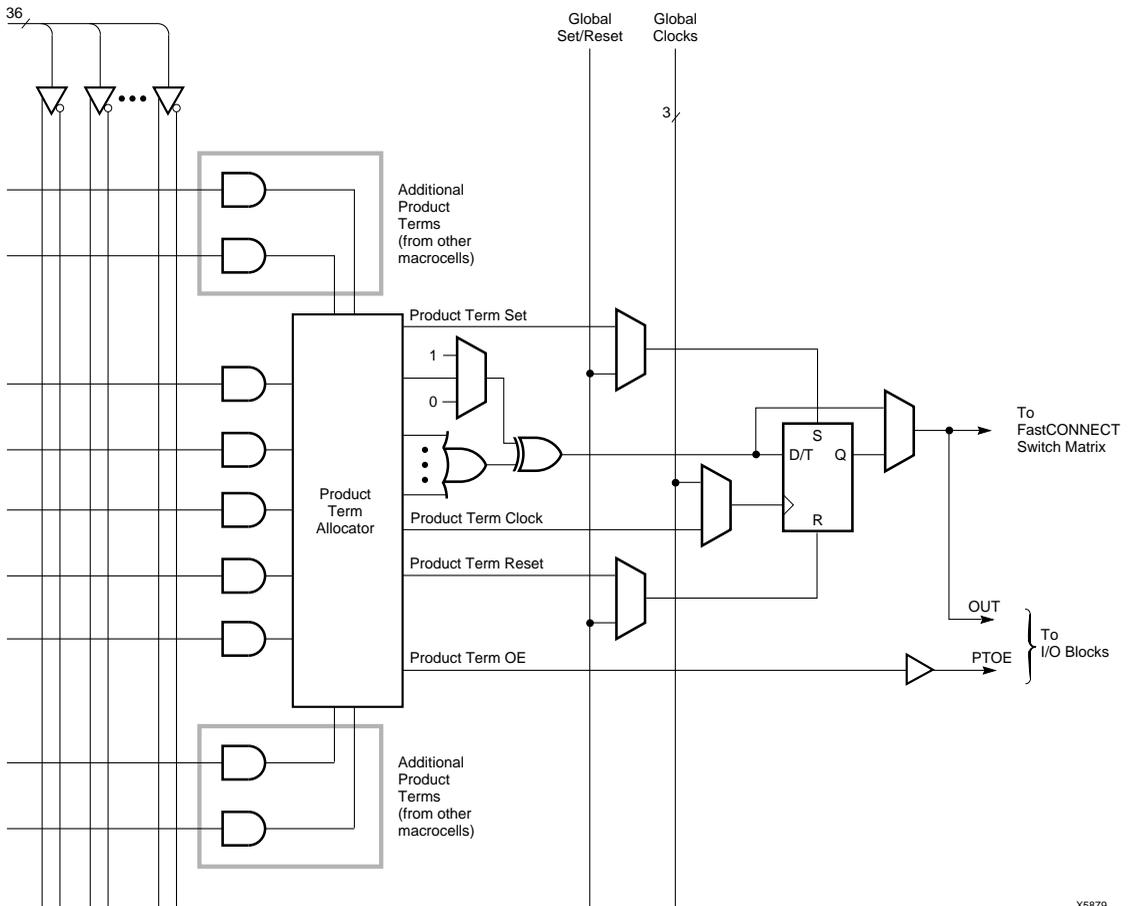
Figure 11: XC9500 Macrocell Within Function Block
