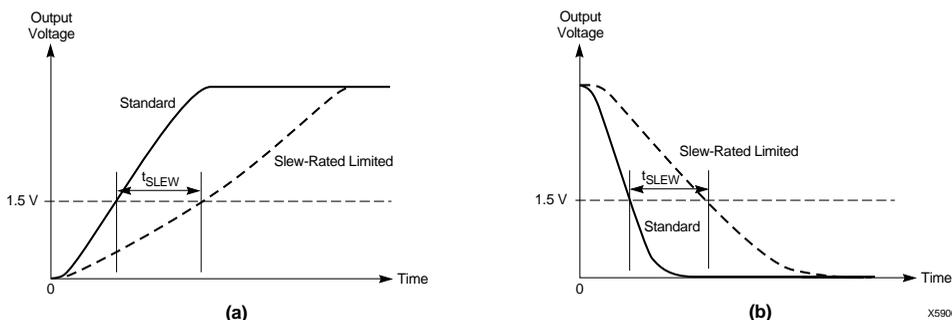
Figure 19: Output Slew-Rate Control For (a) Rising and (b) Falling Outputs
