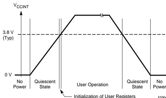
Figure 24: Device Behavior During Power-up
