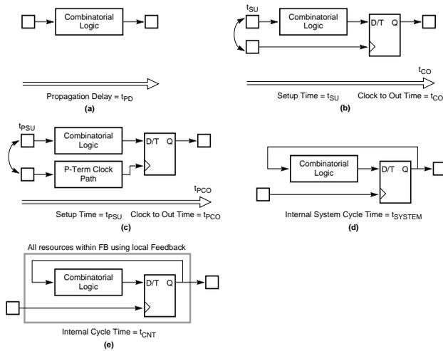
Figure 22: Basic Timing Model
