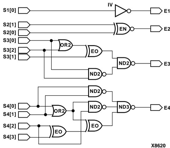
Figure 6-5 Concurrent CHECK Procedure Design
