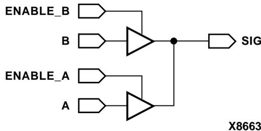
**Figure 6-3 Two Three-State Buffers Driving the Same Signal**
