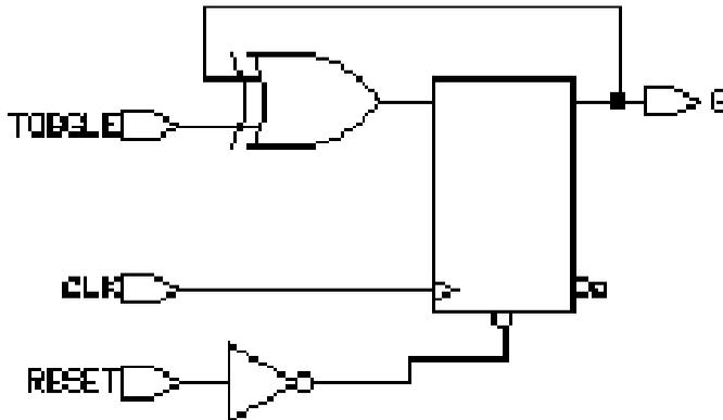
**Figure 7-22 Toggle Flip-Flop with Enable and Asynchronous Reset**
