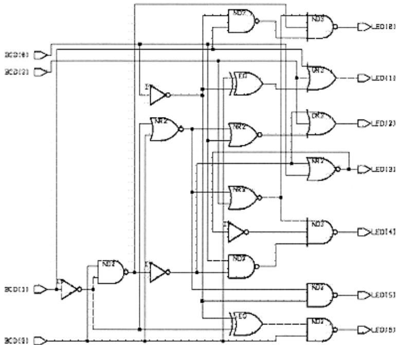
Figure 8-18 Seven-Segment LED Decoder with O LED Default
