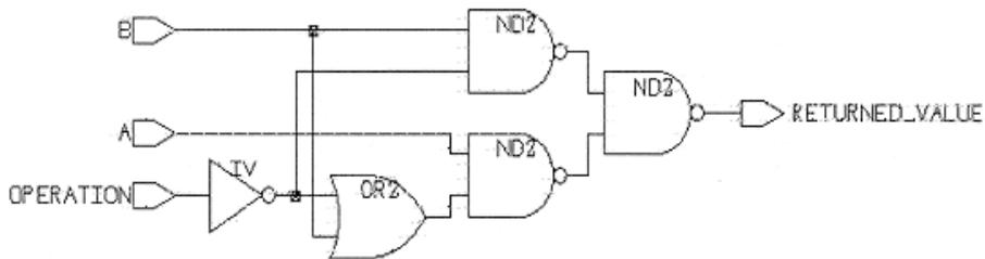
**Figure 5-10** Circuit for Using Multiple return Statements
