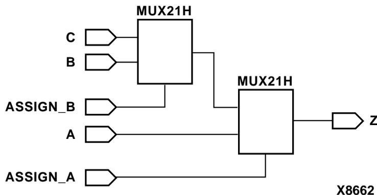
**Figure 6-6 Conditional Signal Assignment Design**
