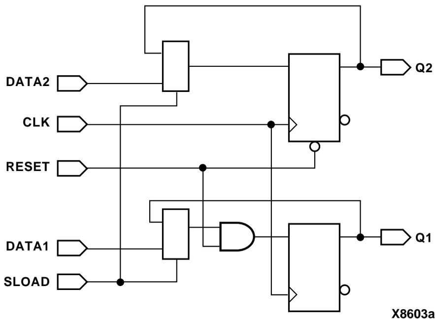
**Figure 7-17 Multiple Flip-Flops with Asynchronous and Synchronous Controls**
