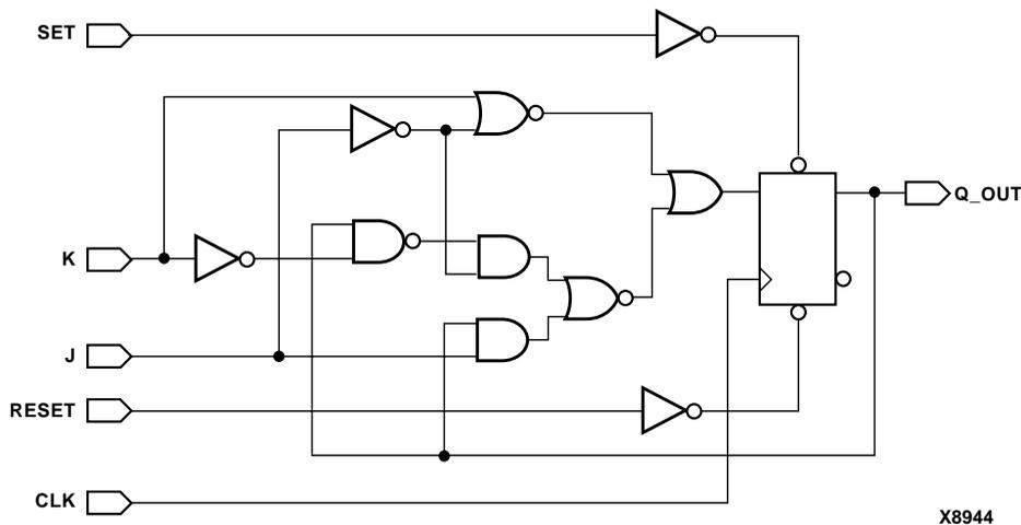
Figure 7-19 JK Flip-Flop with Asynchronous Set and Reset
