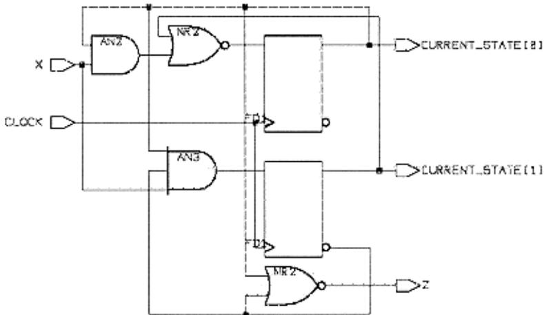
Figure 8-13 Schematic of an Improved State Machine
