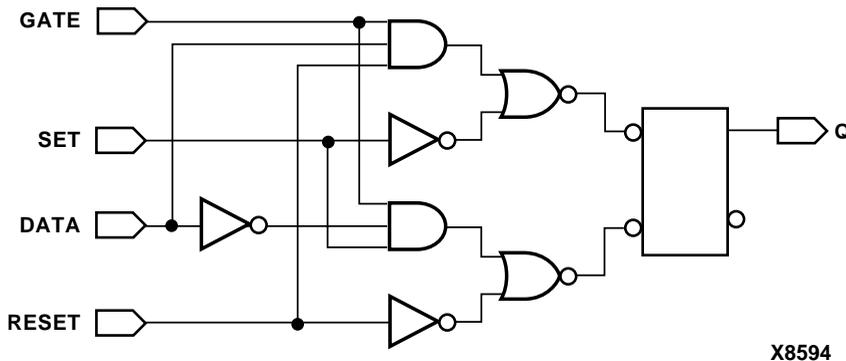
**Figure 7-5 D Latch with Asynchronous Set and Reset**
