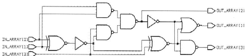
Figure 5-9 Circuit Design for Procedure Call to Sort an Array
