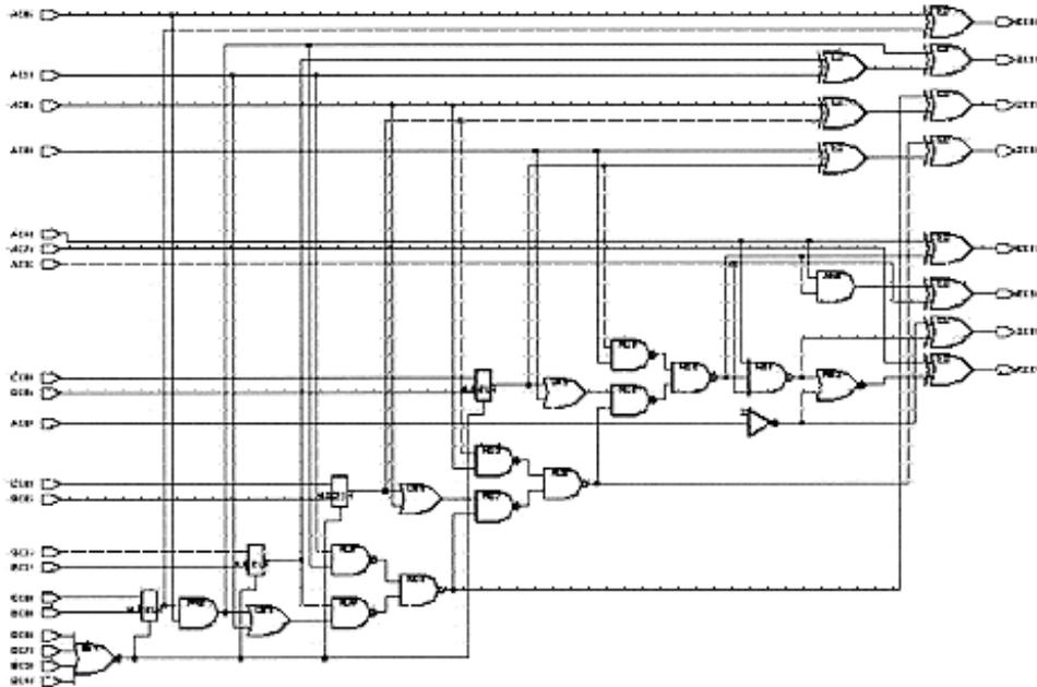
Figure 8-11 Using TEMP Declaration to Save Circuit Area
