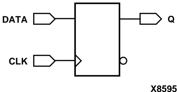
**Figure 7-8 Positive Edge-Triggered D Flip-Flop Using rising\_edge**
