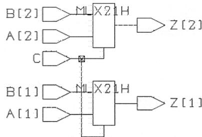
**Figure 5-12** Circuit Design without Component Implication Directives
