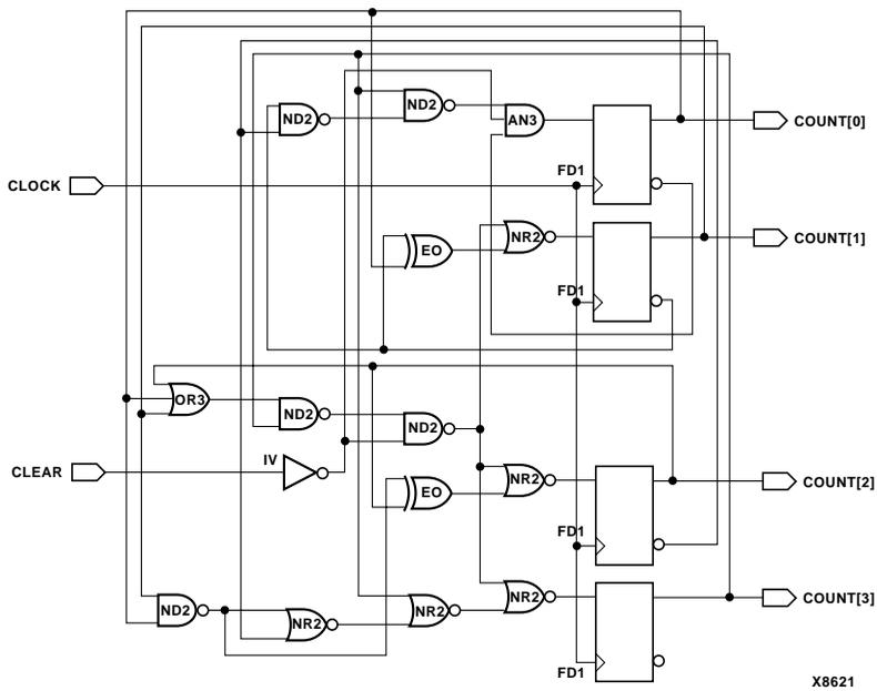
**Figure 6-2 Modulo-10 Counter Process with wait Statement Design**
