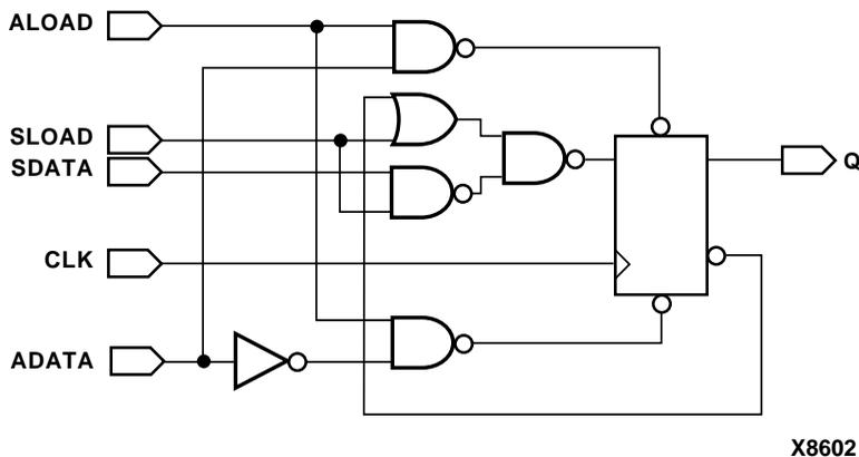
**Figure 7-16 D Flip-Flop with Synchronous and Asynchronous Load**
