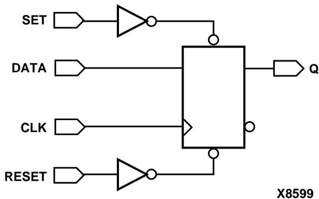
**Figure 7-13 D Flip-flop with Asynchronous Set and Reset**
