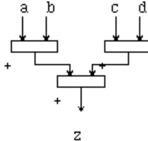
Figure 8-3 Diagram of 4-Input Adder With Parentheses
