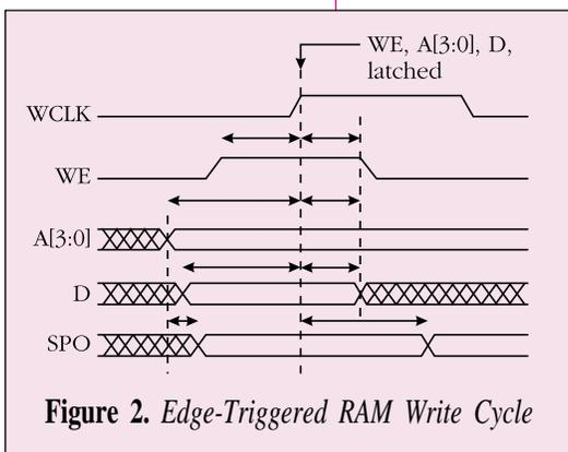
Figure 2. Edge-Triggered RAM Write Cycle
