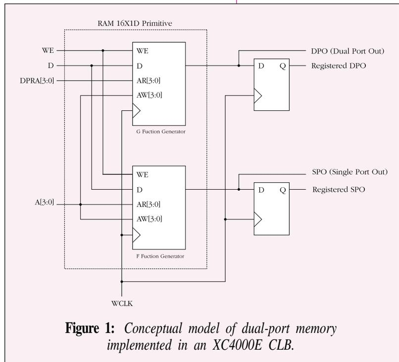
**Figure 1:** Conceptual model of dual-port memory implemented in an XC4000E CLB.
