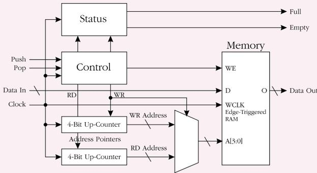
Figure 2: FIFO with edge-triggered RAM
