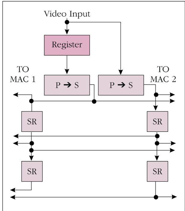
Figure 5 - (right) Sharing input shift registers between parallel MACs.
