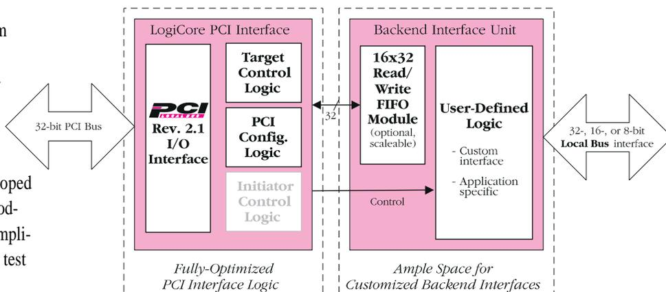
programmable gates remain free for integration of the unique, back-end functions of the application. This is a high-performance, one-chip solution.
