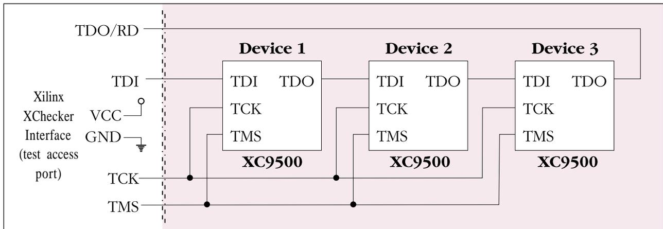
and then shifting out the result, you can effectively and automatically test devices and their interconnections on a PC board.
