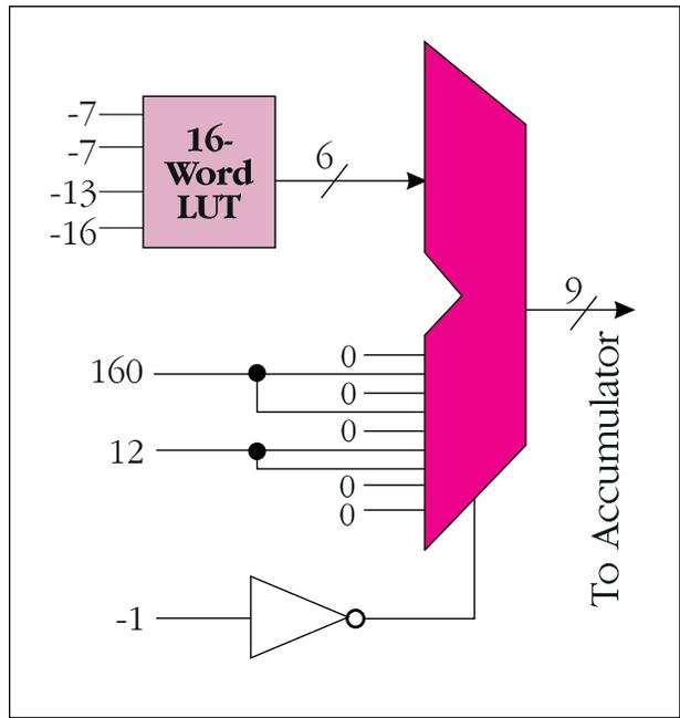
Figure 4 - (top) Final implementation of Laplacian operator.
