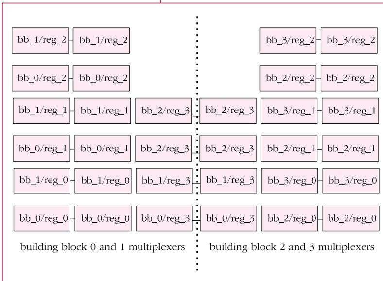
**Figure 7** Register Array Floorplan Layout (bottom half)
