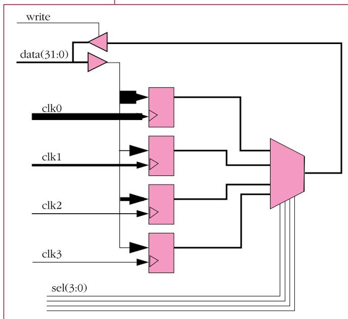
The basic building block for this design can be implemented in two different ways. The first uses two sum-of-product cells and an OR cell to generate the 4-to-1 multiplexer, and uses a total of 11 CLCs per bit slice (Figure 2). The second uses four three-state buffers to generate the 4-to-1 multiplexer, and uses a total of 12 CLCs per bit slice (Figure 3). To determine which approach is better, the user must examine how the design will fit into the XC8100 FPGA architecture as a whole.
