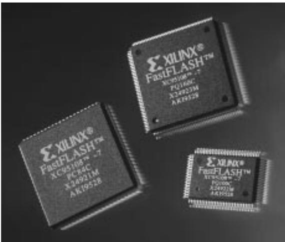
devices with multiple codes, and abolishes the stand-alone programming step. The resulting reduction in programming time also results in significant cost savings, especially at high unit volumes. Furthermore, built-in version control and in-system board customization contribute to manufacturing flexibility, saving time and money.
