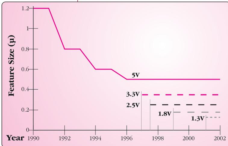
**Rapidly shrinking device geometries will require the use of smaller supply voltages.**
