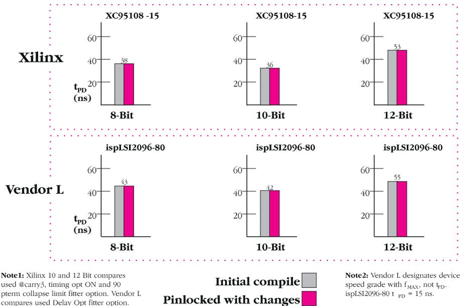
to measure the effect of routing resources and function block fan-in on the CPLD's pinlocking performance. A typical design change involves the correction of an error in which one of the input data paths was ordered incorrectly.
