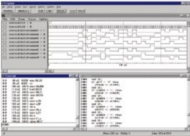
Figure 4 - Screen dump of Bus Monitor Model Technology's V-System.
