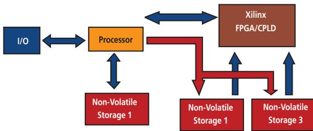
Figure 4 - Basic system architecture.
