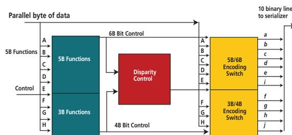
Figure 2 - 8B/10B encoder logic block diagram.
