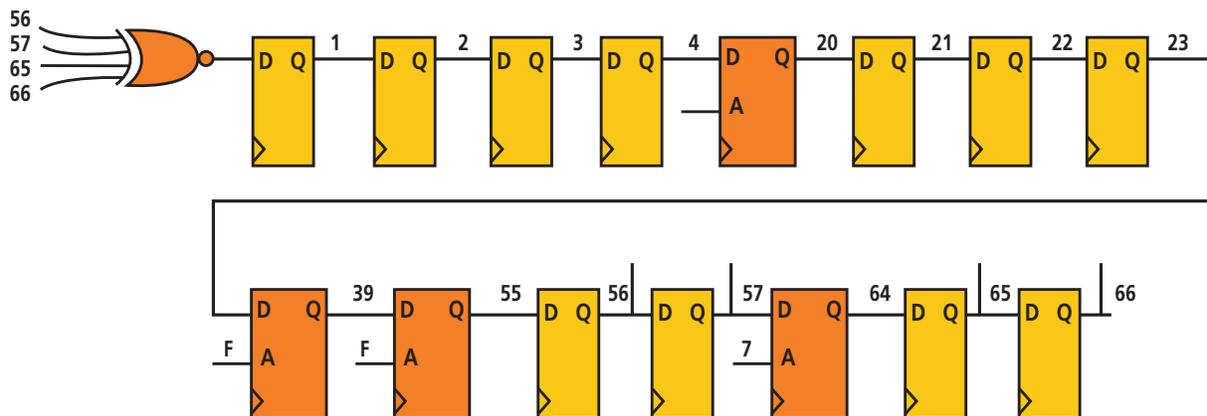
Figure 6 - Example of an LFSR counter.
