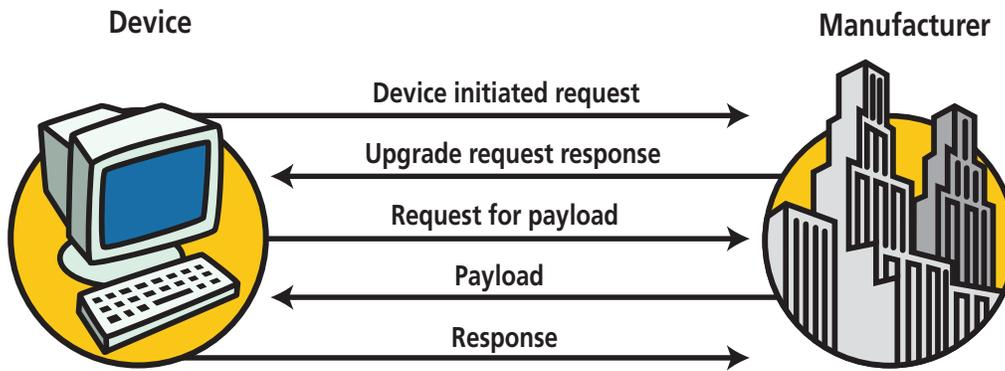
Figure 1 - The remote upgrade process.
