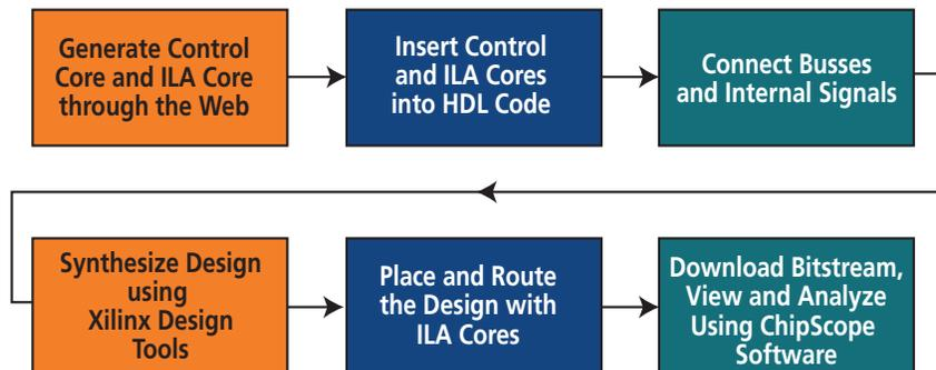
Figure 2 - ChipScope ILA flow.
