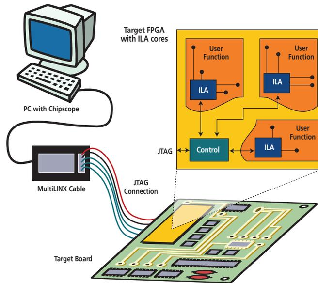
Figure 1 - Integrated Logic Analyzer (ILA) block diagram.
