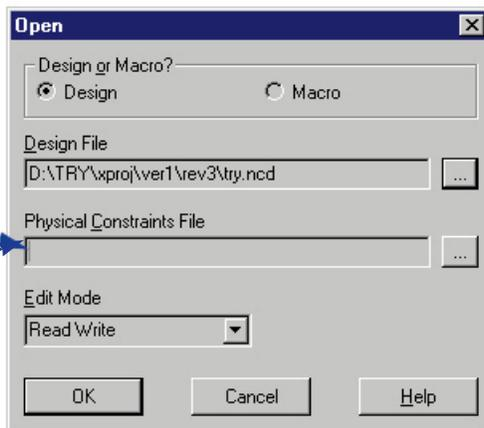
Figure 4 - Omit the PCF file to speed routing times.
