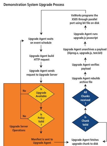
Figure 3 - Demonstration system upgrade process.
