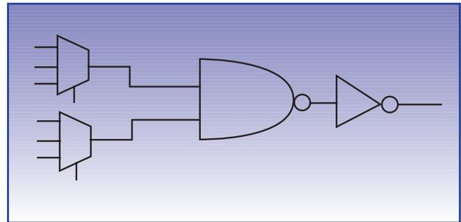
Figure 1 - CoolRunner Fast Zero Power AND gate.
