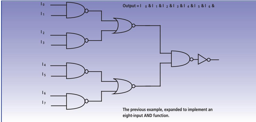
Figure 3 - Expanding the number of inputs.
