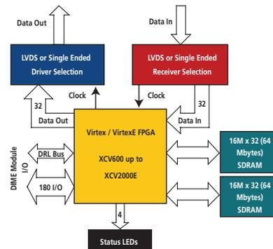
Figure 1 - Ballyderl block diagram.
