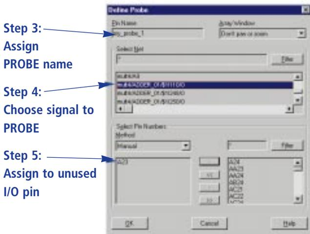
Figure 2 - Assigning signals to probes.
