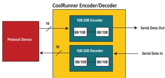
Figure 1 - 16B/20B block diagram.
