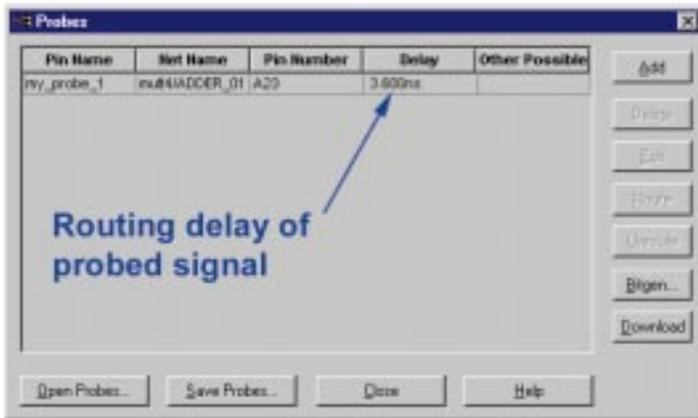
Figure 3 - Routing delay of probed signal.
