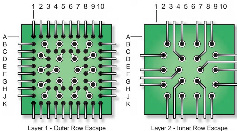
Figure 3 - 56-ball grid array in a chip scale package
