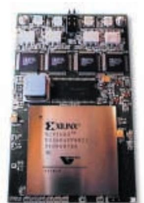
Figure 3 - Ballyriff 4-Channel 100 MSPS 12-bit ADC DIME module
