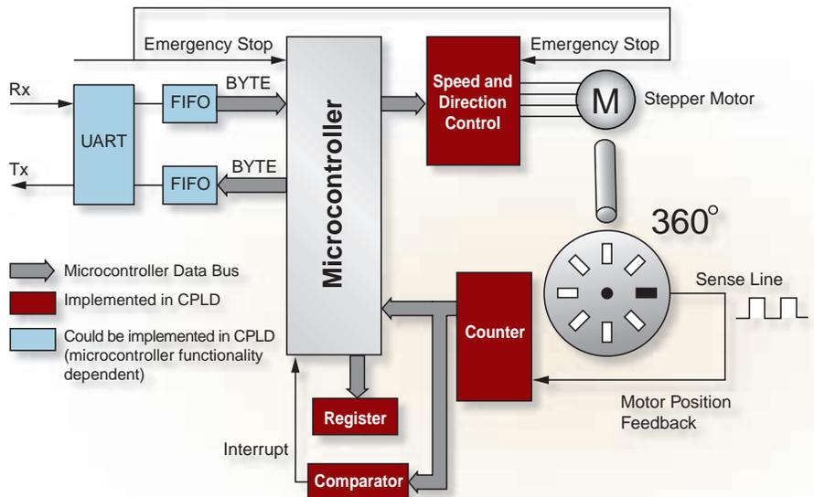
Figure 7 - Partitioned Design: Microcontroller and CPLD
