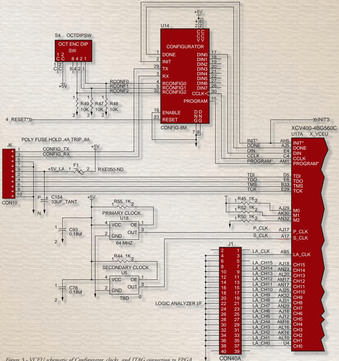
Figure 3 - VCEU schematic of Configurator, clocks, and JTAG connection to FPGA
