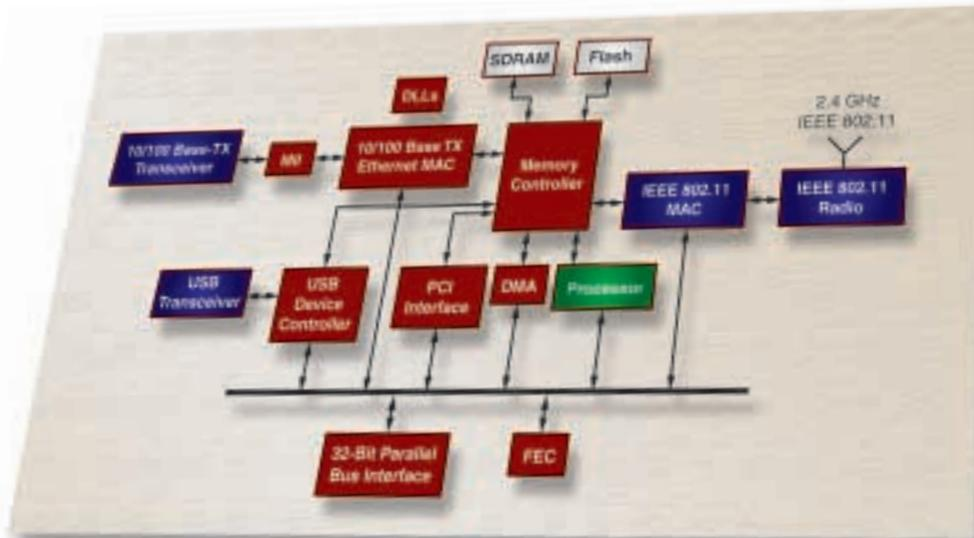
Figure 2 - Wireless LAN-to-Ethernet home networking bridge
