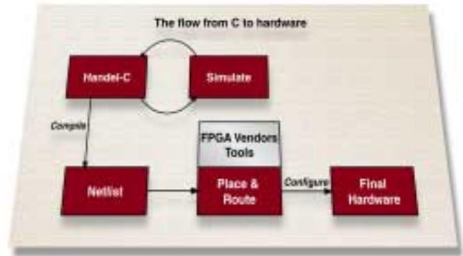
Figure 3 - Handel-C design flow
