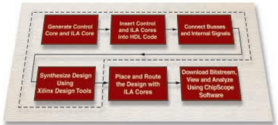
Figure 1 - ChipScope flow handled by Certify software
