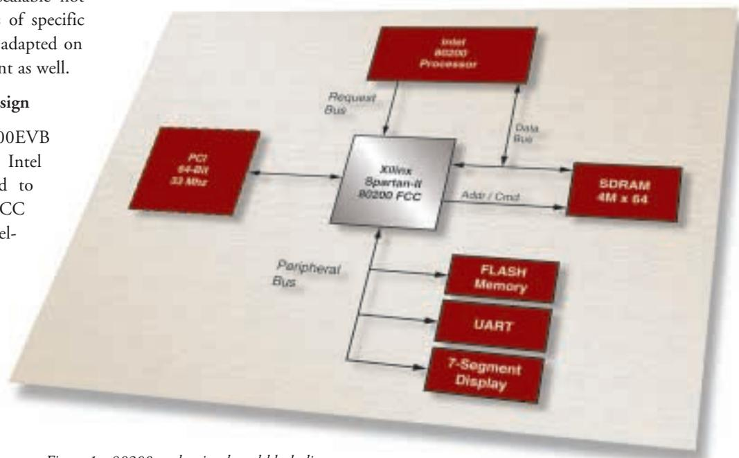
Figure 1 - 80200 evaluation board block diagram
