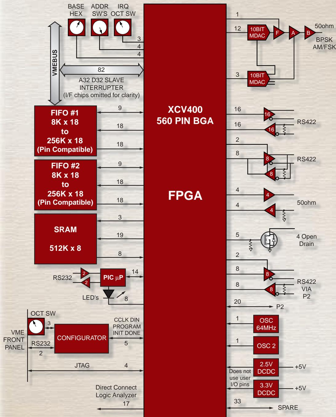
Figure 2 - VCEU FPGA interfaces
