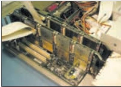
Figure 2 - High performance FPGA system with 16 Virtex-E devices capable of over 200 billion MACs
