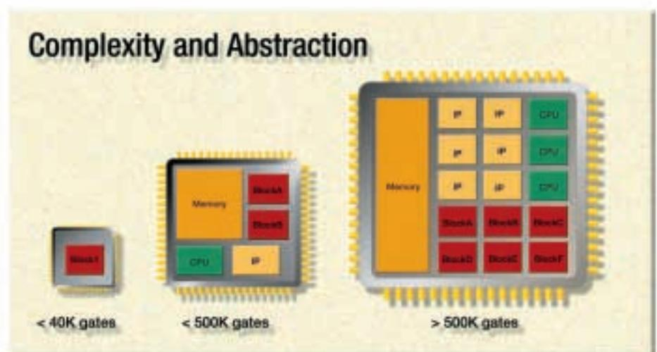
Figure 1 - The increasing density, higher speeds, and application of mixed design with IP cores has enabled the new FPGA/SoC environment.
