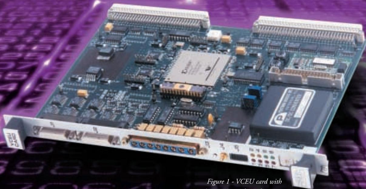
*Figure 1 - VCEU card with XCV400 FPGA and Configurator*
