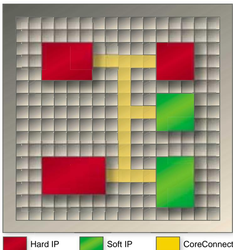
con area. The Virtex-II IP-Immersion architecture accommodates virtually any pre-defined rectilinear shape.
