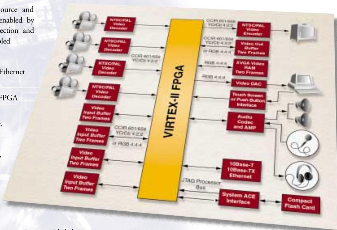
Figure 1 - Block diagram
