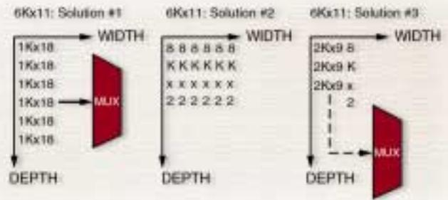
Figure 2 - Three 6Kx11 Block Memory solutions
