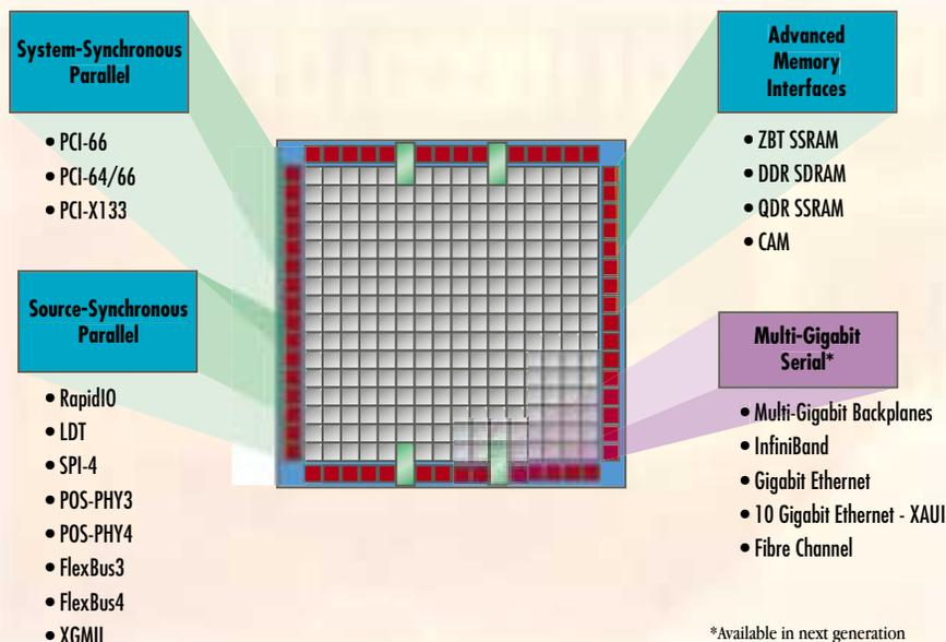
provides both physical interfaces as well as various cores that support the network protocols. With the transition from shared busses to switched fabrics comes a variety of different source-synchronous (parallel) protocols. The following are some of the leading source-synchronous standards that are emerging:
