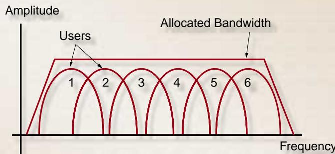
Figure 1 - OFDM allows for greater spectral efficiency
