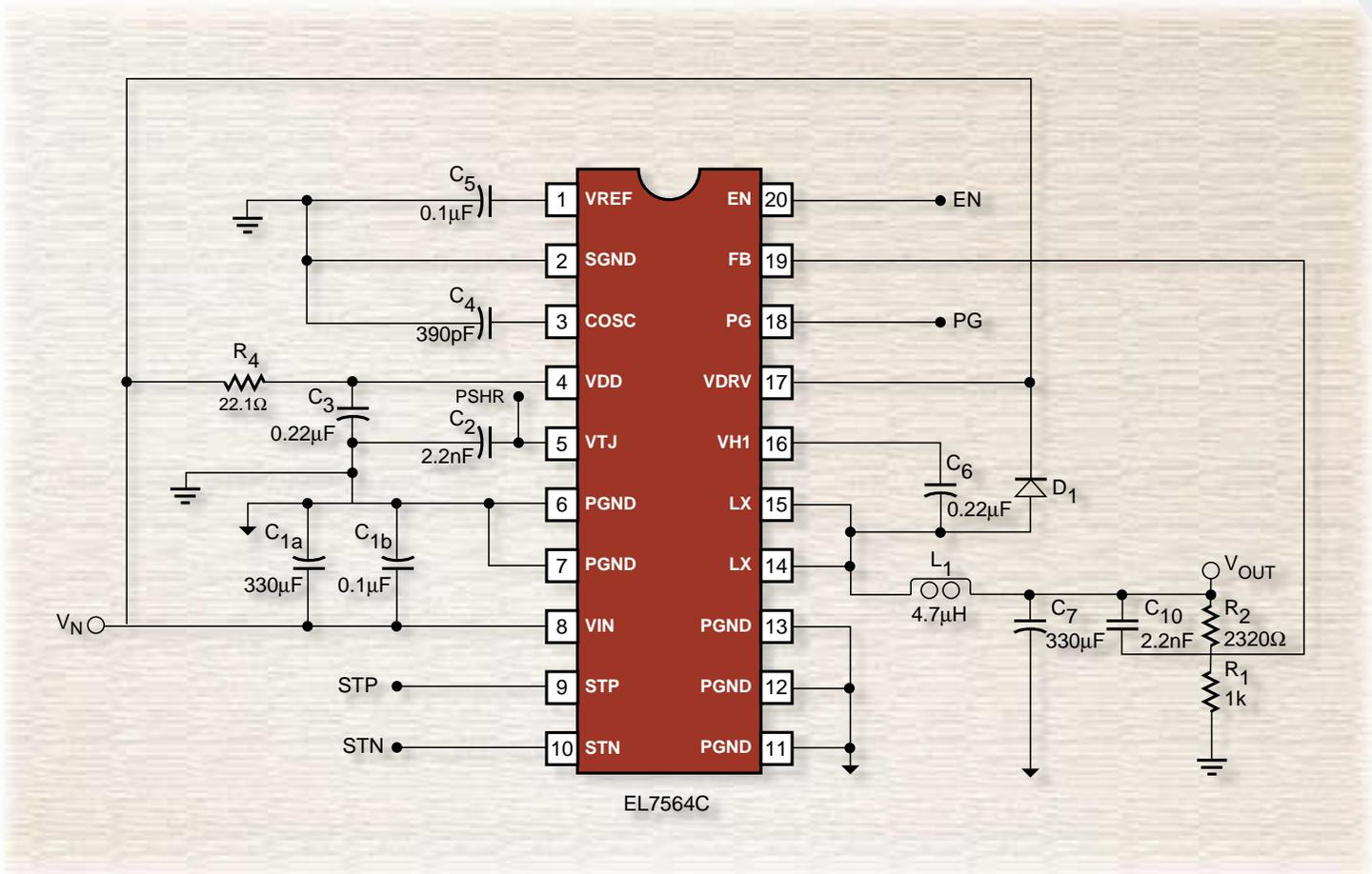
Figure 1 - EL7564C Board Circuit Schematic (VIN = 5V)
