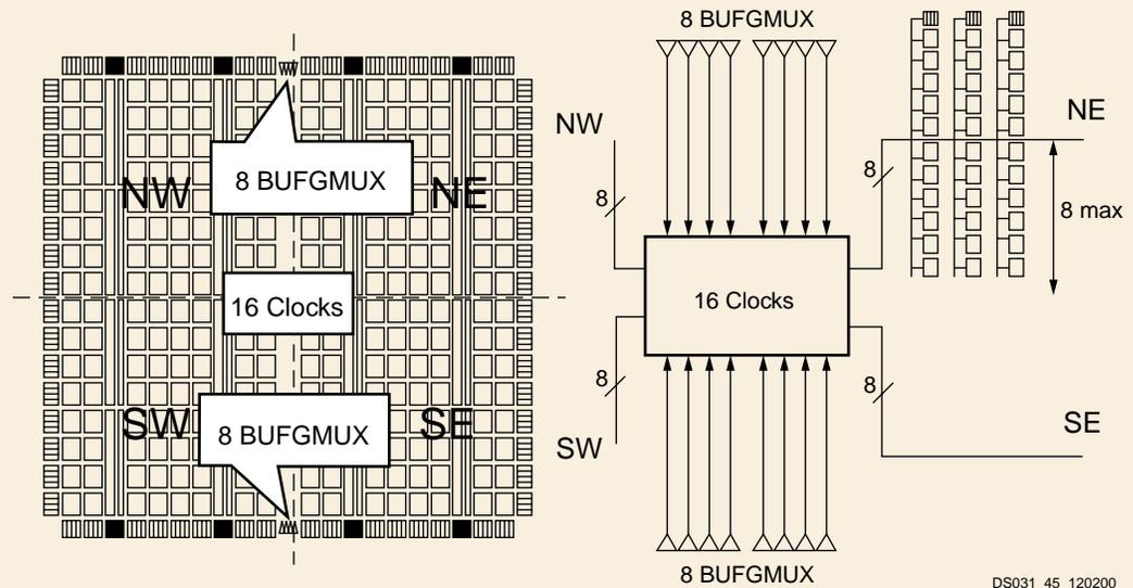
Figure 6: Virtex-II Clock Distribution
