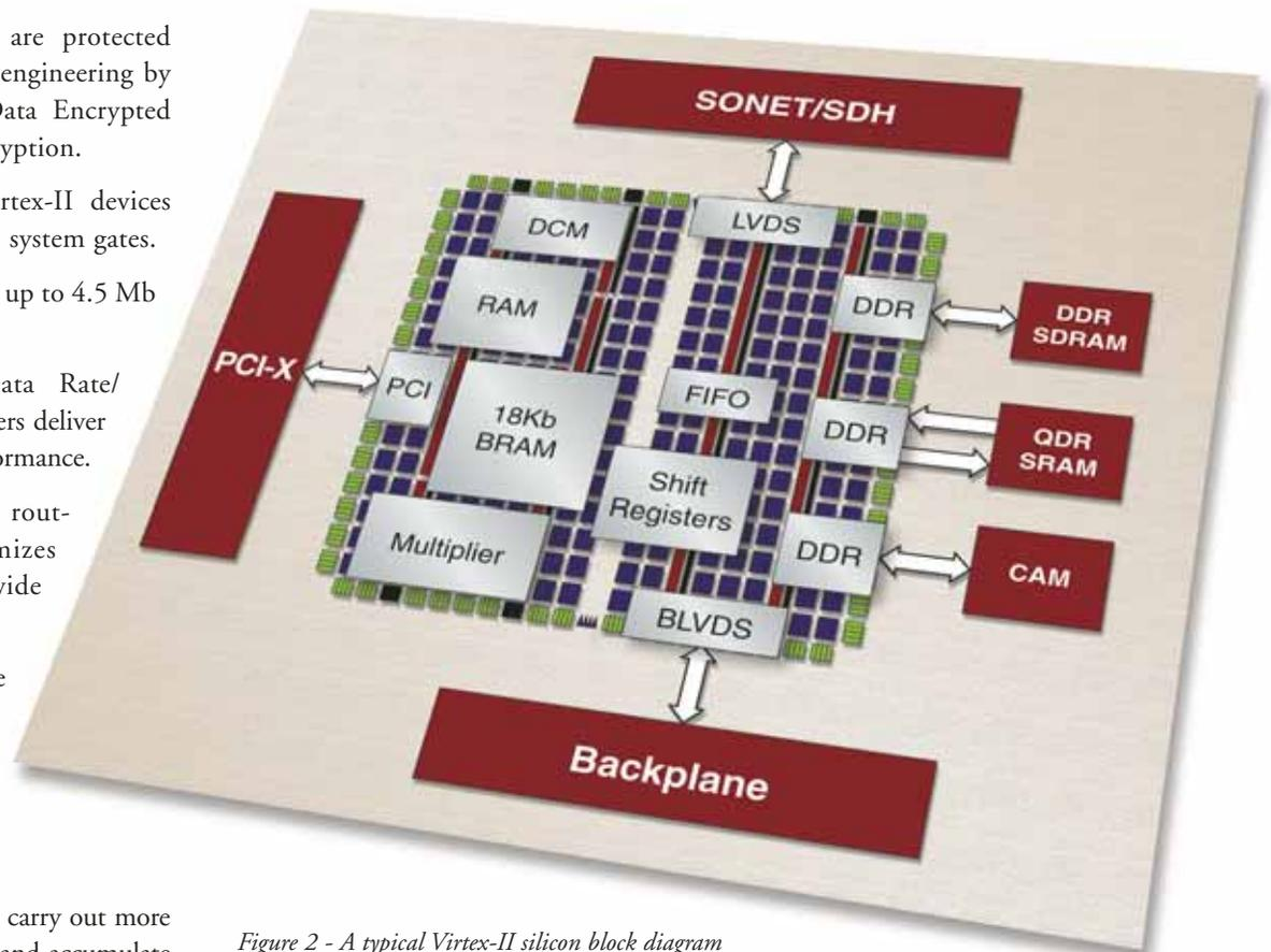
Figure 2 - A typical Virtex-II silicon block diagram
