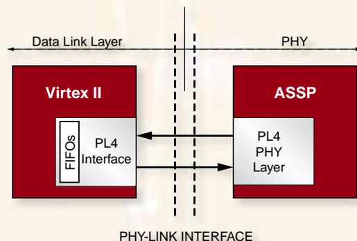
Figure 1 - OIF SPI-4 Phase 2 System Reference Model
