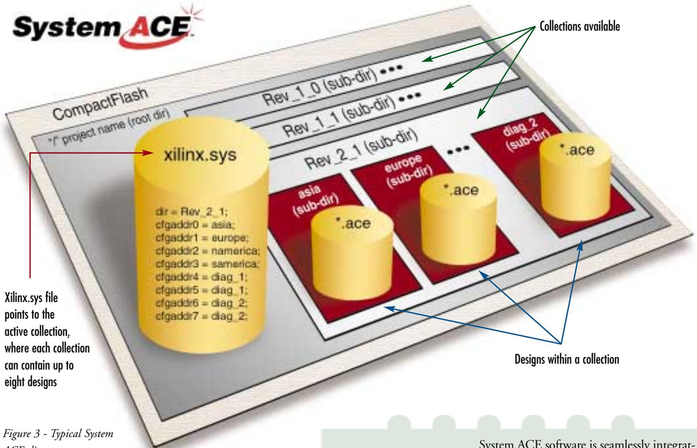
Figure 3 - Typical System ACE directory structure
