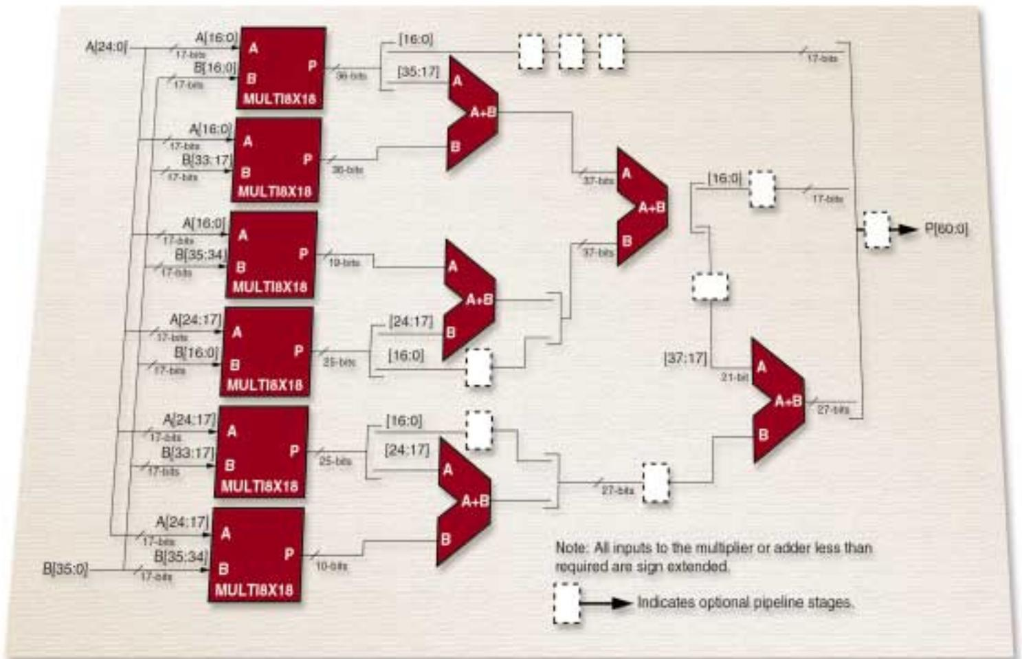
Figure 3 - Implementation produced by the Multiply Generator LogiCORE
