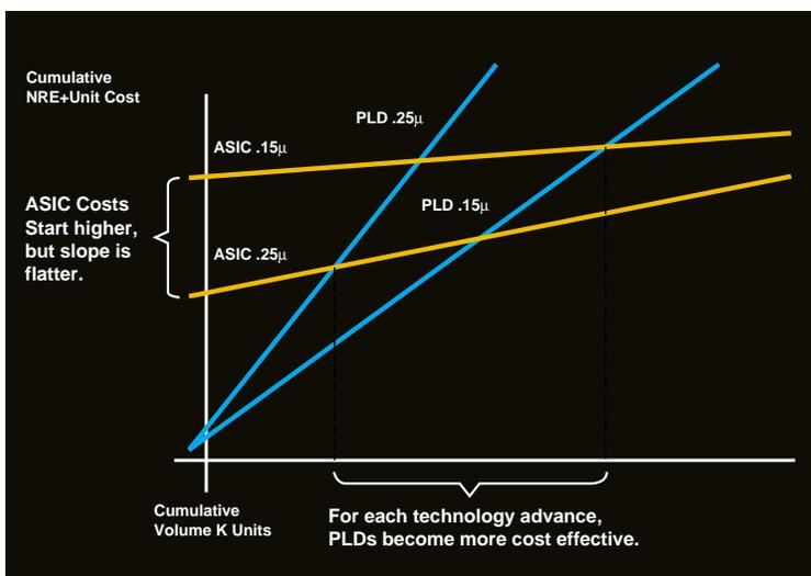
Figure 3. FPGA to ASIC crossover improves with process
