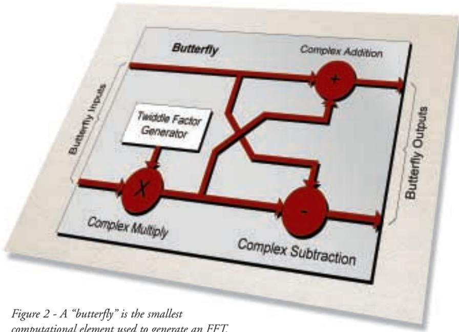
Figure 2 - A “butterfly” is the smallest computational element used to generate an FFT.
