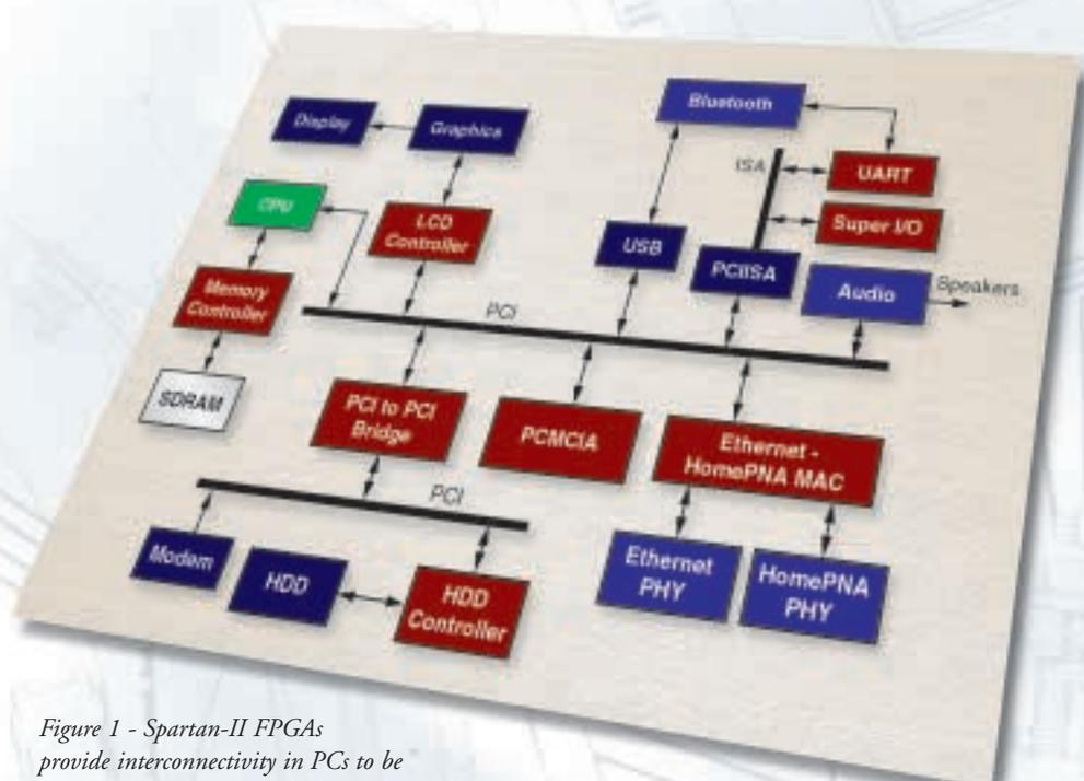
Figure 1 - Spartan-II FPGAs provide interconnectivity in PCs to be HomePNA, Ethernet, and Bluetooth-enabled.
