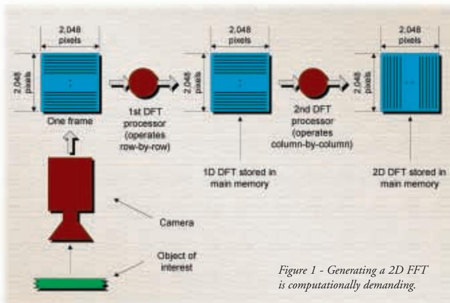
Figure 1 - Generating a 2D FFT is computationally demanding.
