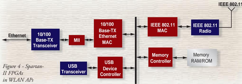
Figure 4 - Spartan-II FPGAs in WLAN APs
