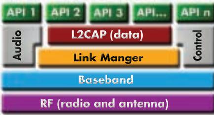
Figure 2 - Bluetooth architecture protocol stack
