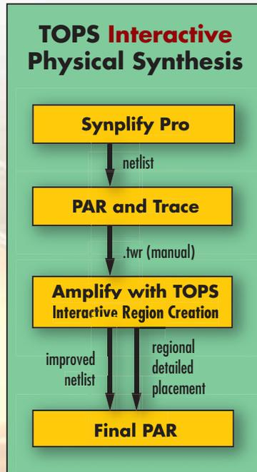
Figure 2 - Interactive physical synthesis methodology with TOPS
