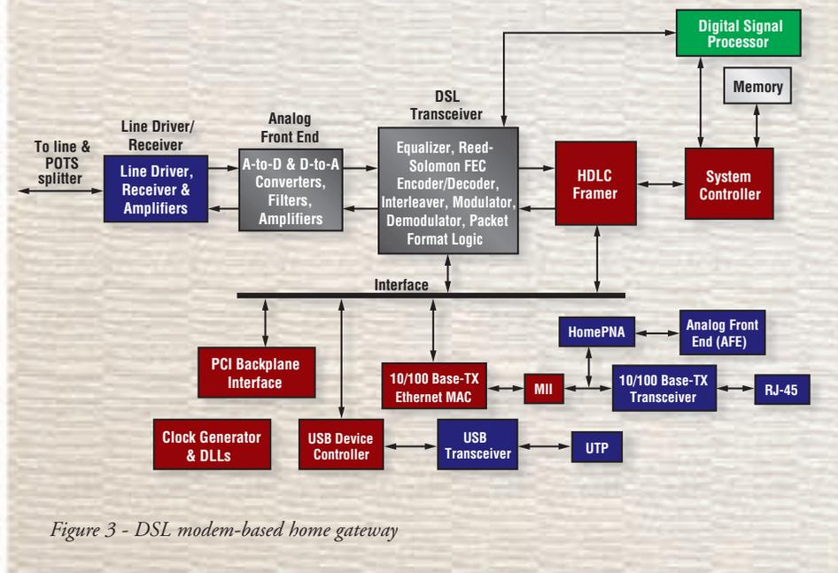
Figure 3 - DSL modem-based home gateway
