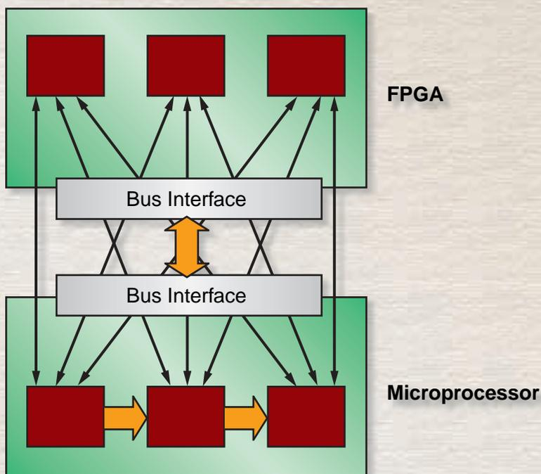
Figure 3 - FPGA-to-microprocessor without MPA support is too complicated.
