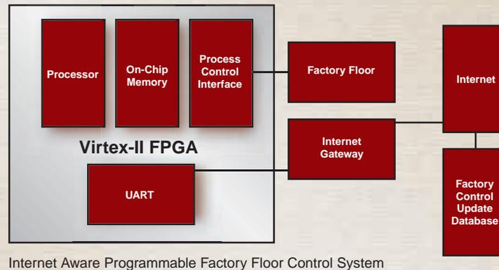
Figure 1 - Application block diagram
