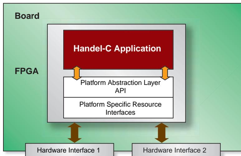
Figure 2 - Platform Specific Resource Interfaces reduce porting times.
