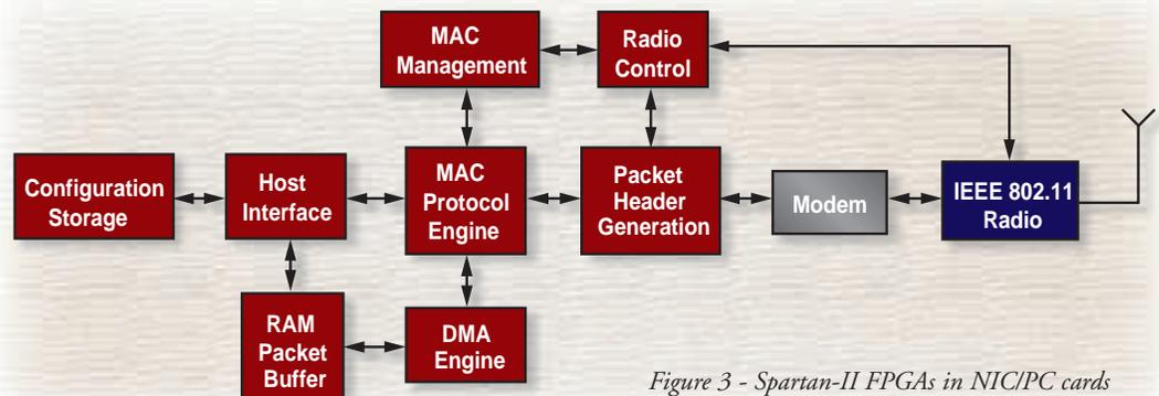
Figure 3 - Spartan-II FPGAs in NIC/PC cards
