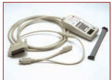
Parallel Cable IV with ribbon cable connector
