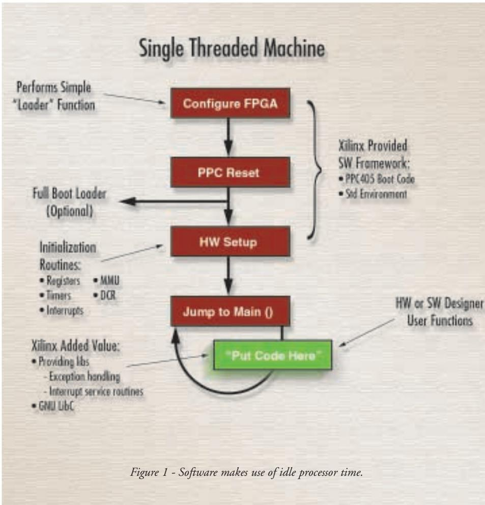
Figure 1 - Software makes use of idle processor time.
