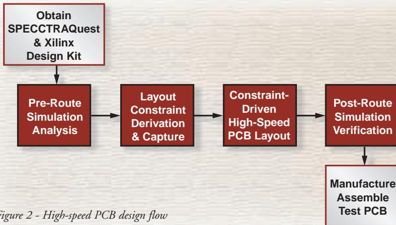
Figure 2 - High-speed PCB design flow
