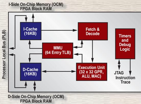
Figure 4 - Inside the PowerPC 405 processor
