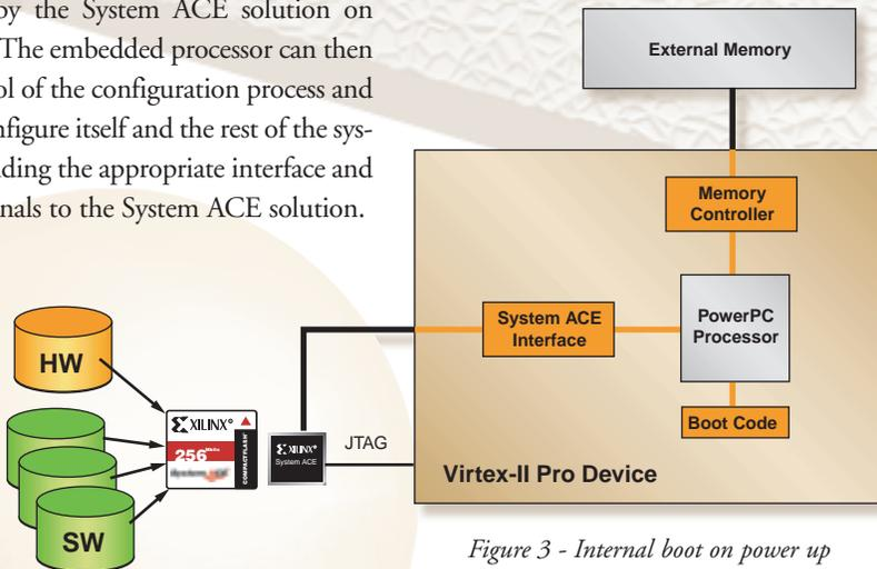
Figure 3 - Internal boot on power up
