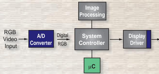
Figure 1 - Generic projection display system design
