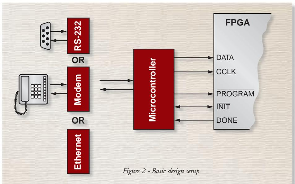
Figure 2 - Basic design setup
