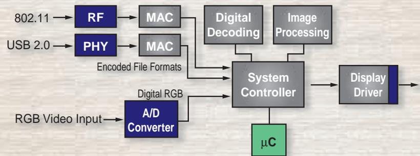
Figure 2 - Digital convergence projection display system design
