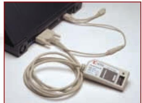
Parallel Cable IV connected to PC
