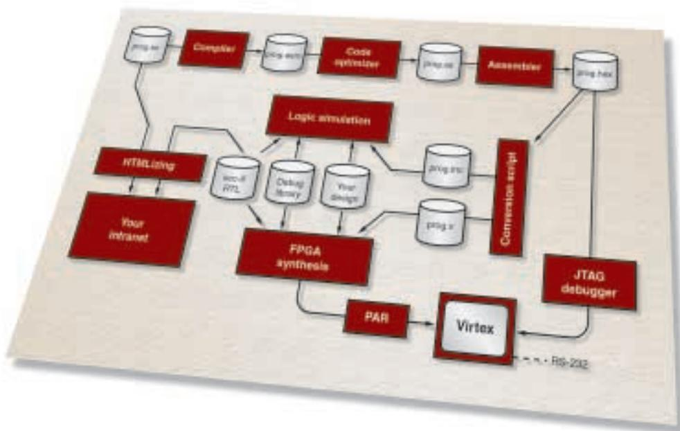
Figure 5 - The *scc-II* program development flow
