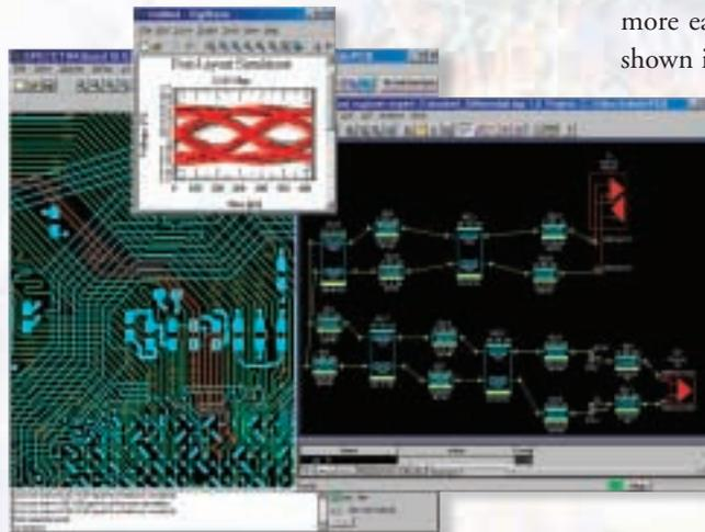
Figure 3 - Simulation from layout and extracting a differential net
