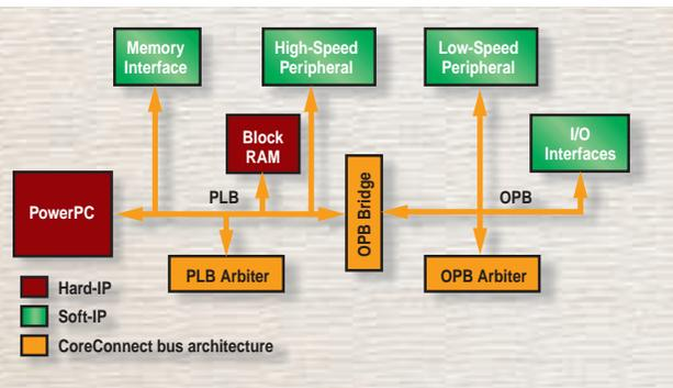
Figure 5 - Hard and soft IP cores
