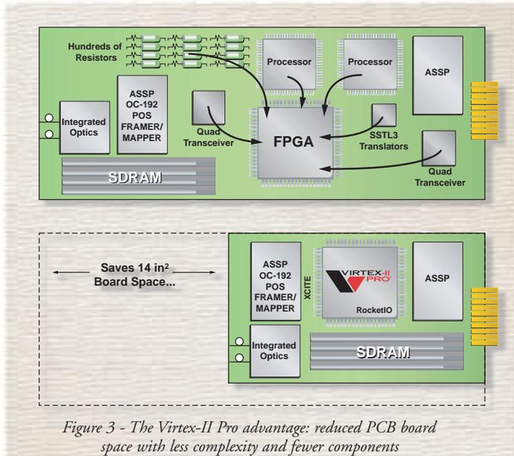
Figure 3 - The Virtex-II Pro advantage: reduced PCB board space with less complexity and fewer components
