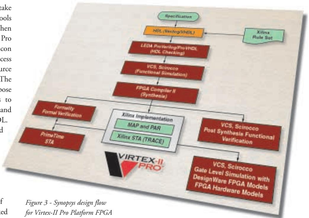
Figure 3 - Synopsys design flow for Virtex-II Pro Platform FPGA
