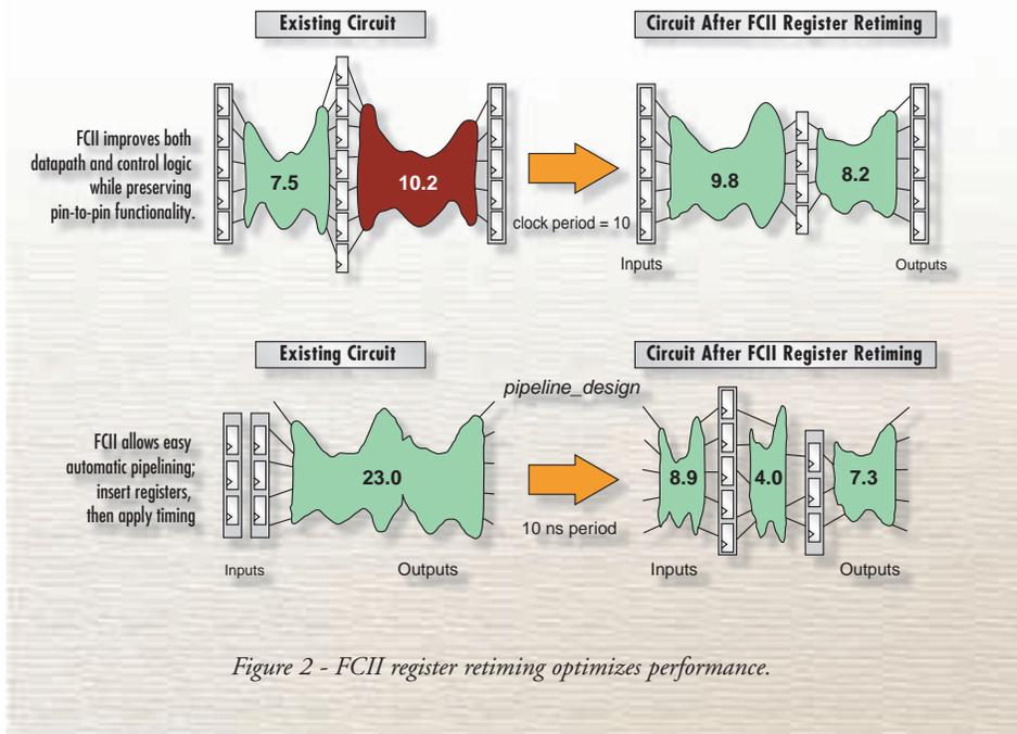
Figure 2 - FCII register retiming optimizes performance.
