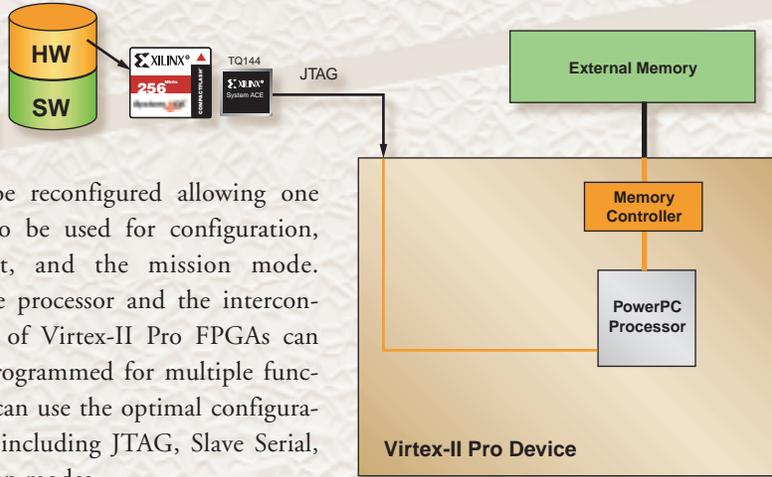
Figure 2 - Configuration via JTAG port
