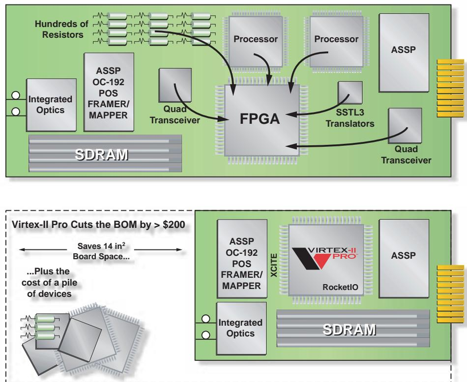
Figure 1 - Leading edge price/performance through integration and reduction of board size
