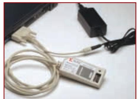
Parallel Cable IV connected to external power supply
