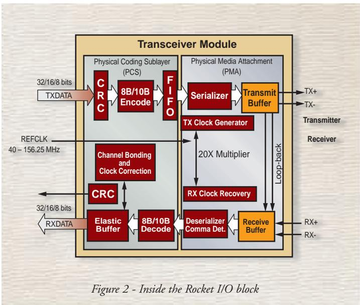
Figure 2 - Inside the Rocket I/O block
