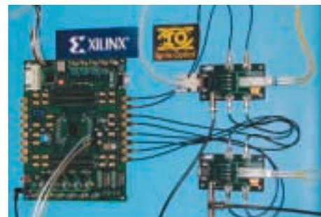
*Figure 1 - Four RocketIO channels at 2.488 Gbps with Ignis Optics' four IGP-2000 OC-48 SFP optical transceivers*
