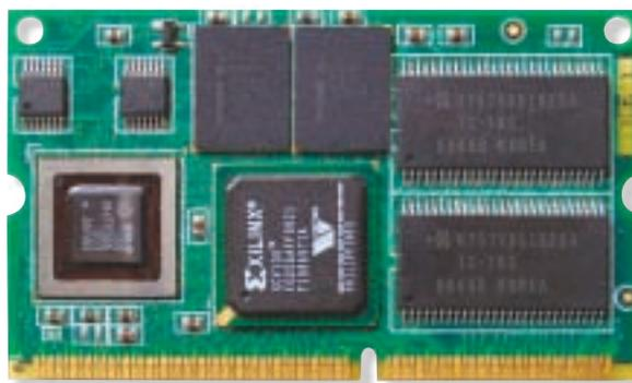
Figure 3 - Hitachi SH3  $\mu$ Engine with Virtex XCV100
