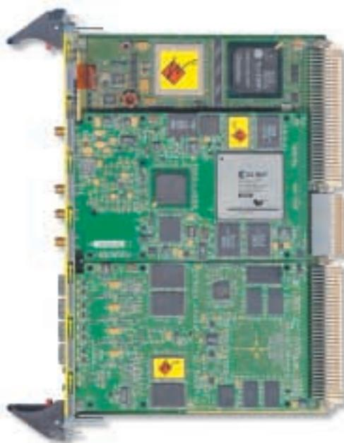
Figure 3 - WILDSTAR II for VME with I/O cards ready to insert in chassis
