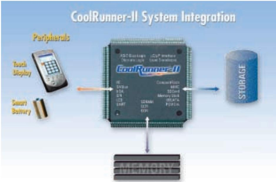
Figure 2 - Multiple functions in a single CPLD
